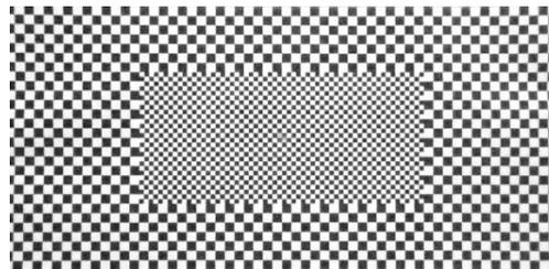
*Figura 57: Distorsion chart corretta dalle distorsioni.*
