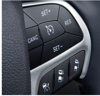
Figure 2.23: ACC controller on the steering wheel
