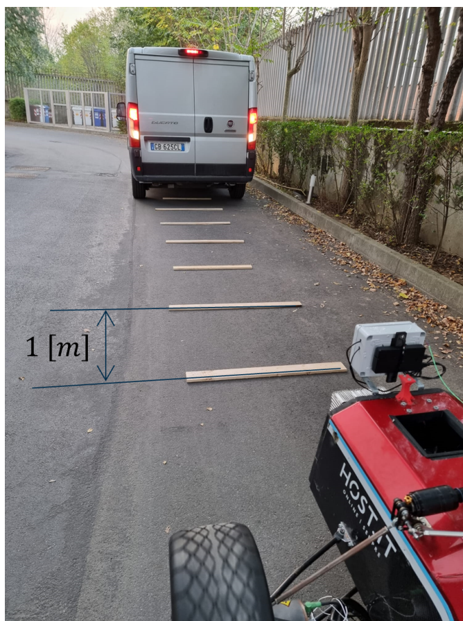
Figure 6.2: Validation of radar output information in terms of relative distance
