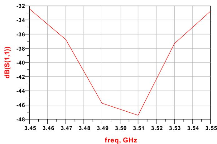
Figure 3.29: Fundamental matching condition illustrated by  $S_{11}$ .
