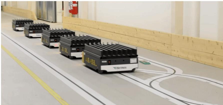
**Figure 1.2:** AGVs following tracks on the floor [6]
