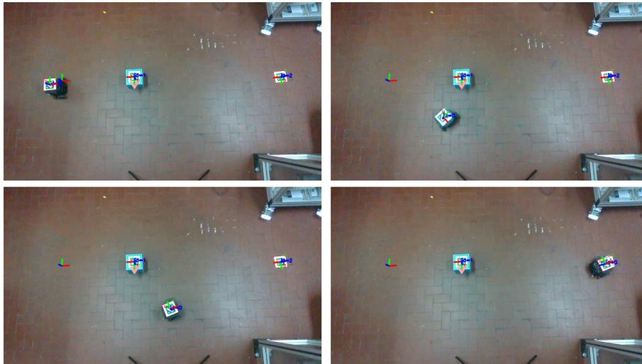
(b) ArUco detection from camera point of view
