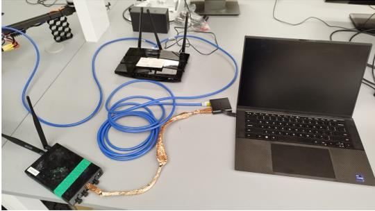
(a) Setup of laptop connected to the USRP, and to a router via Ethernet cable.
