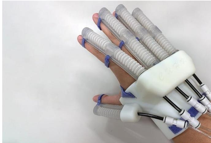
*Figure 3 Example of soft robot for rehabilitation*
