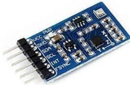
Figure 13 IMU sensor
