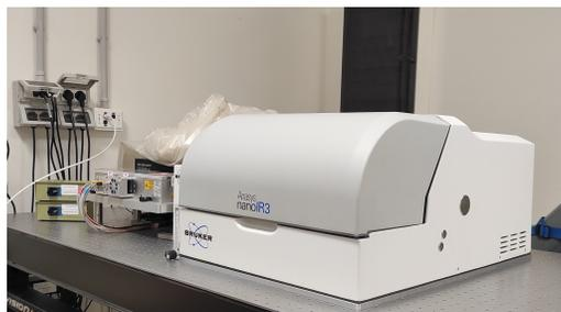
Figure 6.2.3: Anasys nanoIR3-s atomic force microscope.
