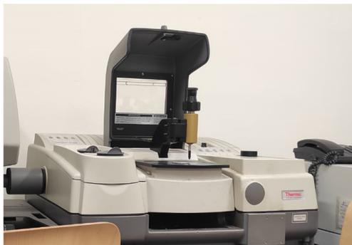
Figure 6.1.6: Nicolet 5700 spectrometer used to measure FT-IR spectra
