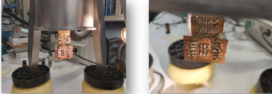
Figure 3.10: Sample holder mounted inside the cryocooler before the closure of the cryochamber. Contacts are connected to the sample, in order to perform measurements during the cooling and heating phases.
