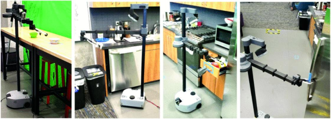
**Figure 1.3:** Robot prototype developed for [4] composed by a mobile base and a manipulator.
