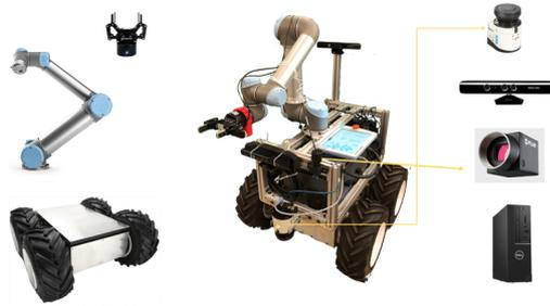
**Figure 1.2:** Prototype of a mobile robot [2], the mobile base is constituted by differential wheels while on top we have an anthropomorphic manipulator.
