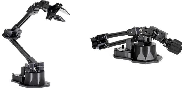
**Figure 4.4:** WidowX 250 Robot Arm used for manipulation
