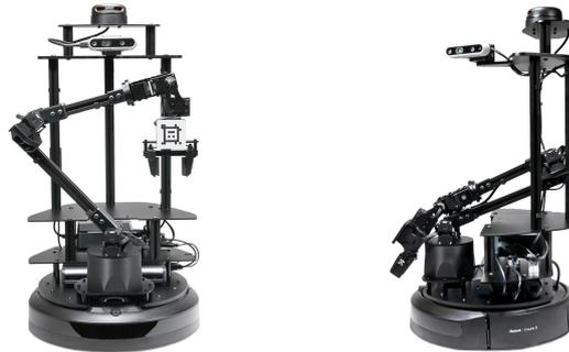
**Figure 4.1:** Mobile manipulator Locobot WX250-6DOF. Front view (left), lateral view (right)
