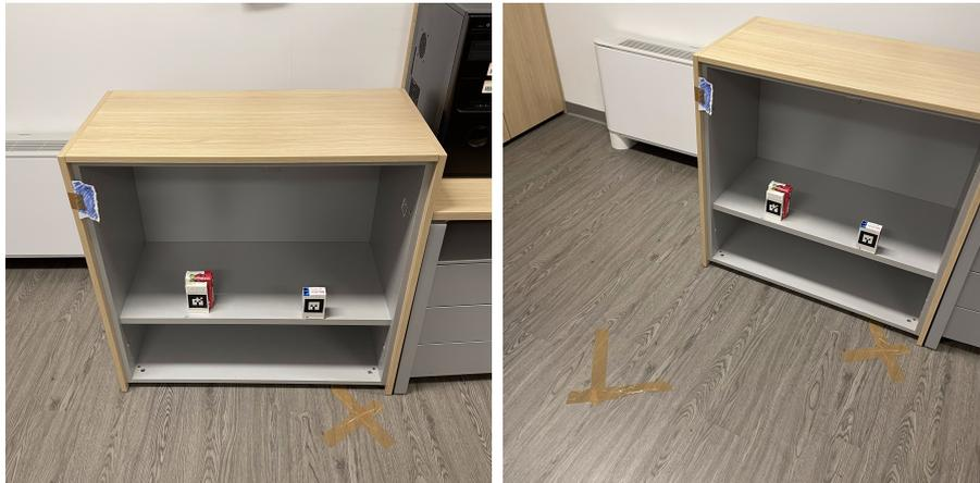
**Figure 8.9:** In these figures, we can have a look at possible positions assumed by the shelf for validating the algorithm. These positions are marked with duct tape on the floor to assure the repeatability of the experiments.
