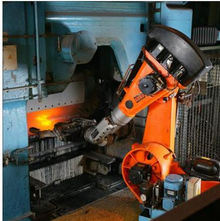
**Figure 1.1:** Example of manipulator working in a dangerous environment (foundry) for die casting in metal manufacturing [1].
