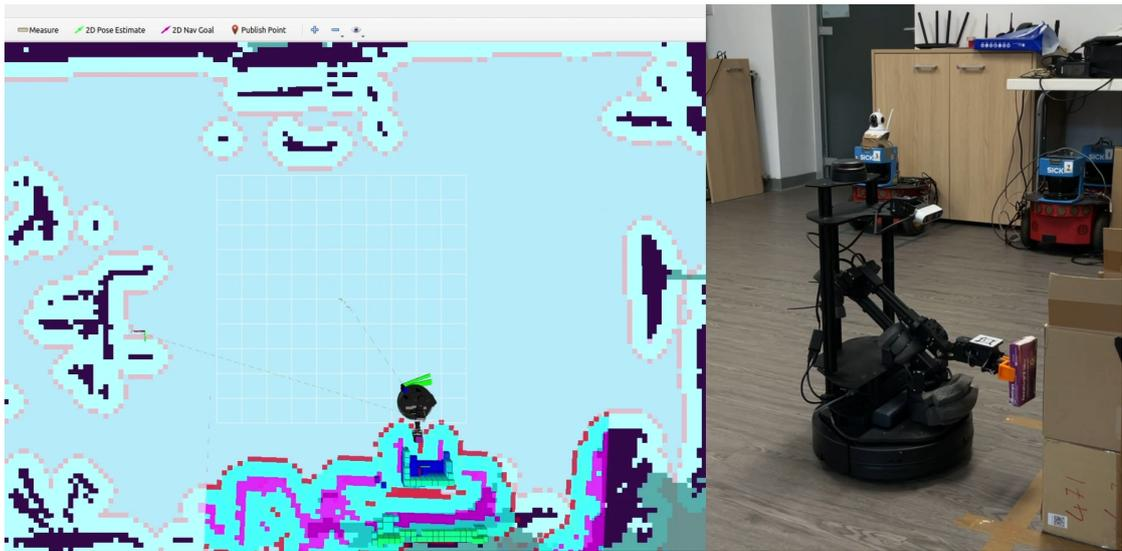
Figure 8.15: The mobile base reaches the **place pose**, now the arm should start running
