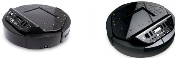
**Figure 4.3:** Kobuki YMR-K01-W1, mobile platform used for navigation
