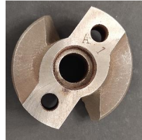
Figure 32: Flange with 2 circumferential hole and some cuts in the lateral surface
