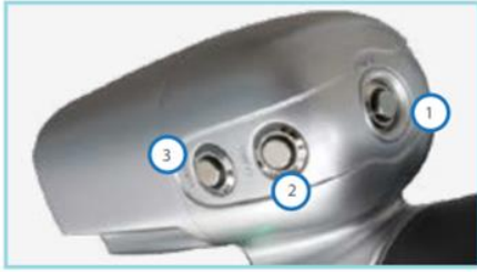
Figure 6: vision node button (1), point button (2), free button (3) [7]
