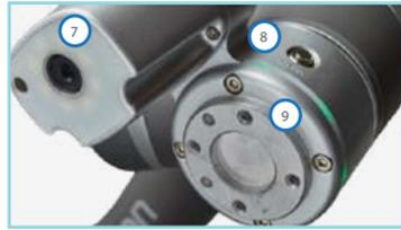
Figure 8: Vision system (7), gripper button (8), tooling flange (9) [7]
