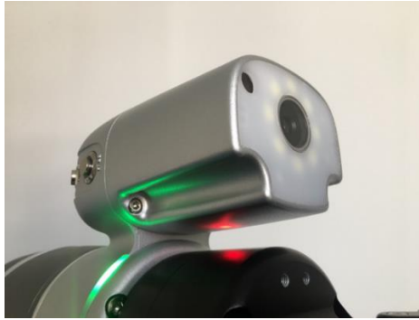
Figure 11: Camera integrated in the cobot [7]
