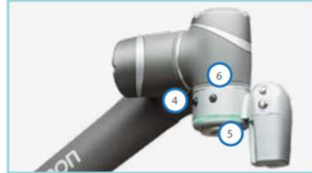
Figure 7: Analog I/O connector (4), light ring (5), Digital I/O connector (6) [7]
