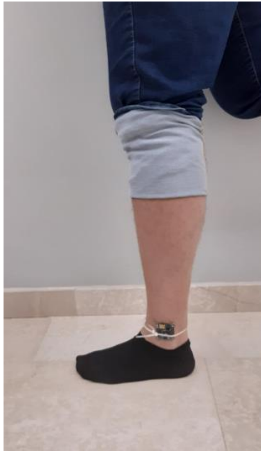
Figure 67-Position of the accelerometer for the test.
