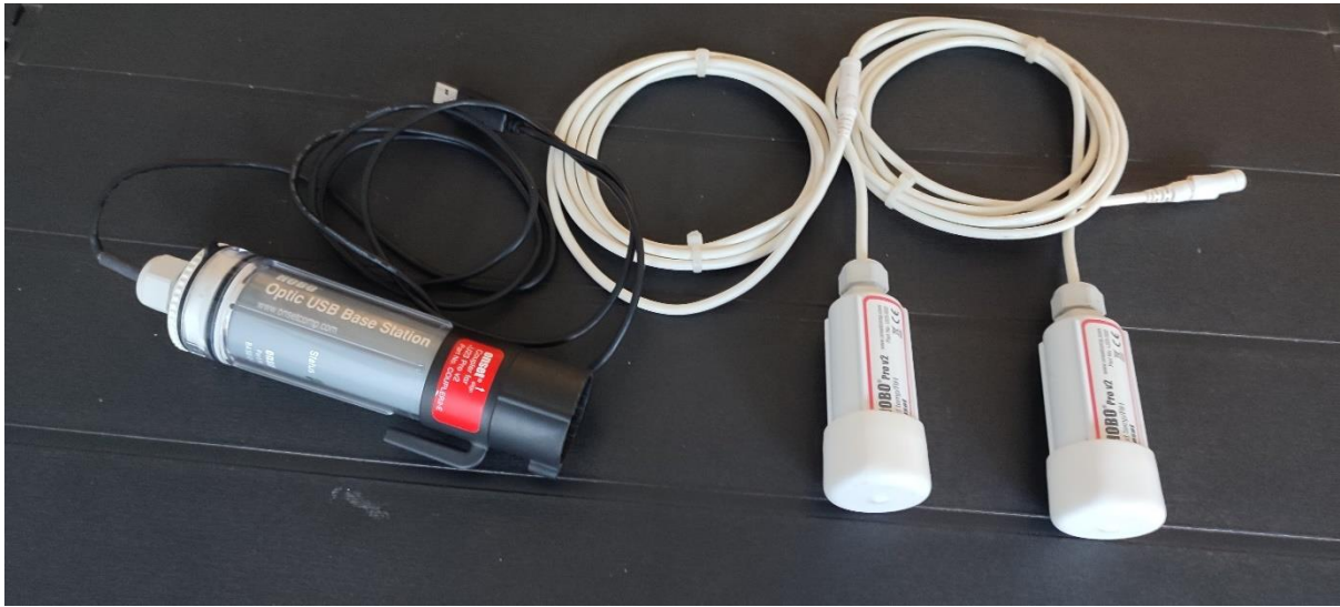
Figure 63-HOBO device for the measurment of the moisture and temperature.
