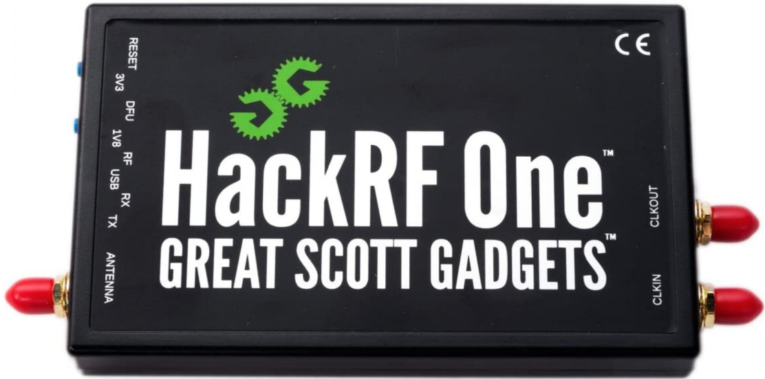
Figure A.1: HackRF One device.
