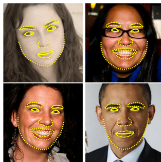
Figure 2.9: Output of Dlib’s face landmarks on the images of HELEN dataset. Figure from [37].
