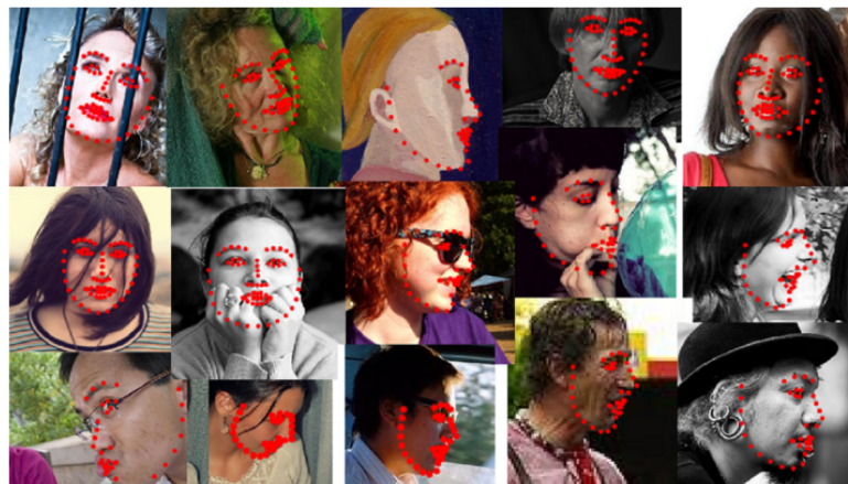
Figure 2.14: Example landmark detection from OpenFace 2.0. It is possible to notice its capability to deal with profile faces and occlusions. Figure from [39]
