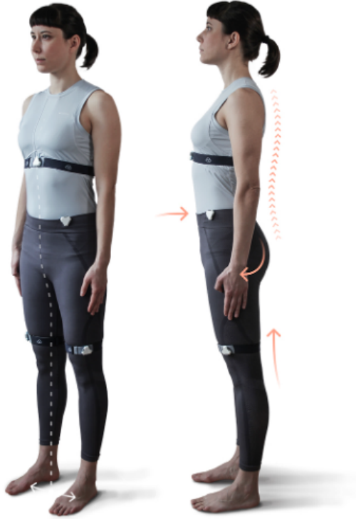
Figure 2.12: A typical full-body configuration of IMUs including IMUs positioned on the knees, waist and chest (Notch Pioneer Kit, 2021, Notch Interfaces Inc. All rights reserved).
