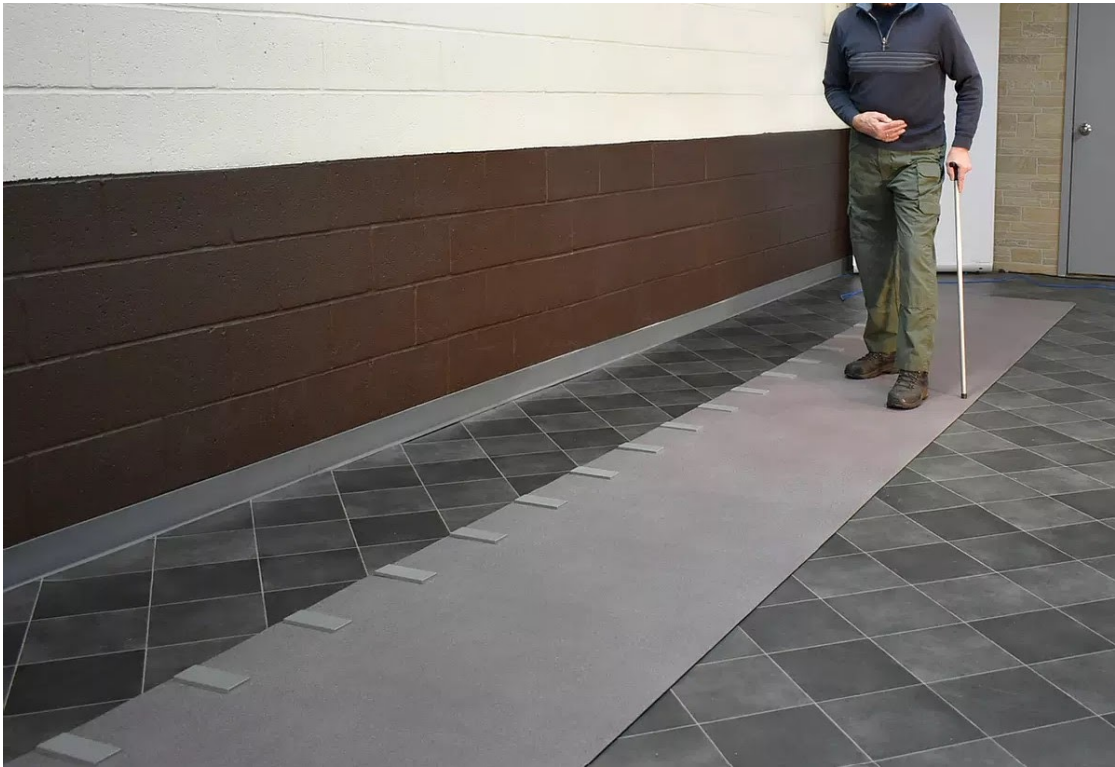
Figure 2.8: The GAITRITE system, one of the most widely used instrumented walkways [53].
