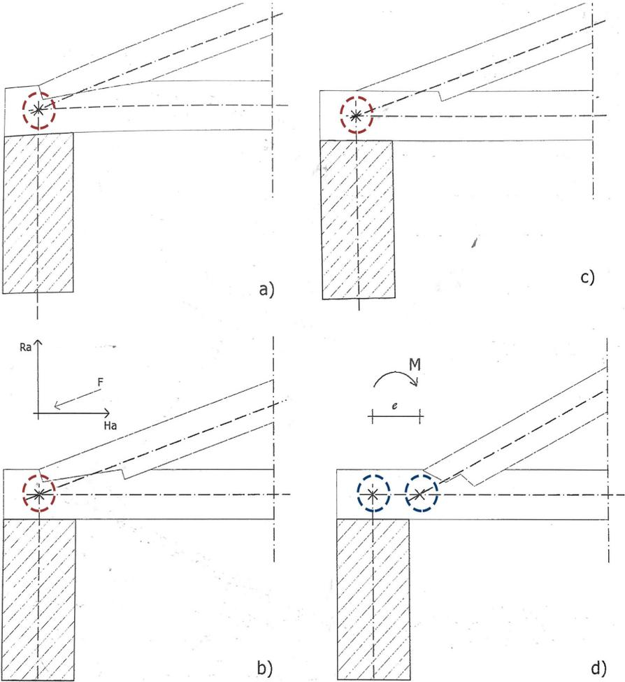
Figure 21: Connection of the axes of rafter and tie beam (Barbisan and Laner, 2000)
