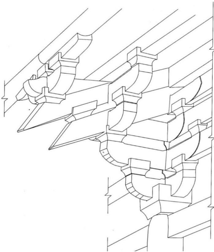
Figure 51: Four jumps Dougong on the inner columns with two Ang and two Hua gong (Pan, 2017)
