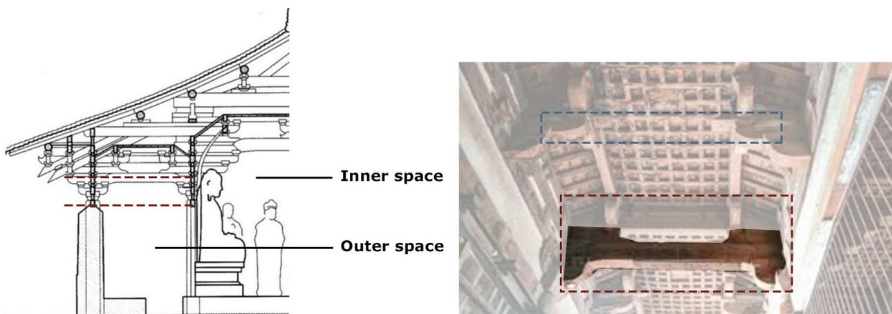
Figure 54: Continuous interface of the main hall of Foguang temple
