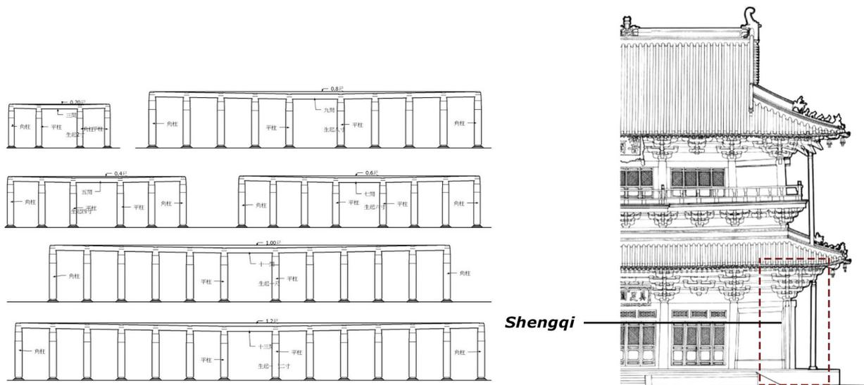
Figure 71: Left: diagram of “Shengqi” of the corner columns; Right: present of “Shengqi” in the Guanyin pavilion<sup>23</sup>
