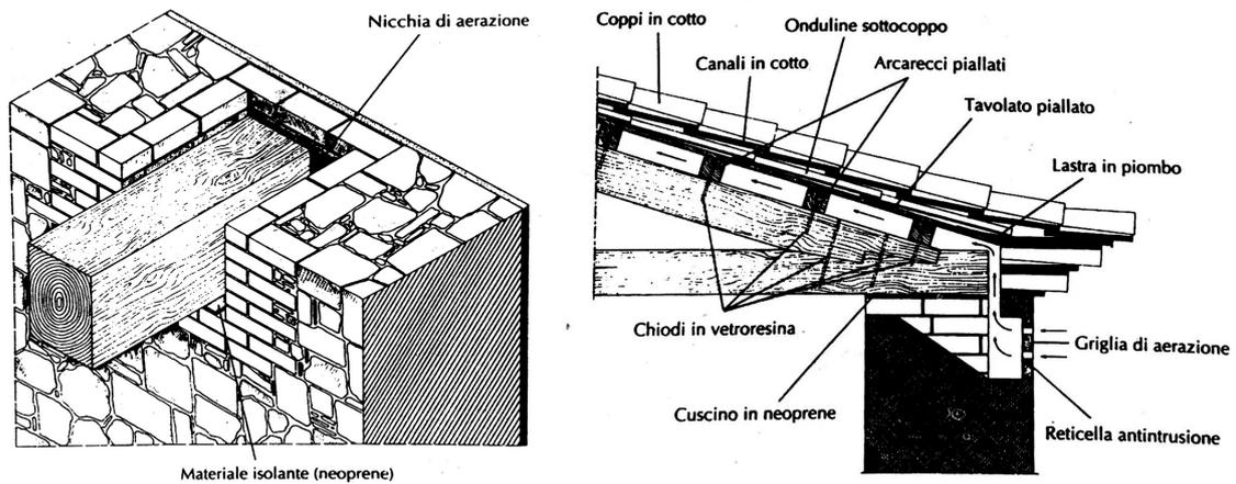
Figure 25: Air gap between tie beam and masonry wall. (Liotta, 1994)
