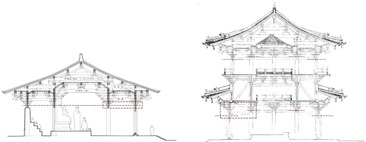
Figure 52: Comparison of the height of the outer column and inner column of the main hall of Foguang temple (left) and the Guanyin pavilion of Dule temple (right)
