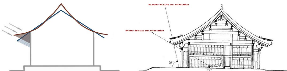
Figure 36: Left: Summer Solstice and Winter Solstice sun orientations; Right: Shadow area with different slopes of the roof
