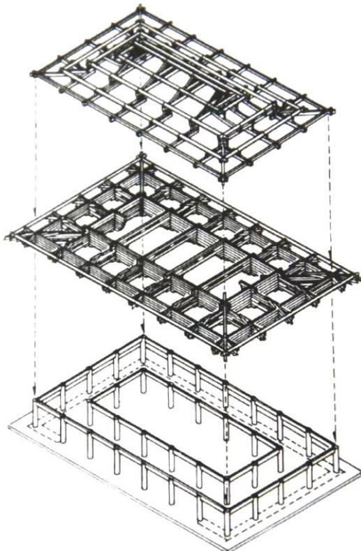
Figure 53: Axonometry diagram of a palace order architecture
