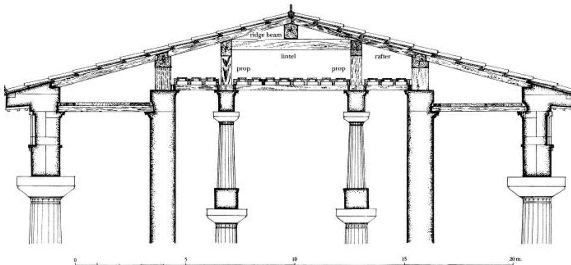
Figure 4: Post and Lintel roof (Klein, 1998)
