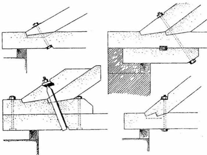
Figure 23: Examples of connection of rafter and tie beam by T. Krauth and F. Sales Meyer (Barbisan and Laner, 2000)
