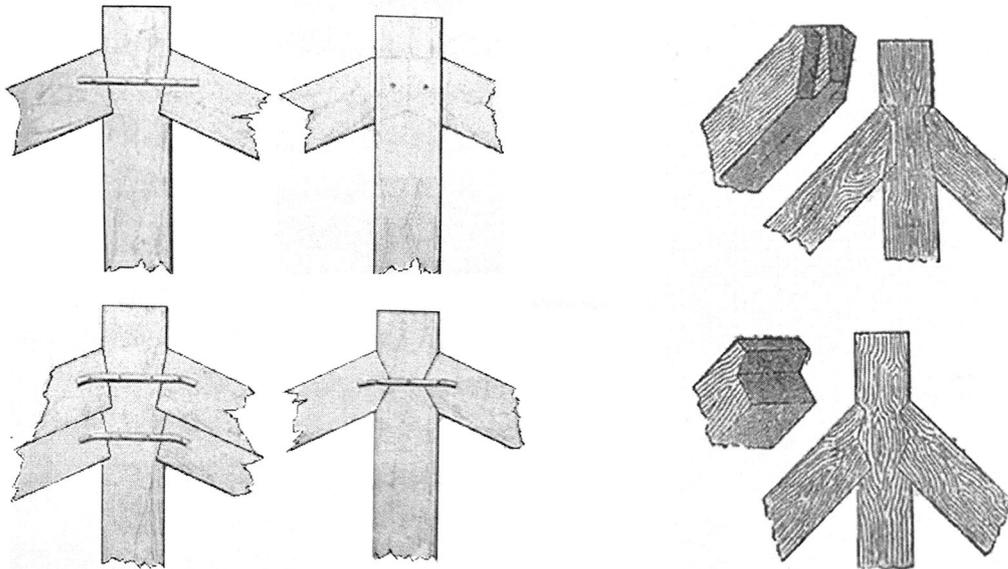
Figure 24: Left: connection with the corner of rafters remained (Aluisetti and Pizzogalli, 1827); Right: tenon and mortise connection between rafter and post (Breymann, 1985)
