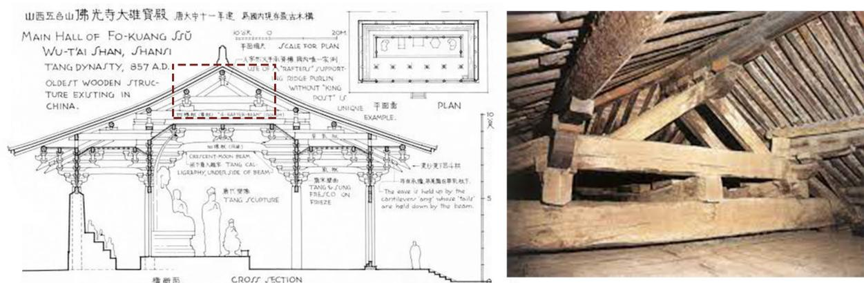
Figure 50: Section and photo of the “rafter” on the roof of the main hall of Foguang temple (Liang, 1984)
