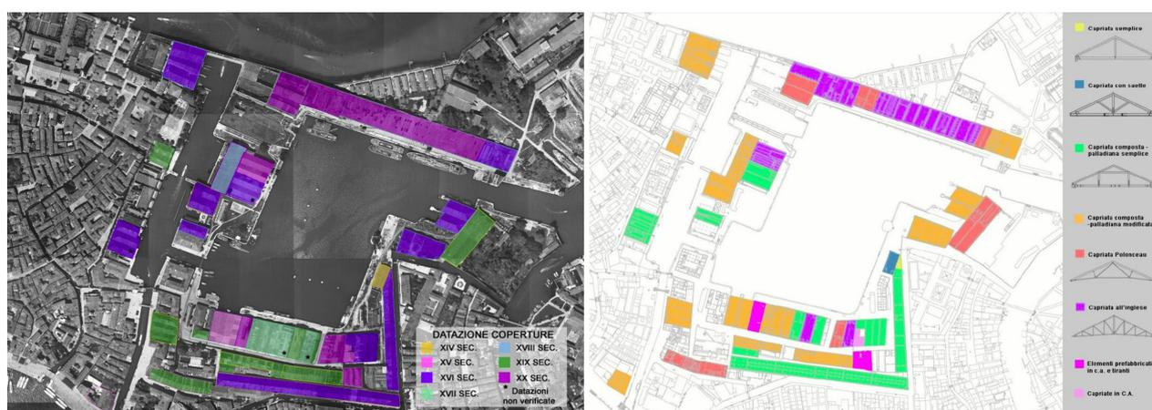
Figure 29: Roof construction times and identification of trusses by G. Bettiol (Menichelli et al, 2009) (Bertolini Cestari and Marzi, 2018)
