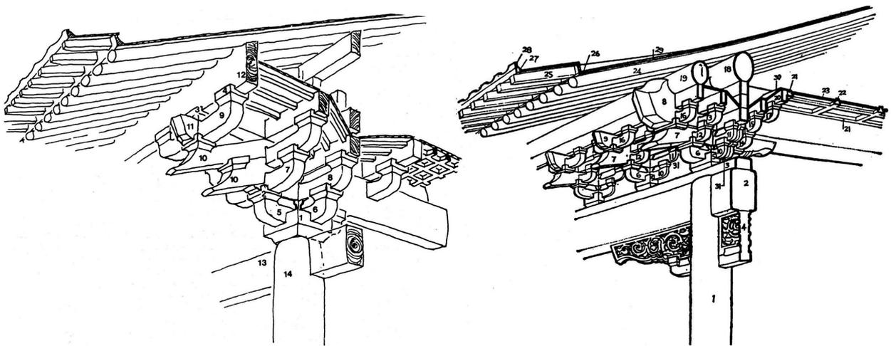
Figure 44: Comparison of Song style Dougong (left) and Qing style Dougong (right) (Liu, 1984)
