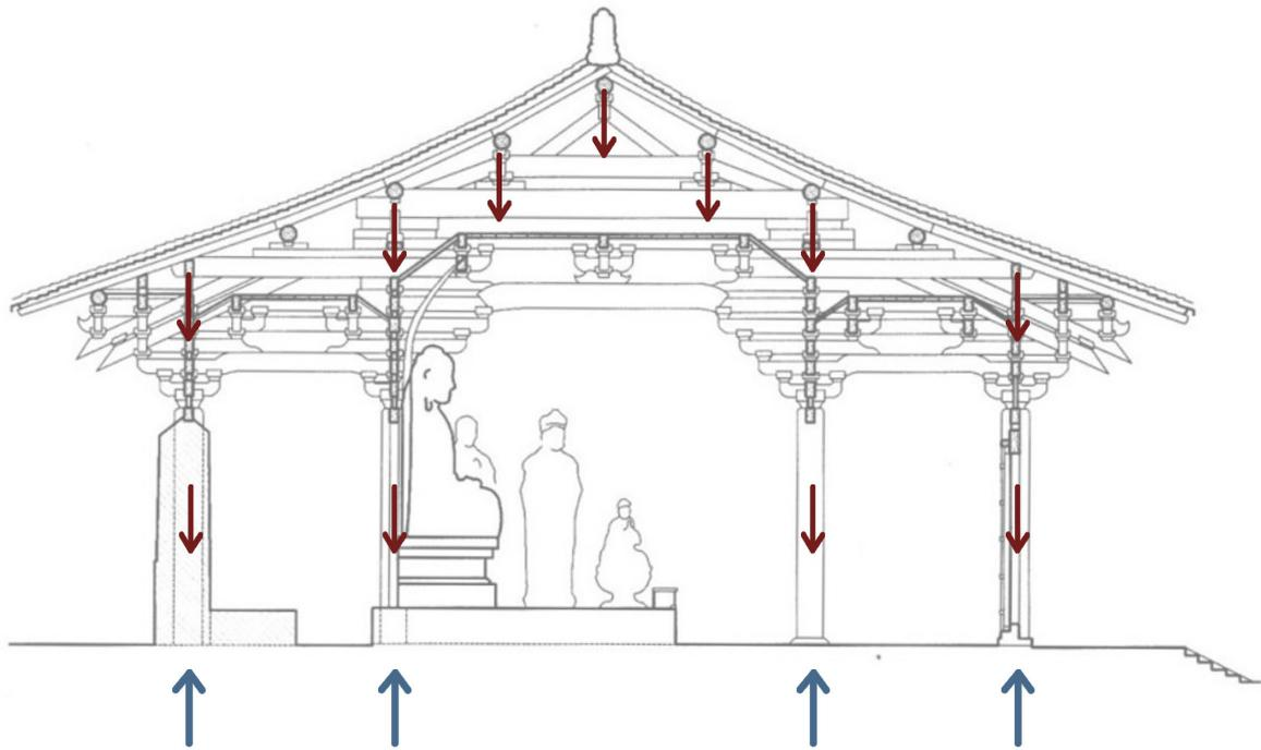
Figure 39: Transmission of forces within Chinese architecture, example of the main hall of Foguang temple
