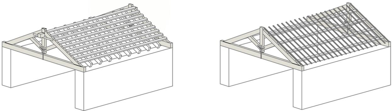
Figure 8: Left: Piedmont roof with truss structure; Right: Lombard/Roman roof with truss structure
