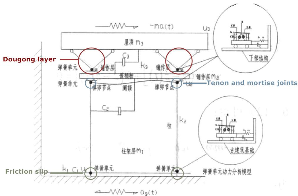
Figure 72: Dynamic analysis of ancient Chinese architecture (Gao et al, 2008)
