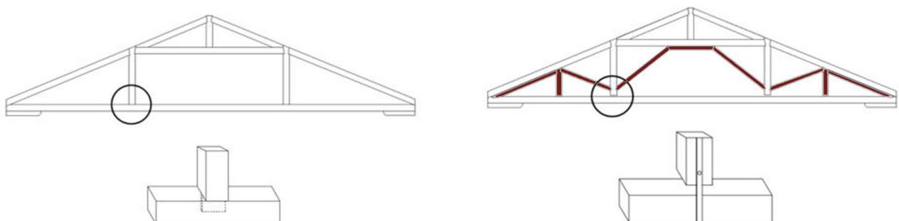
Figure 32: Left: original closed joint truss; Right: intervened open joint truss, the new elements highlighted in red (original drawing by Ferretti et al, 2022)
