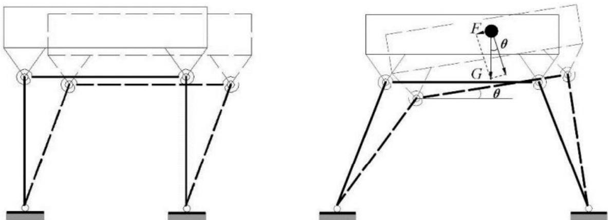
Figure 70: Left: parallel column; Right: column with "Ce Jiao"
