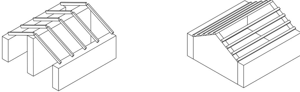
Figure 7: Left: Piedmont roof; Right: Lombard/Roman roof
