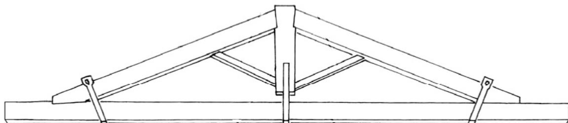
Figure 11: King post truss with braces (*Capriata semplice con saettoni*)
