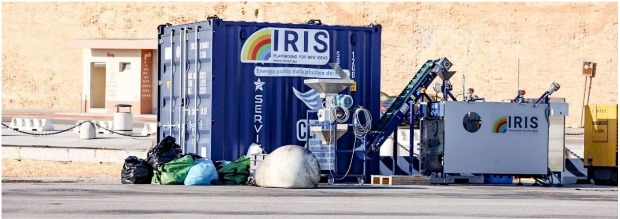
Figure 8: Green Plasma machine and waste to be pyrolyzed for energy supply
