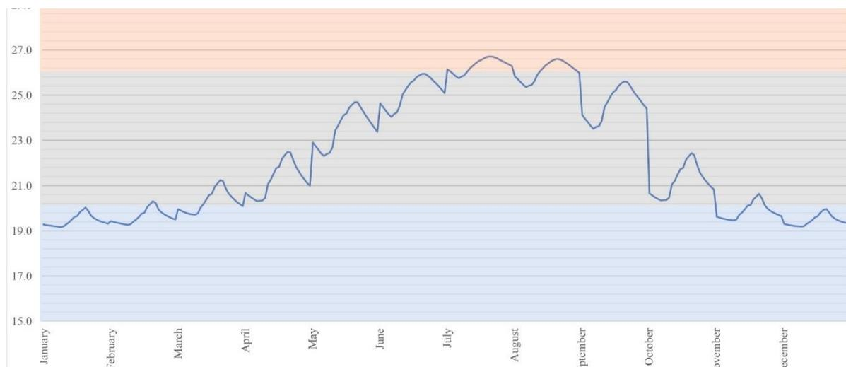
Figure 4.13 Operative temperature - with louver shades (multi-zone model)
