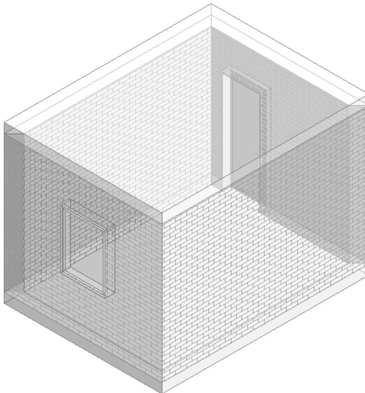
*Figure 3.7 Graphical representation of the single-zone model*
