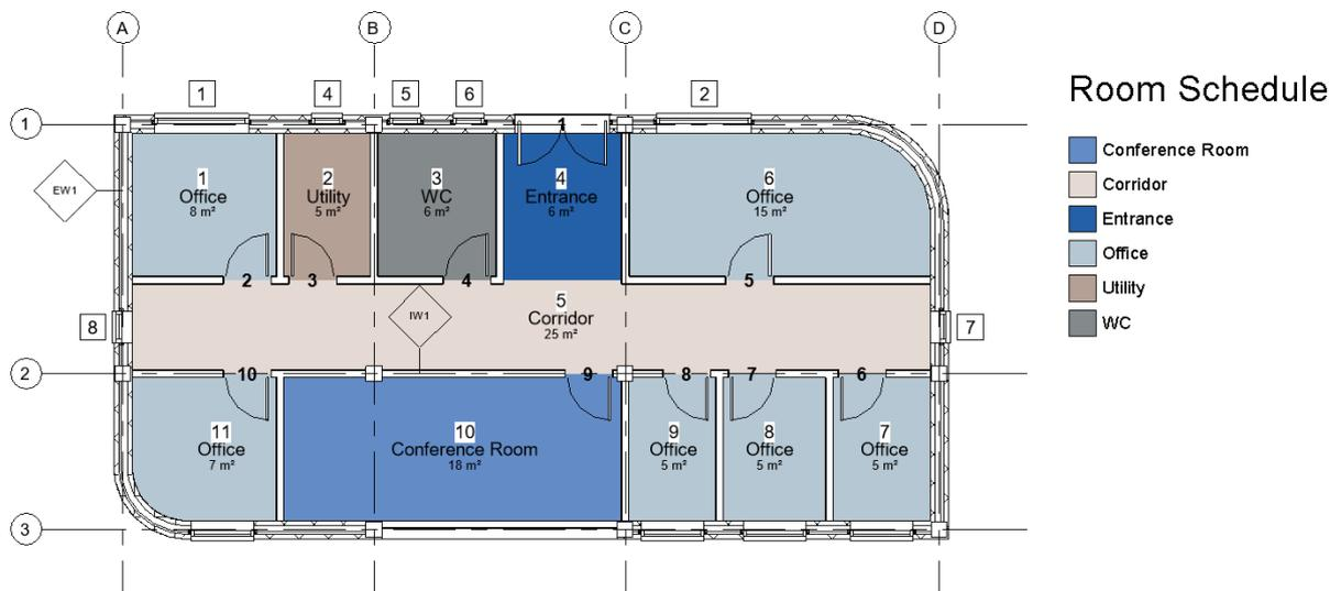
Figure 3.33 Floor plan of the multizone model with room programs
