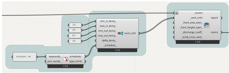
Figure 3.55 ning a window control component "HB Window Opening" to apertures
