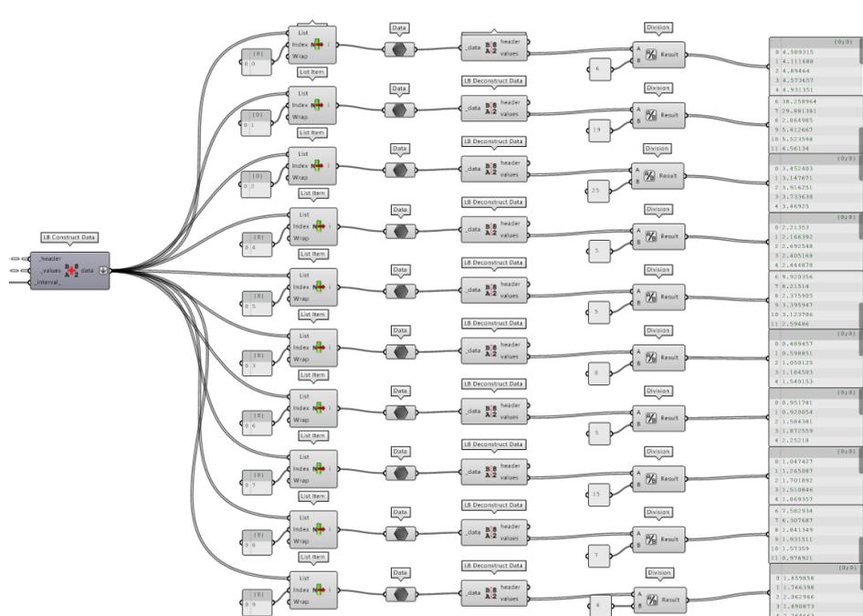
Figure 3.59 Deconstructing data to divide the primary energy use by zone area
