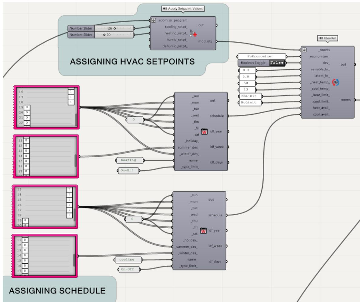
Figure 3.54 Assigning HVAC system with the component "HB Ideal Air"
