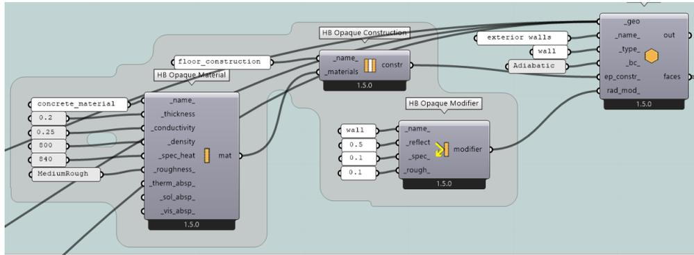
Figure 3.15 “HB Face” algorithm with construction modifier for opaque component-adiabatic walls
