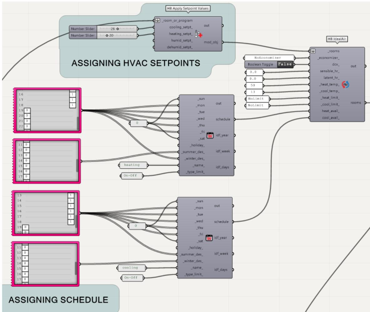
Figure 3.21 Assigning HVAC system with the component "HB Ideal Air"
