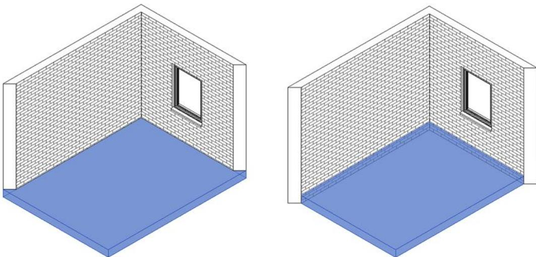
*Figure 3.6 Modified inverted floor extrusion, inside the interior wall surface borders*
