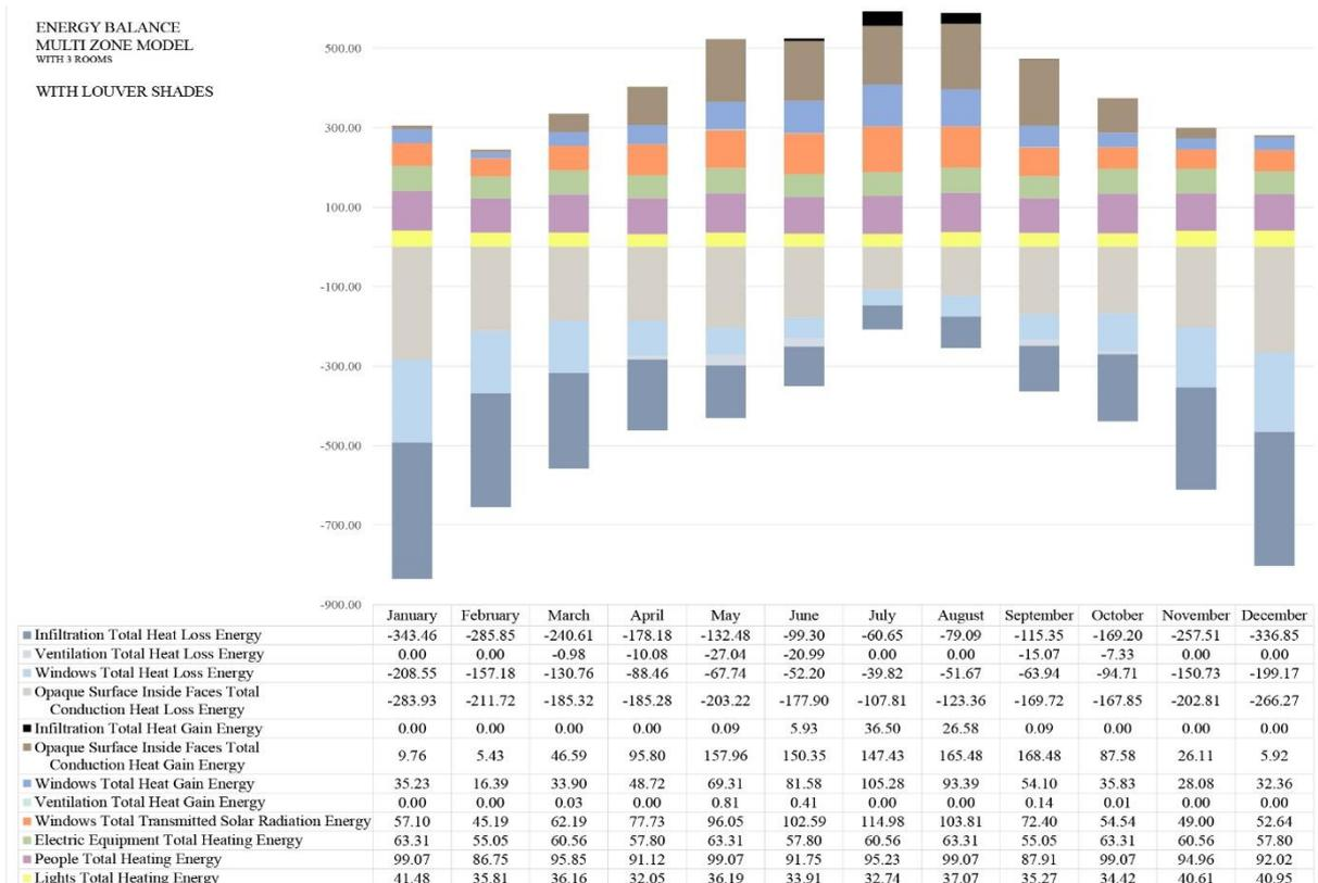
Figure 5.6 Energy balance with louver shades (three zone model)
