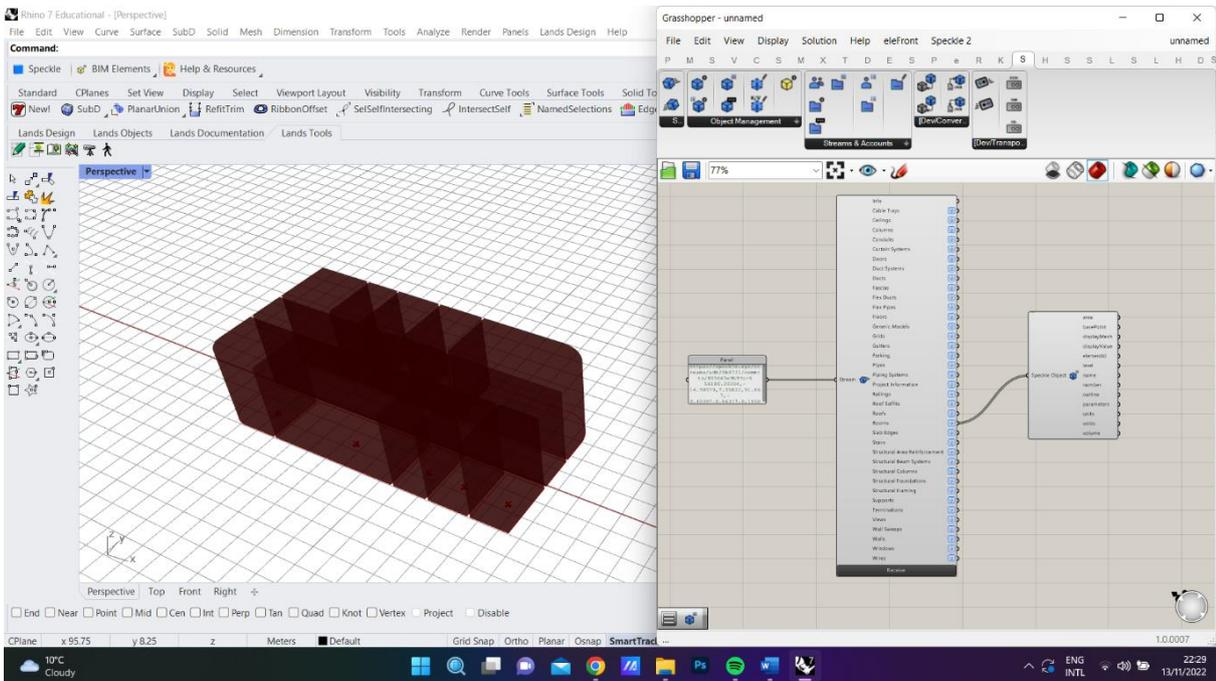
Figure 3.36 Receiving the geometry on Grasshopper using the Speckle stream
