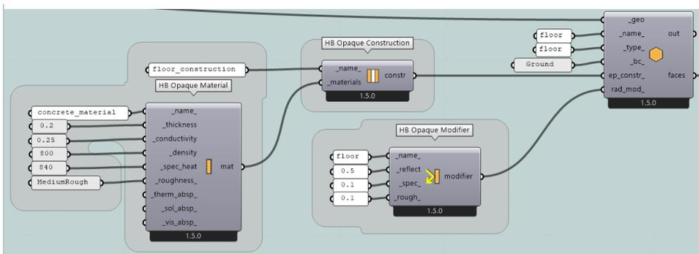
Figure 3.14 “HB Face” algorithm with construction modifier for opaque component-floor
