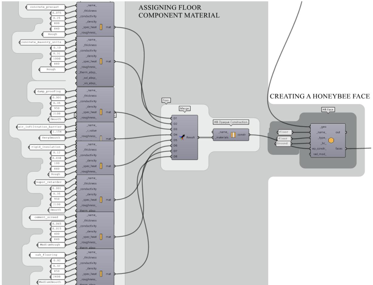
Figure 3.46 "HB Face" algorithm with construction modifier for opaque component- floor
