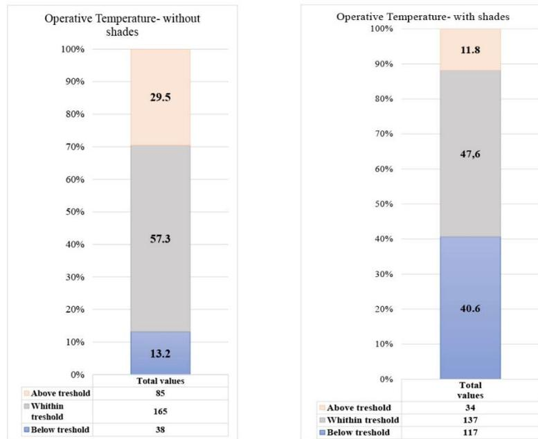
Figure 5.9 Average operative temperatures values below, in and above threshold (three zone model)
