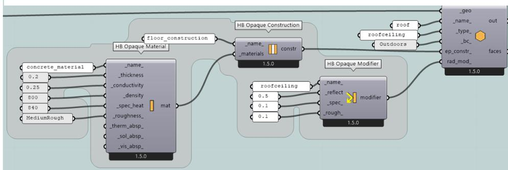
Figure 3.13 “HB Face” algorithm with construction modifier for opaque component-roof
