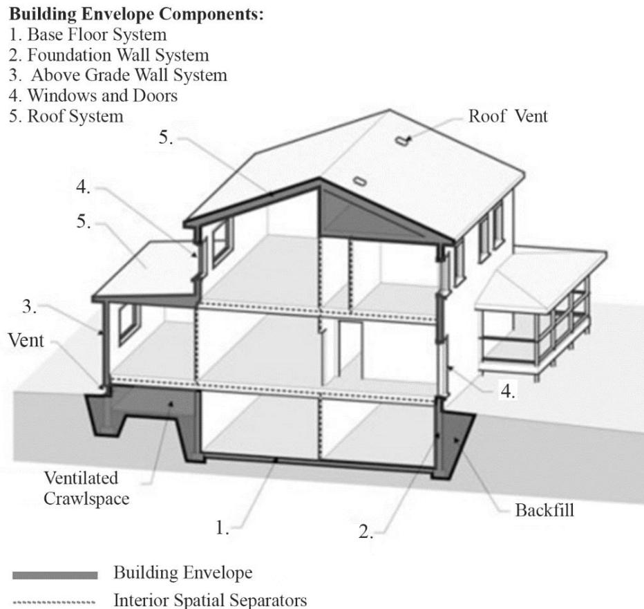
Figure 2.1 Building envelope components
