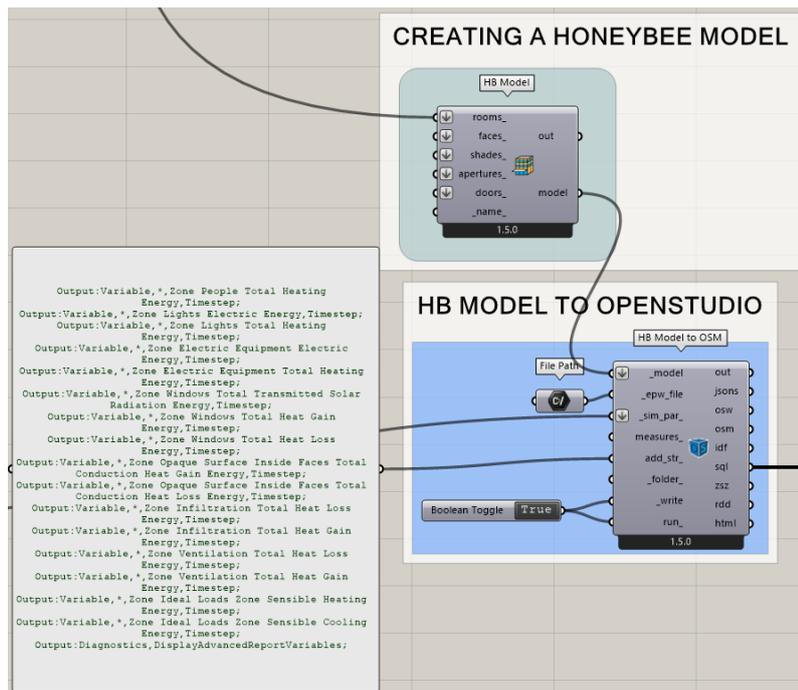
Figure 3.24 Requesting the desired outputs and running the simulations
