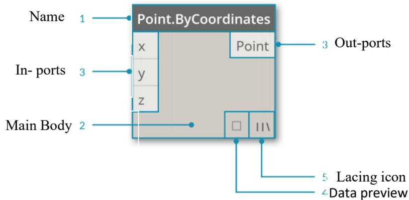
Figure 2.21 Node components on Dynamo
