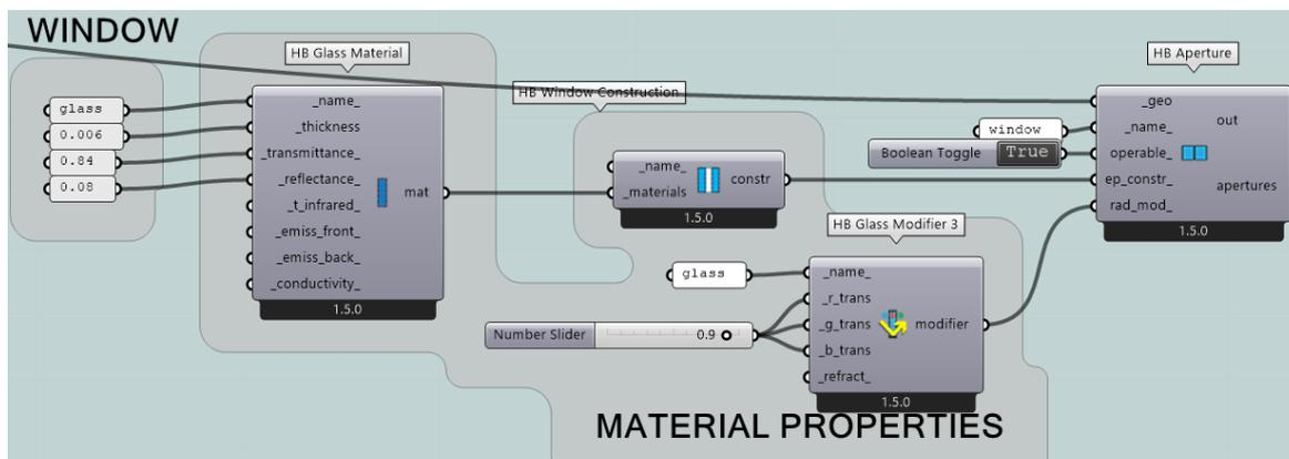
Figure 3.16 “HB Aperture” algorithm with construction modifier for transparent component
