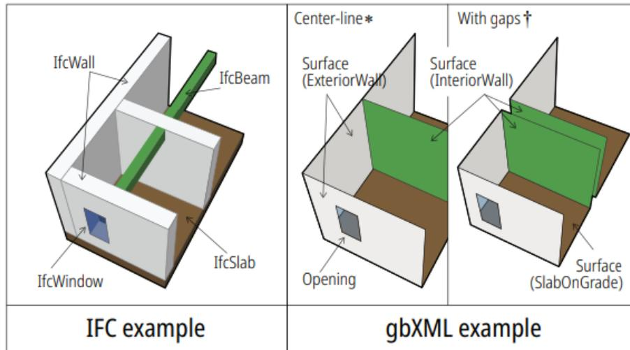
Figure 2.19 Different geometry representations by IFC and gbXML, an example. (\*) Modelled by wall centre line (without gaps). (†) Modelled by wall faces (with gaps)
