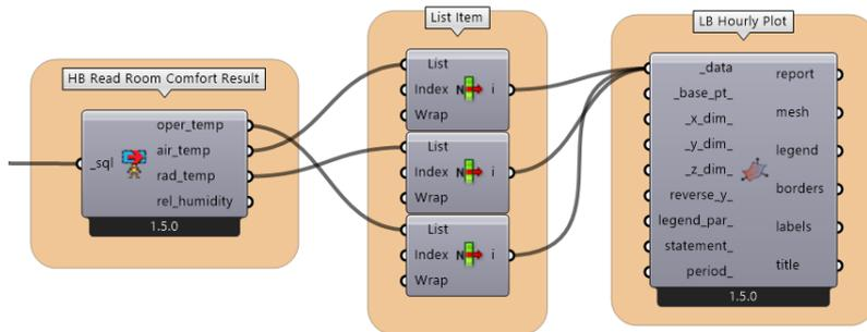
Figure 3.64 "HB Read Room Comfort Results" algorithm for thermal comfort visualization
