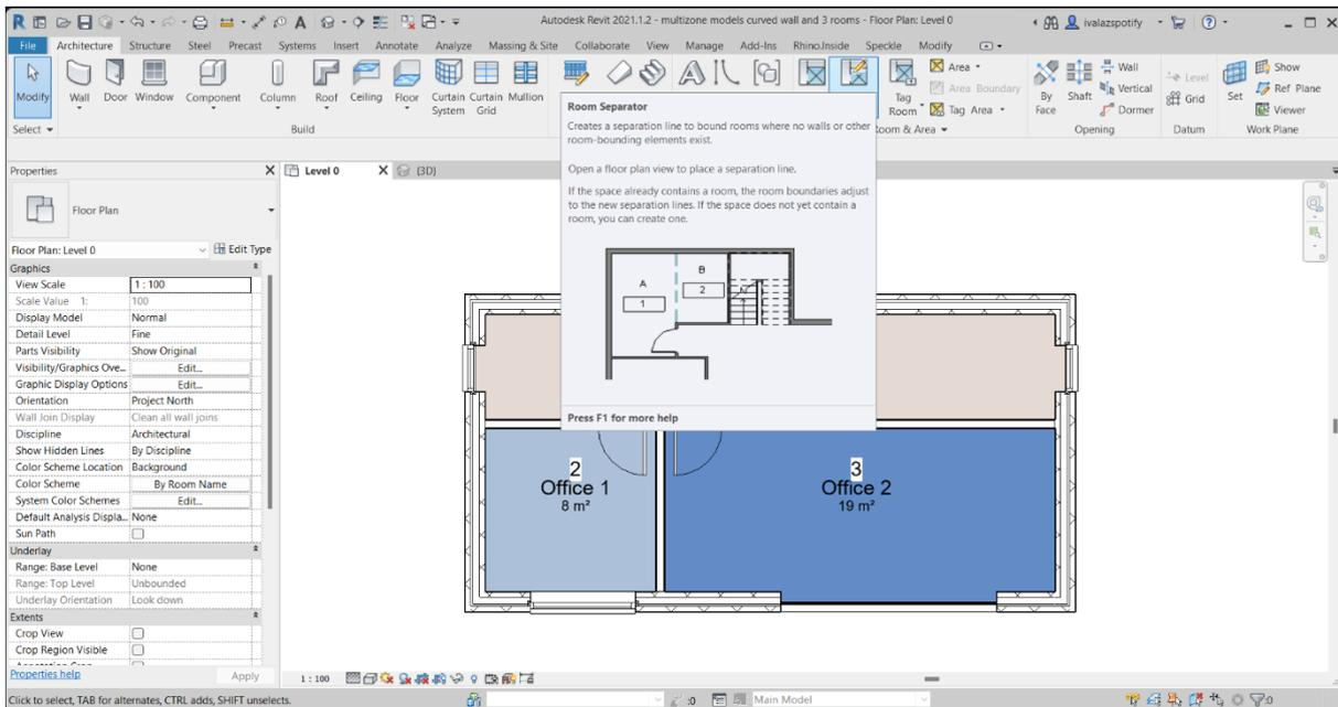
Figure 5.2 Using the command "Room Separator" to construct enclosed room volumes (Case study 3)
