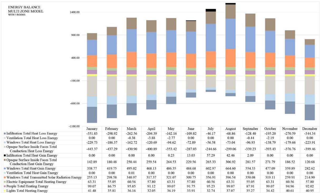
Figure 5.5 Energy balance without louver shades (three zone model)
