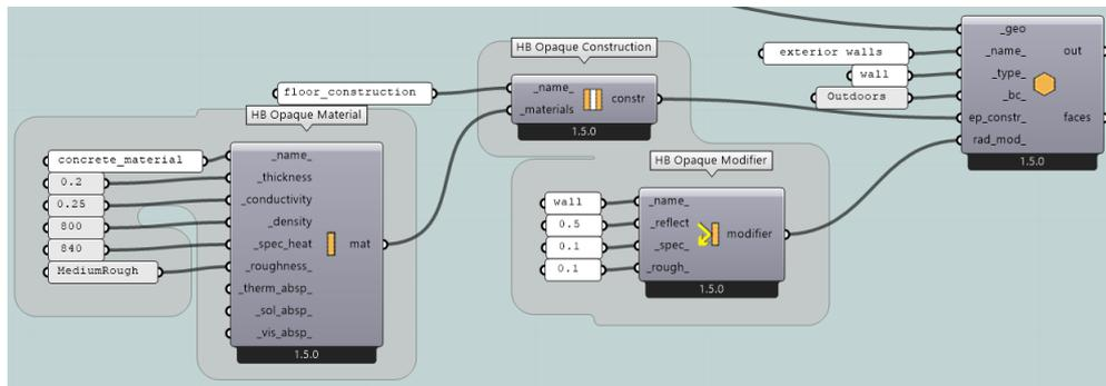
Figure 3.12 “HB Face” algorithm with construction modifier for opaque component-outdoors walls
