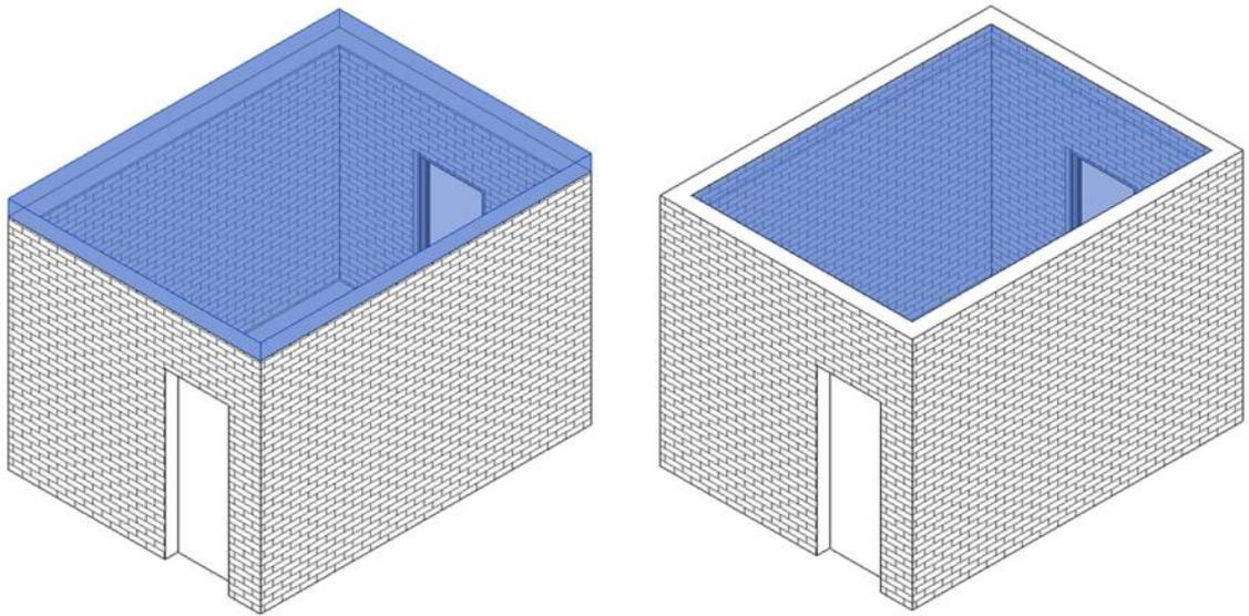
*Figure 3.5 Modified inverted roof extrusion, inside the interior wall surface borders*
