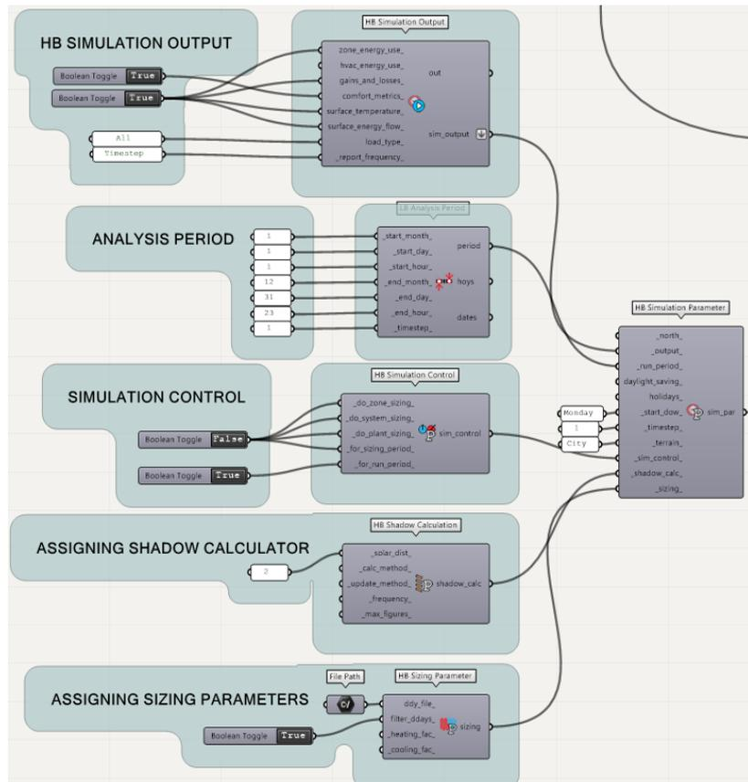
Figure 3.23 Simulation model inputs
