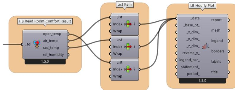
Figure 3.28 “HB Read Room Comfort Results” algorithm for thermal comfort visualization
