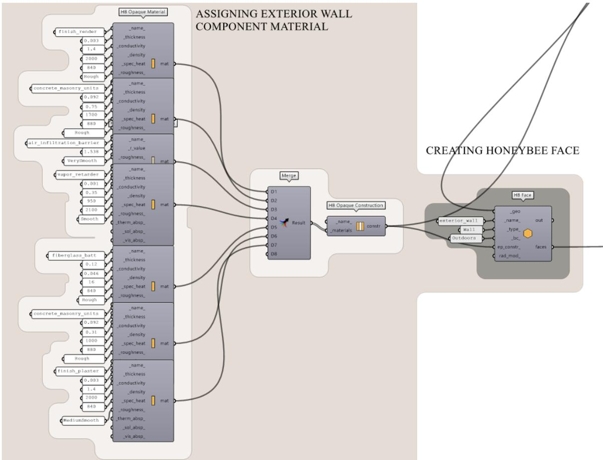
Figure 3.48 "HB Face" algorithm with construction modifier for opaque component-exterior wall
