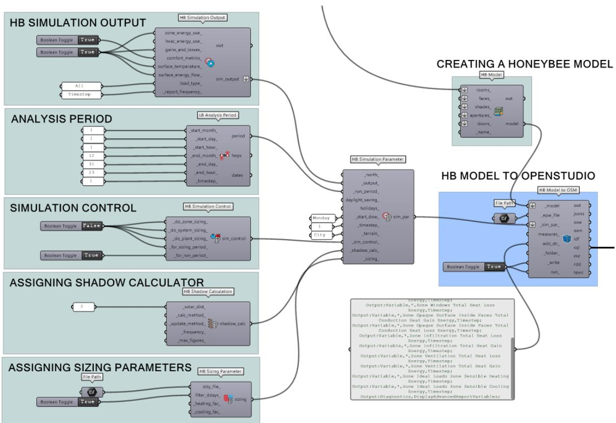
Figure 3.56 Simulation parameters for energy and thermal comfort analysis
