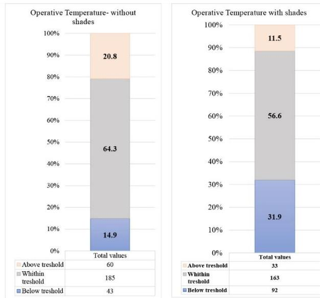
Figure 4.15 Average operative temperatures values below, in and above threshold (multi-zone model)
