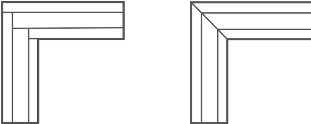
Figure 3.4 Types of wall-joints on Revit 1. BUTT 2. MITTER
