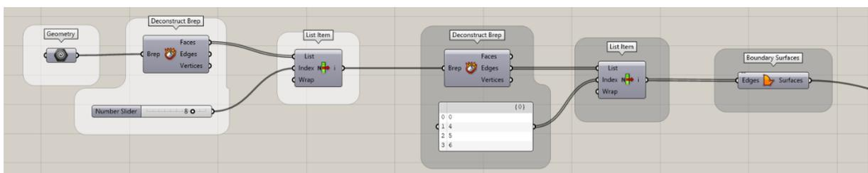
Figure 3.10 Grasshopper workflow of closing the window opening on the south-west facade
