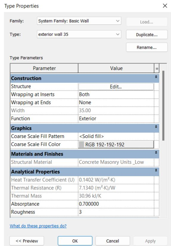
Figure 3.5 "Edit Type" menu on the Revit interface
