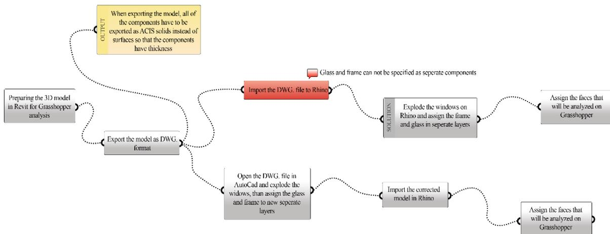
Figure 3.9 Graphical representation of the workflow using .DWG exportation
