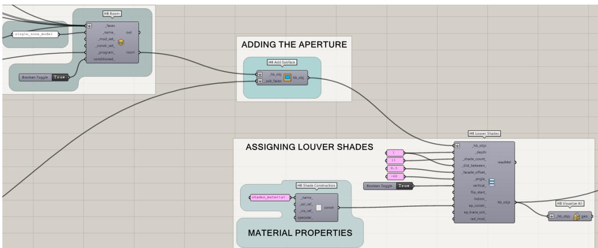
Figure 3.19 Assigning "HB Louver Shades" to the "HB Room" algorithm
