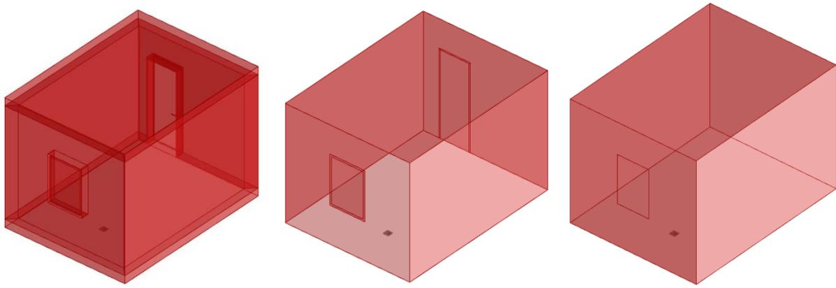
Figure 3.11 Visualized analytical model on Rhino: 1. Imported geometry; 2. Selected surfaces for the analytical model with window and door opening; 3. Closed boundary
