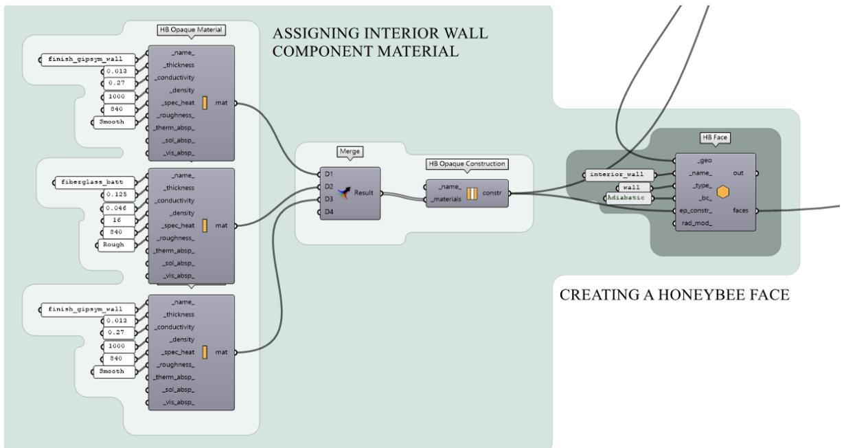
Figure 3.45 "HB Face" algorithm with construction modifier for opaque component- interior wall
