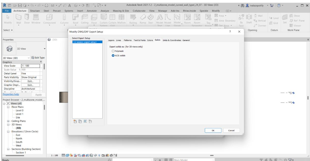
Figure 3.2 Revit “Modify DWG/DXF Export Setup” to export the components as solids
