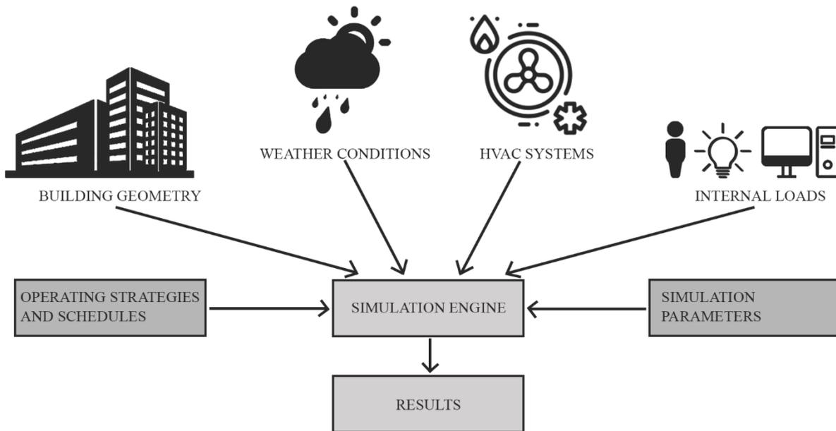
Figure 2.3 Data flow using simulation engines
