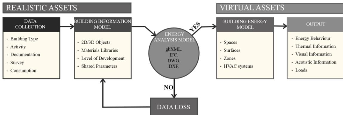
Figure 2.17 Workflow from BIM to BEM
