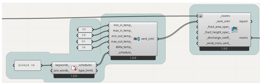
Figure 3.22 Assigning a window control component "HB Window Opening" to apertures
