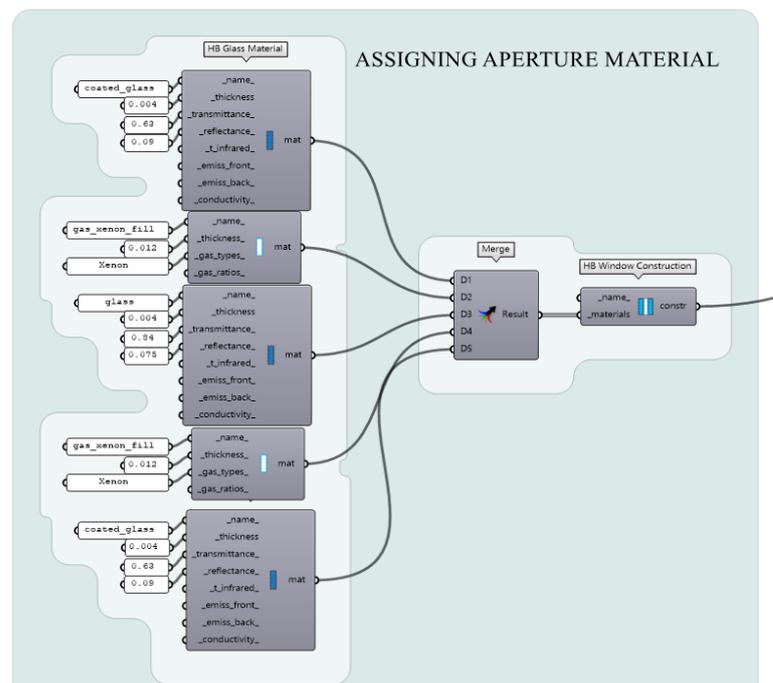
Figure 3.49 Assigning material to the transparent glass component
