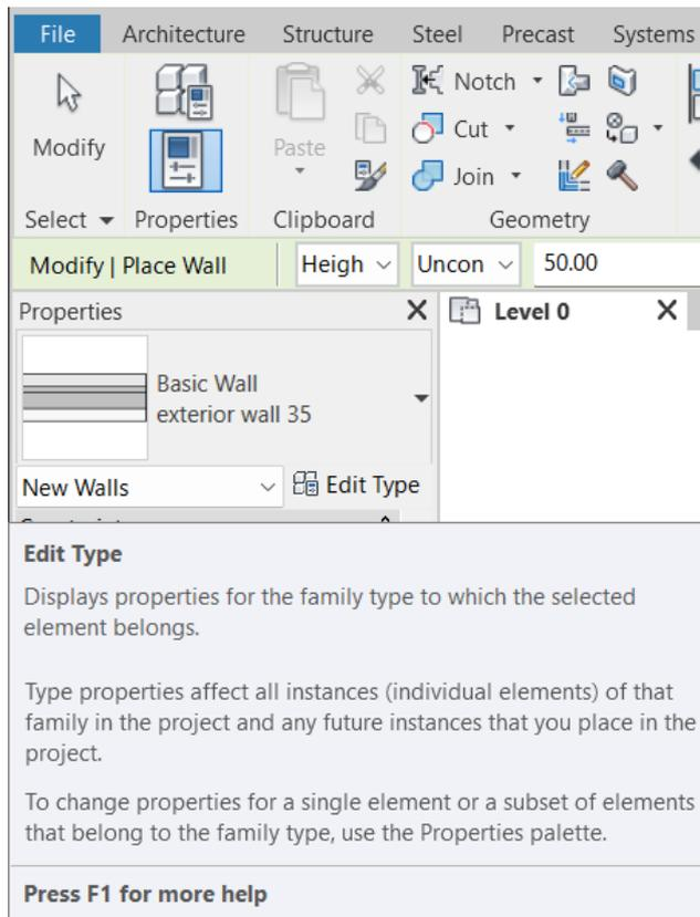
Figure 3.4 Description of "Edit Type" option in Revit for component modification
