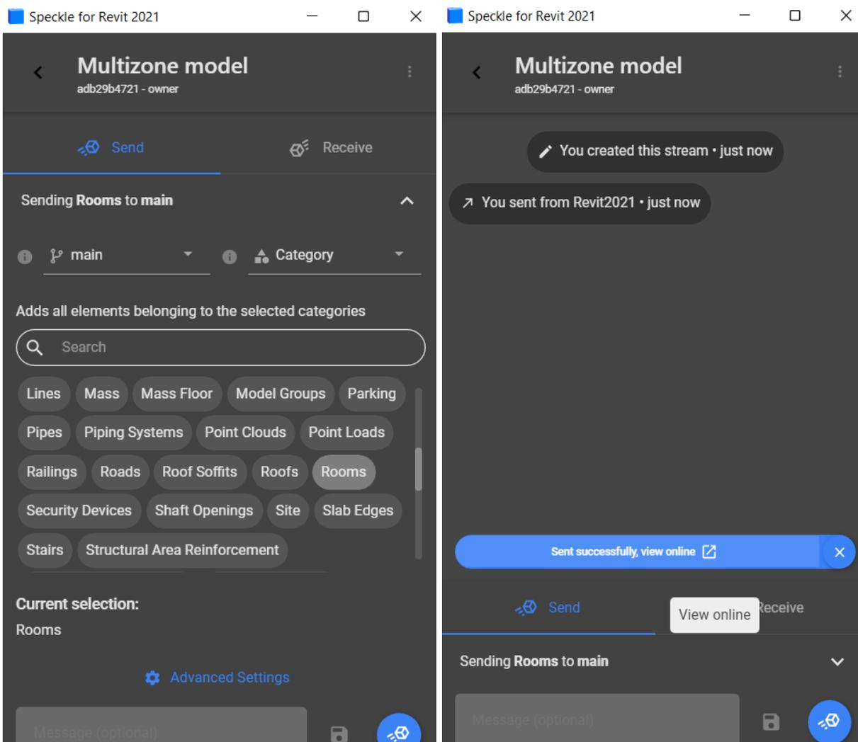
Figure 3.34 1. Choosing the geometry on Revit that will be transferred using the Speckle stream; 2. Speckle stream window that contains the link to the online Speckle cloud
