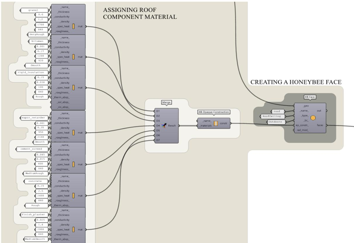
Figure 3.47 "HB Face" algorithm with construction modifier for opaque component-roof
