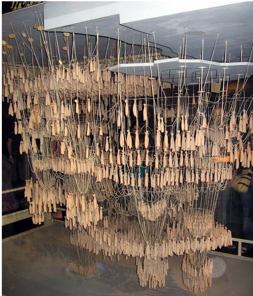
Figure 10: Gaudi's upside-down physical model of the Sagrada Familia
