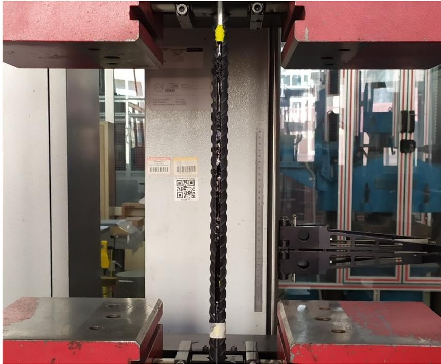
*Figure 4.3 Detail of the rebars undergoing to the test*
