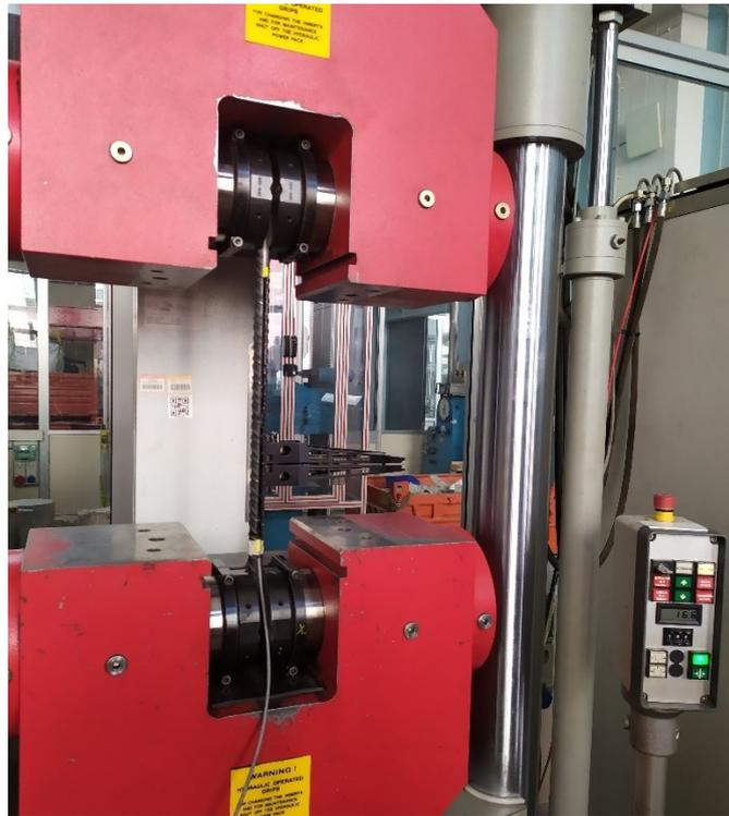
Figure 4.1 Hydraulic machine used for the tensile test
