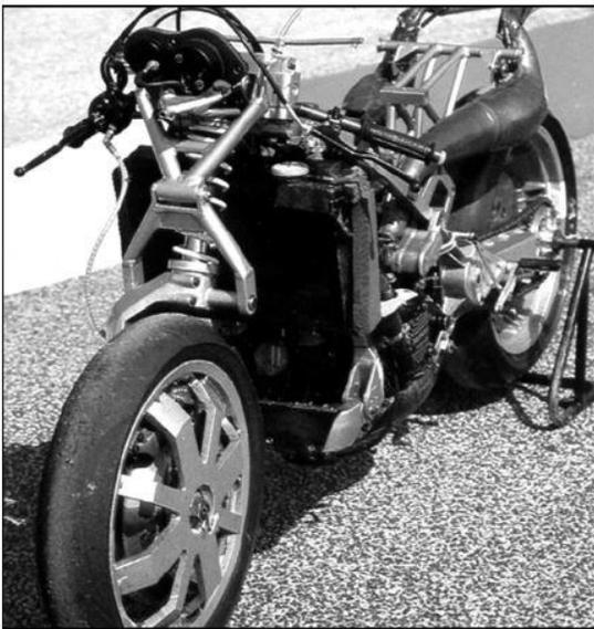
Yet another approach on the Elf bikes (post Cortanze). This design owes much to the McPherson strut, common on modern cars. The typical lower arm is retained but the upper location is done entirely by the suspension unit which has a larger than normal sliding rod.
