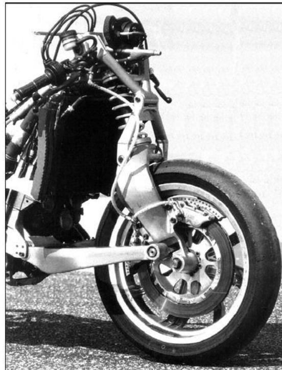
**Fig. 1.9 McPherson strut-based suspension [2]**
