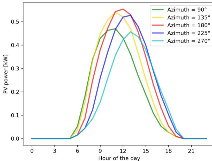
Figure 4.12: Average (over the whole year) daily profiles of PV generation with different orientations, considering a peak power of 1 kW.
