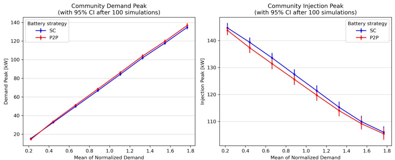
Figure 5.7: Effects of varying the mean of the yearly demand on the community demand peak and injection peak, in the case of energy communities with batteries.
