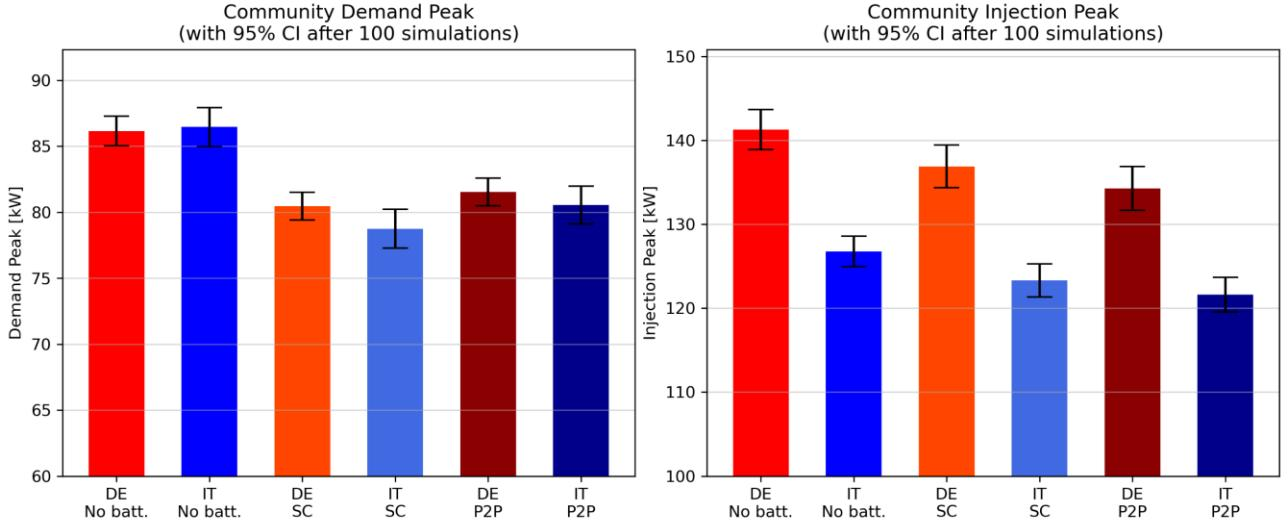
Figure 5.3: Demand peak and injection peak, comparing the German and Italian custom datasets for three subcases relative to batteries.
