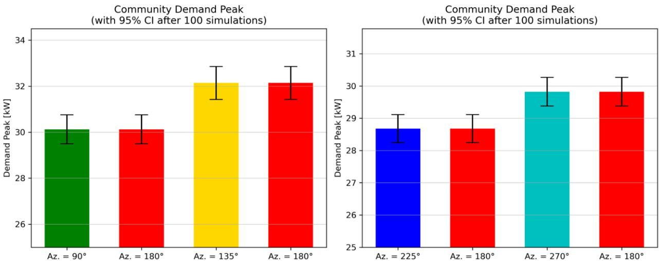
Figure 8.2: Comparisons of demand peak for different PV orientations for the four created datasets with demand profiles whose PCC increased with an orientation different from South.
