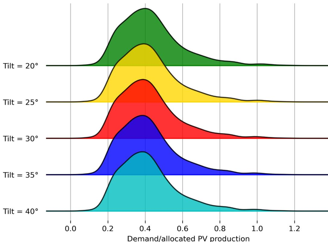
Figure 4.1: Joyplot representing the distributions of normalized demand corresponding to different inclinations of PV systems
