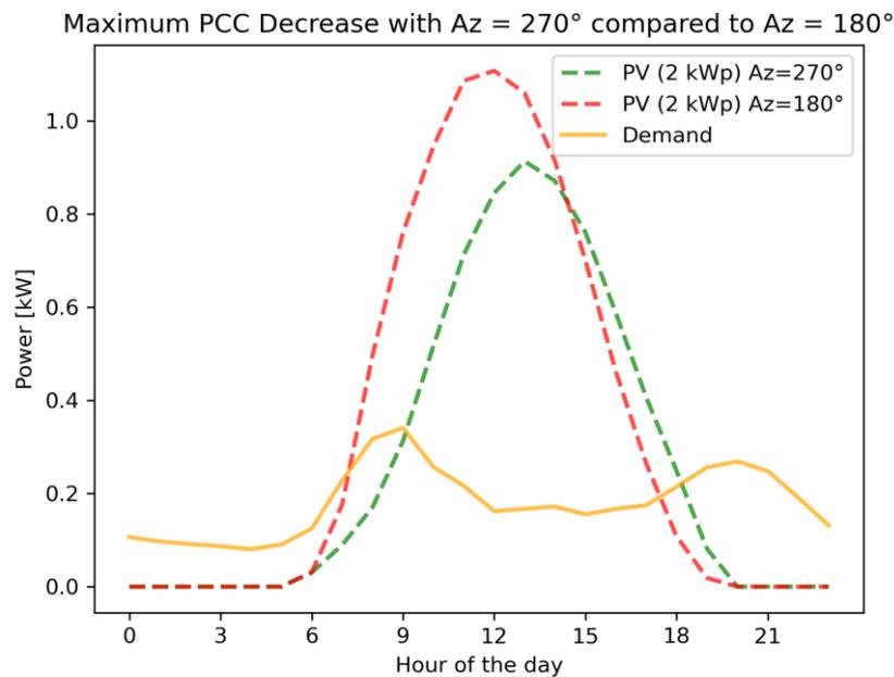
Figure 4.21: Average daily profile of the demand profile whose PCC had the maximum decrease for azimuth angle = 270°, together with the average daily generation profiles of South-oriented and West-oriented PV systems with peak power = 2 kW.
