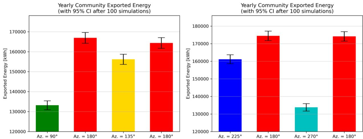
Figure 8.3: Comparisons of yearly exported energy for different PV orientations for the four created datasets with demand profiles whose PCC increased with an orientation different from South.
