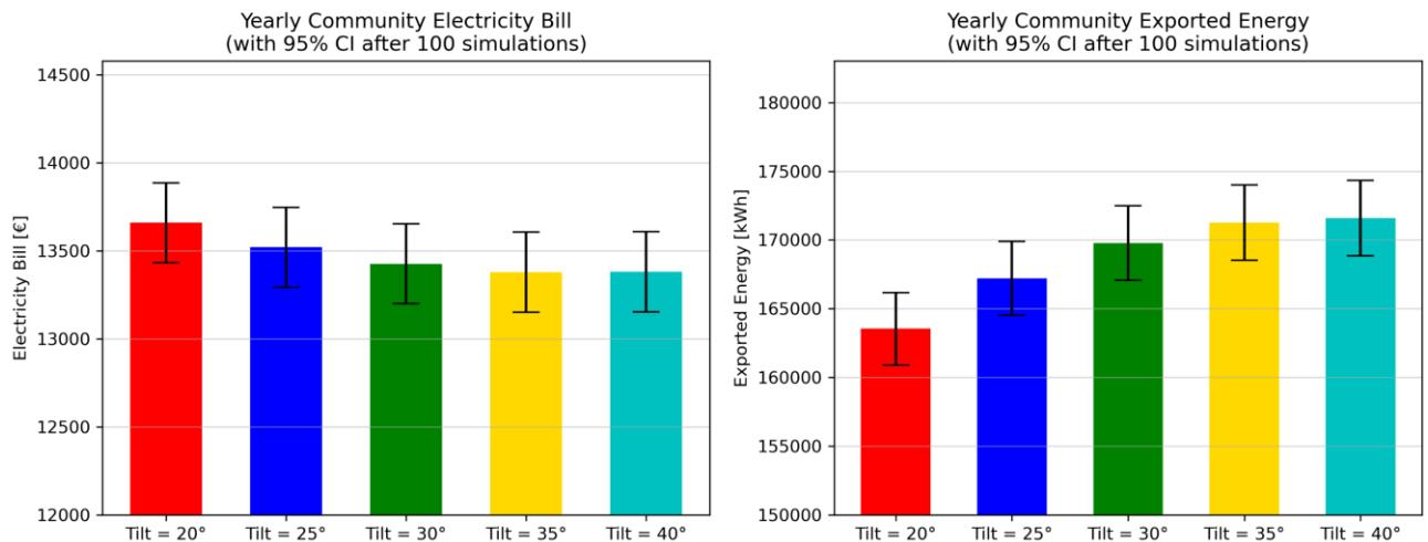
Figure 4.9: Yearly electricity bill and energy exported by the energy community, comparing five different inclinations of PV systems.
