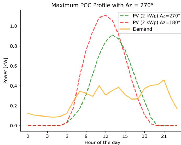
Figure 4.19: Average daily profile of the demand profile with maximum PCC for azimuth angle =  $270^\circ$ , together with the average daily generation profiles of South-oriented and West-oriented PV systems with peak power = 2 kW.
