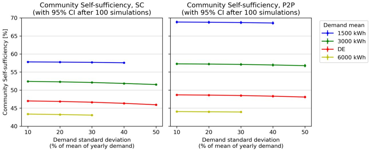
Figure 5.10: Effects of varying the standard deviation of the yearly demand on the community self-sufficiency, in the case of energy communities with batteries.
