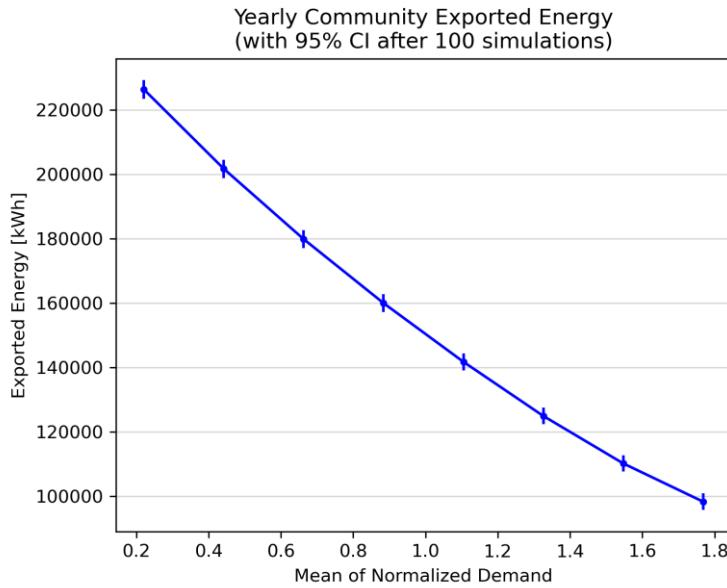
Figure 8.5: Effects of varying the mean of the yearly demand on the yearly energy exported by the community, in the case of energy communities without batteries.
