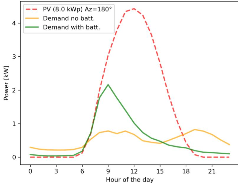
Figure 6.8: Average daily trends of demand with and without batteries and of PV generation relative to the household (number 7) whose PCC had the lowest increase due to batteries.
