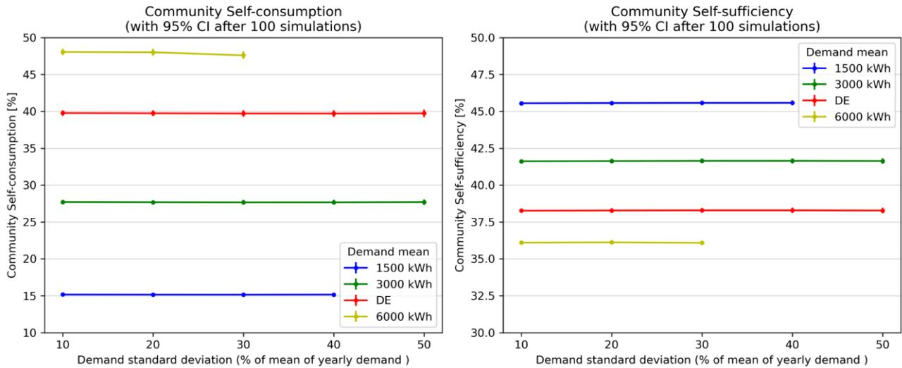
Figure 8.7: Effects of varying the standard deviation of the yearly demand on the community self-consumption and self-sufficiency, in the case of energy communities without batteries.
