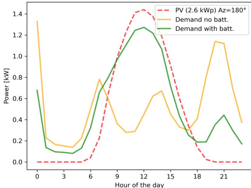
Figure 6.9: Average daily trends of demand with and without batteries and of PV generation relative to the household (number 4) whose PCC had the highest increase due to batteries.
