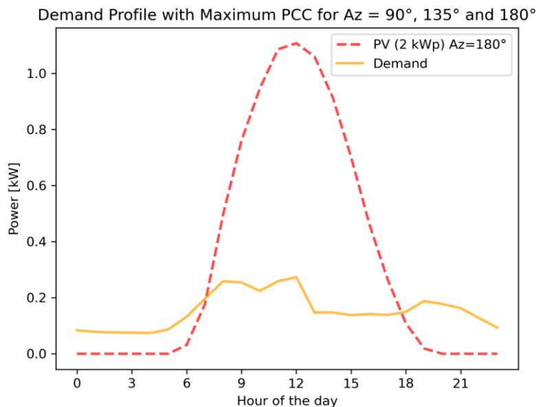
Figure 4.18: Average daily profile of the demand profile with maximum PCC for azimuth angles =  $90^\circ$ ,  $135^\circ$ , and  $180^\circ$ , together with the average daily generation profile of a South-oriented PV system with peak power = 2 kW.
