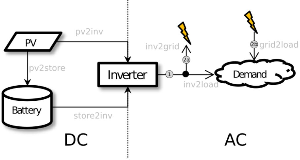
Figure 6.4: Technologies and power flows present in a household with a battery and a PV system [28].
