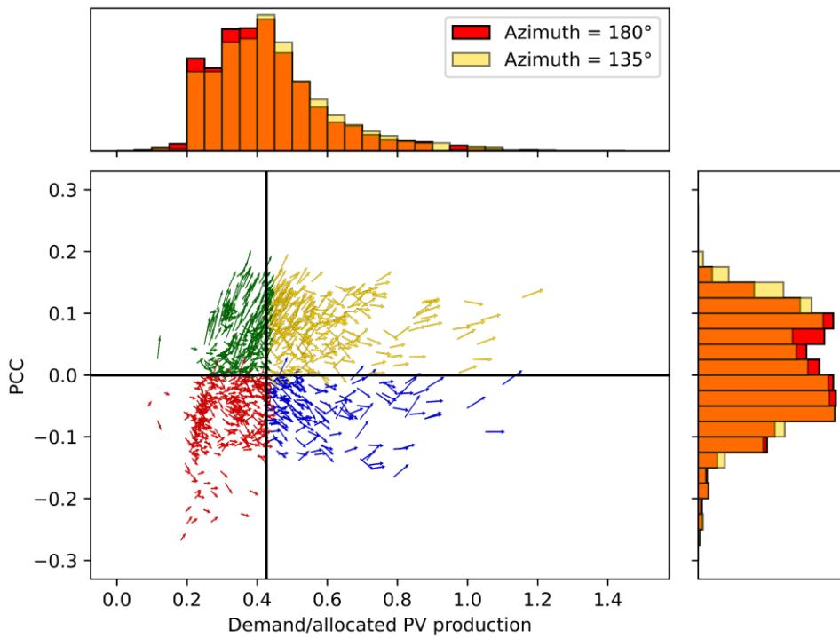
Figure 4.15: Arrow plot (in the PCC-demand plane with normalized demand) and frequency distributions of PCC and normalized demand, comparing South orientation and South-East orientation.
