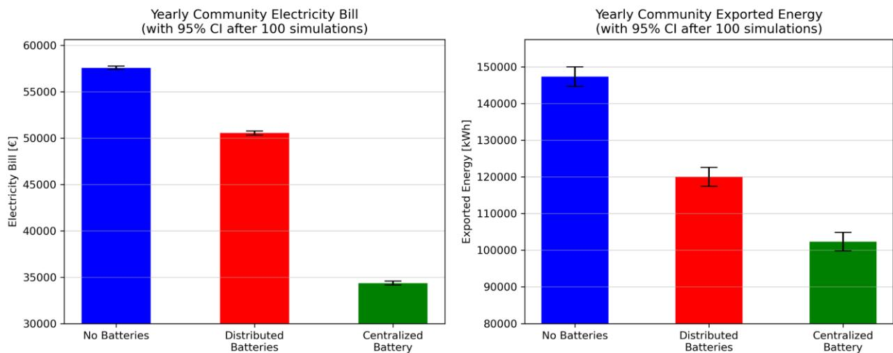
Figure 6.2: Yearly electricity bill and energy exported by the energy community, comparing three cases relative to batteries.
