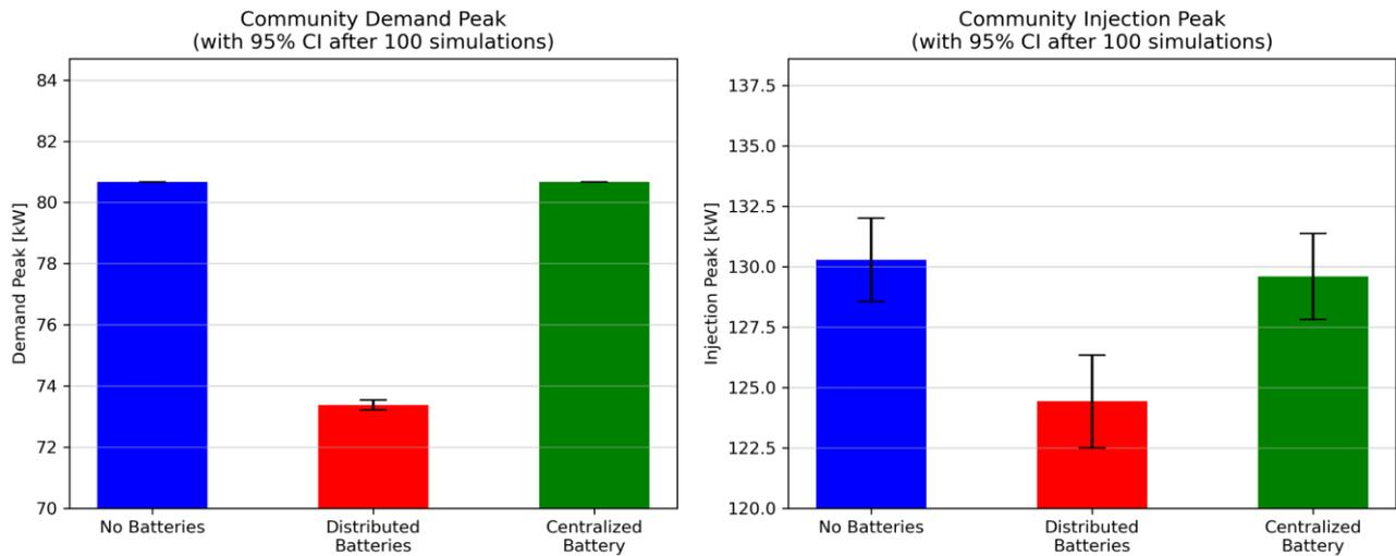
Figure 6.3: Demand peak and injection peak, comparing three cases relative to batteries.
