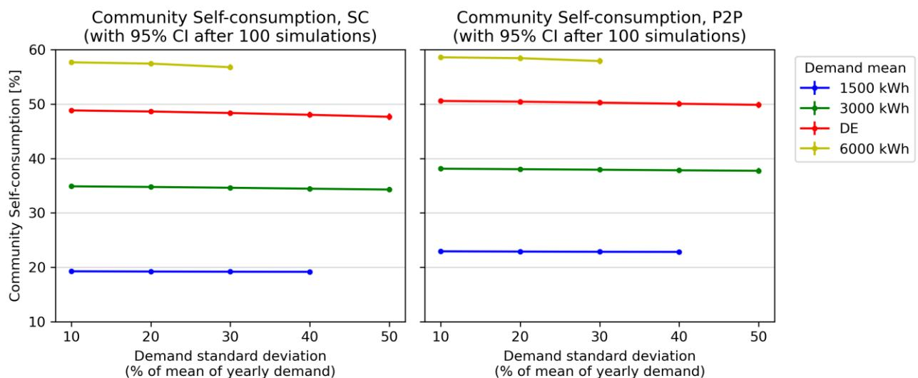
Figure 5.9: Effects of varying the standard deviation of the yearly demand on the community self-consumption, in the case of energy communities with batteries.
