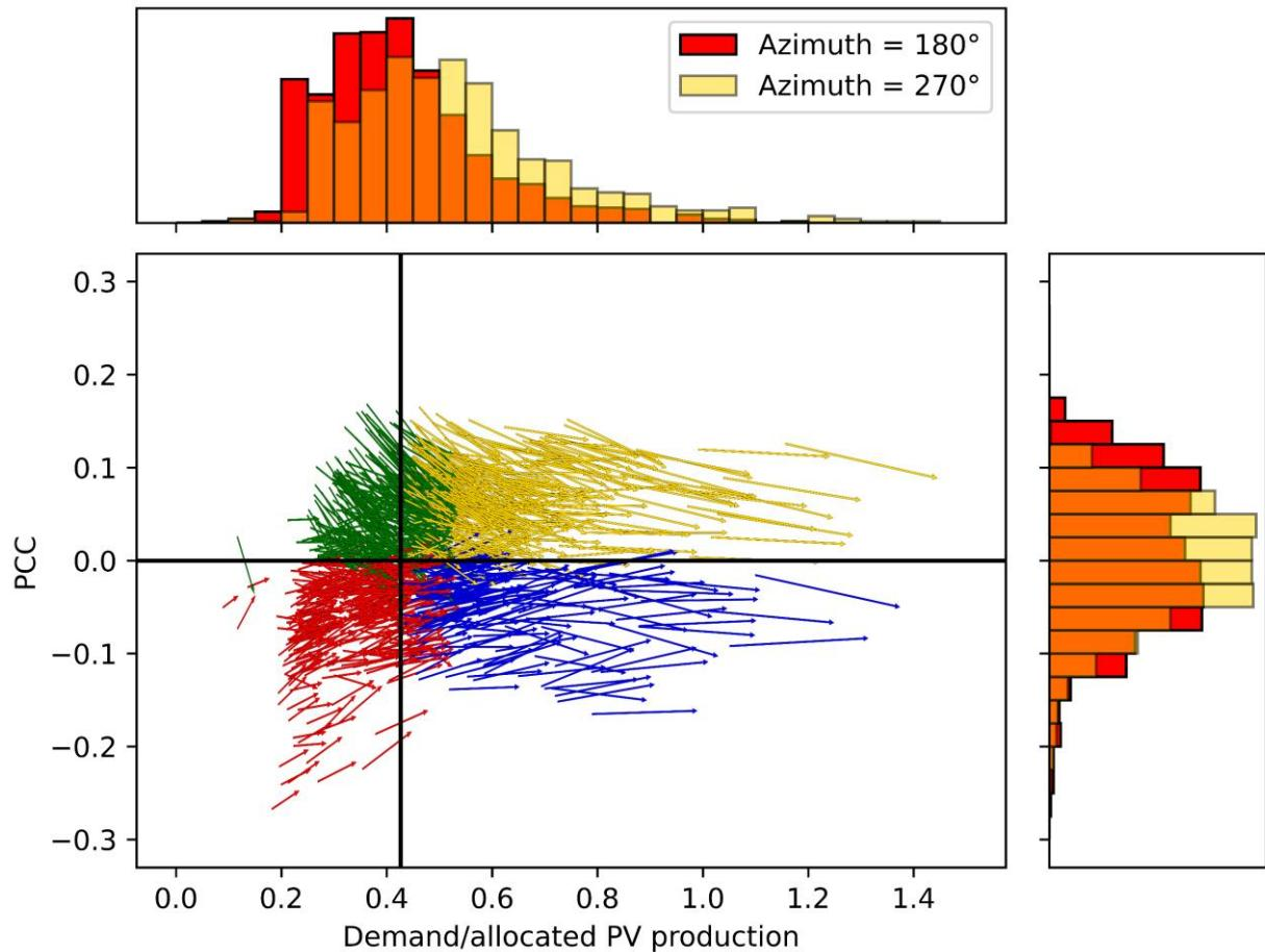
Figure 4.17: Arrow plot (in the PCC-demand plane with normalized demand) and frequency distributions of PCC and normalized demand, comparing South orientation and West orientation.
