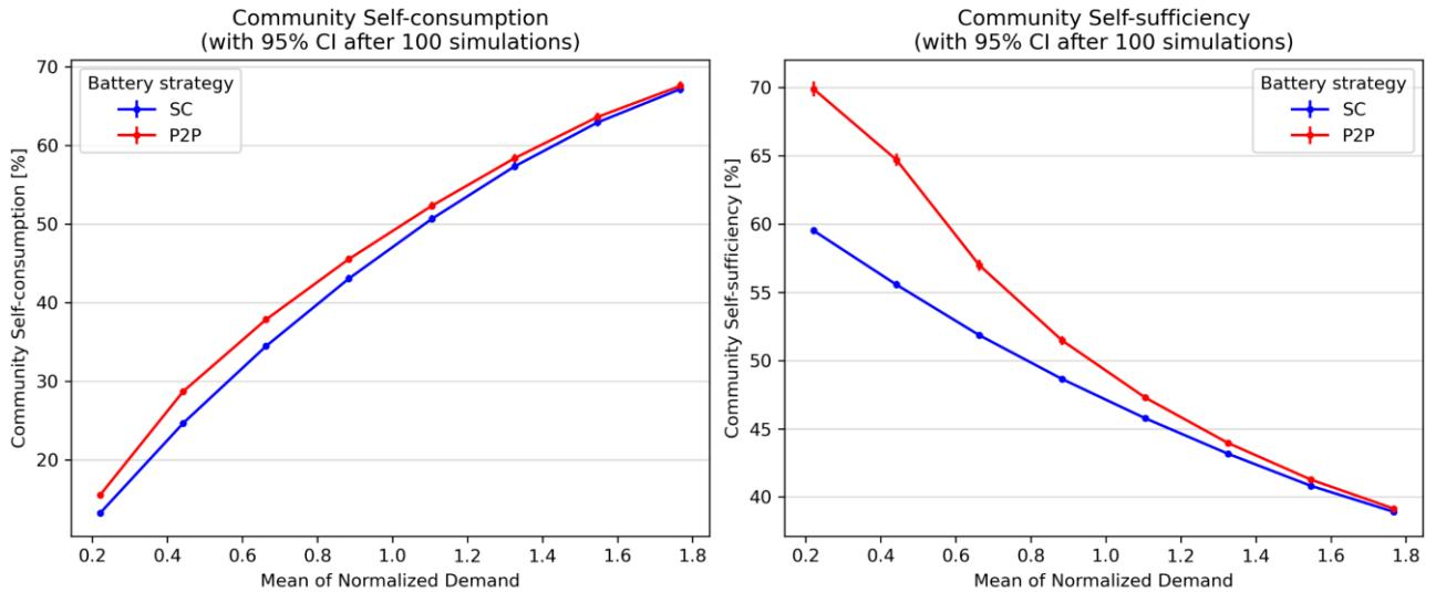
Figure 5.5: Effects of varying the mean of the yearly demand on the community self-consumption and self-sufficiency, in the case of energy communities with batteries.
