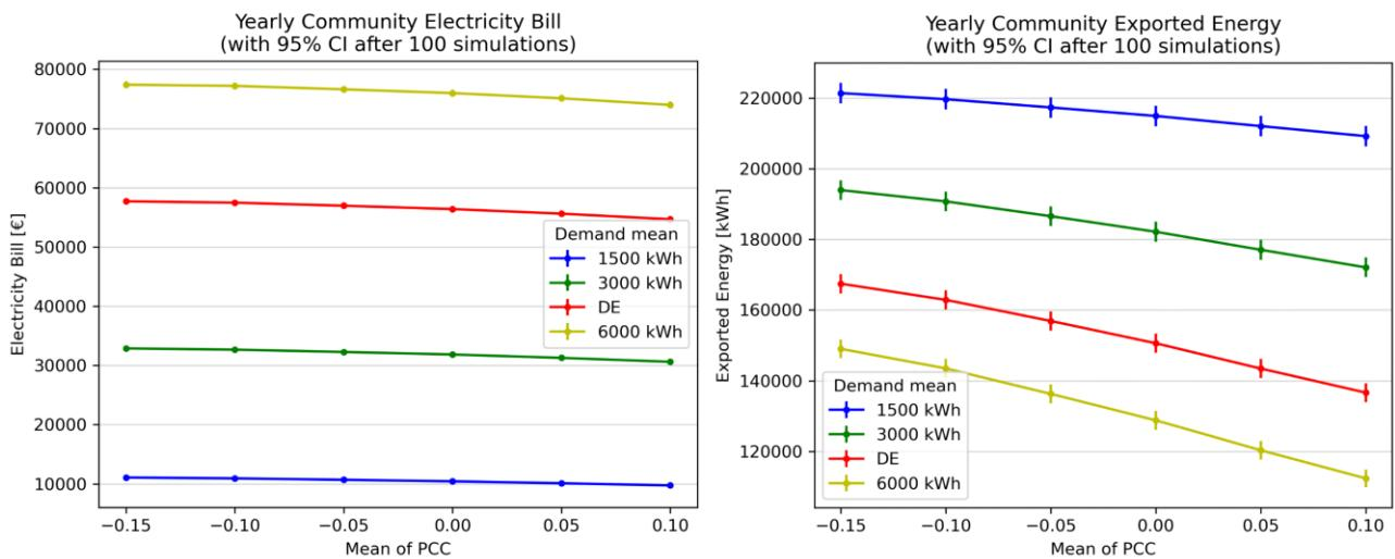
Figure 8.11: Effects of varying the mean of the PCC on the yearly electricity bill and energy exported by the community, in the case of energy communities without batteries.
