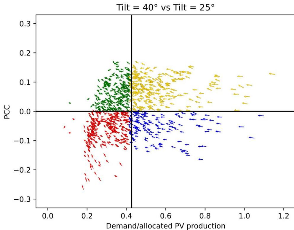
Figure 4.7: Arrow plot in the PCC-demand plane with normalized demand, comparing an inclination of 25° (at the start of the arrows) and an inclination of 40° (at the end of the arrows).
