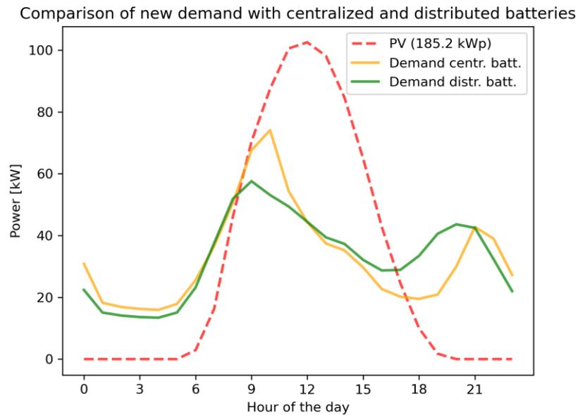
Figure 6.6: Average PV daily generation and average daily trends of the overall new demand for one simulation in the cases of centralized and distributed batteries.
