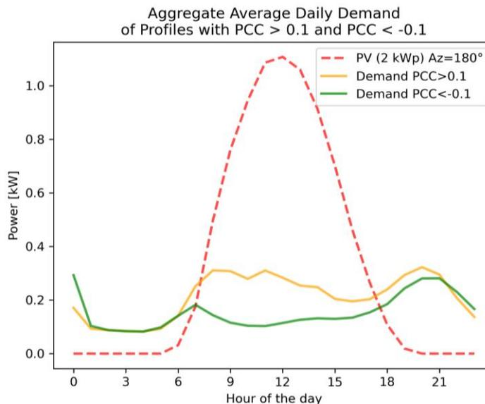
Figure 4.23: Aggregate average daily profile of demand profiles with  $PCC > 0.1$  and of demand profiles with  $PCC < -0.1$ , together with the average daily generation profile of a South-oriented PV system with peak power = 2 kW.
