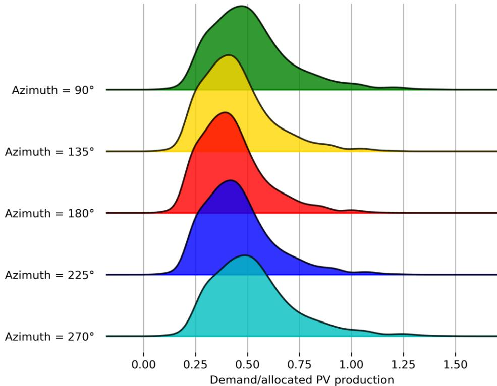
Figure 4.11: Joyplot representing the distributions of normalized demand corresponding to different orientations of PV systems.
