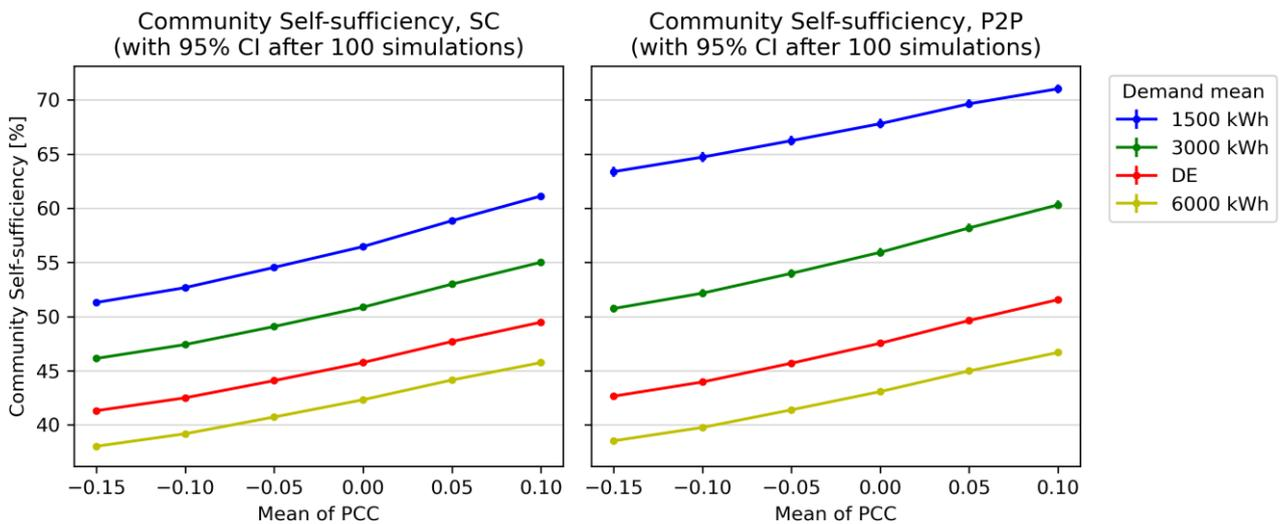
Figure 5.16: Effects of varying the mean of the PCC on the community self-sufficiency, in the case of energy communities with batteries.
