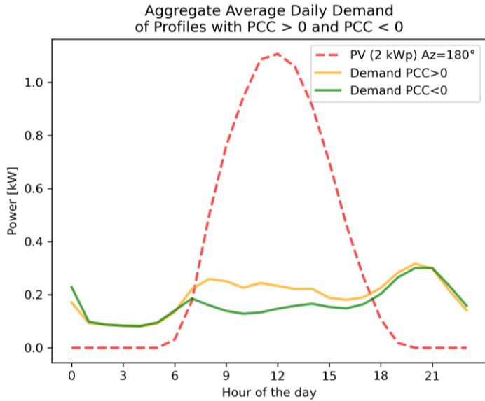
Figure 4.22: Aggregate average daily profile of demand profiles with PCC > 0 and of demand profiles with PCC < 0, together with the average daily generation profile of a South-oriented PV system with peak power = 2 kW.
