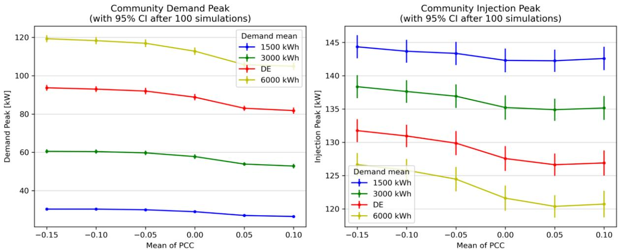
Figure 8.12: Effects of varying the mean of the PCC on the community demand peak and injection peak, in the case of energy communities without batteries.
