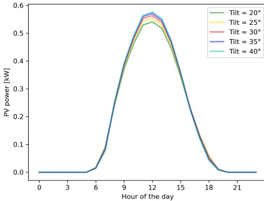
Figure 4.2: Average (over the whole year) daily profiles of PV generation with different inclinations, considering a peak power of 1 kW.
