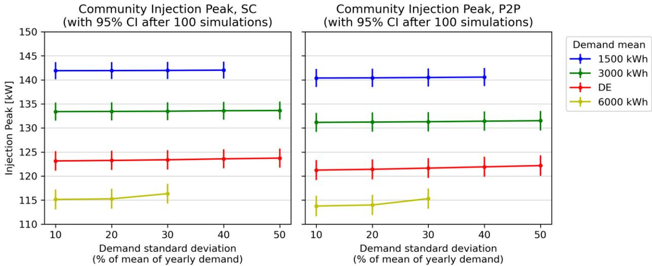
Figure 5.14: Effects of varying the standard deviation of the yearly demand on the community injection peak, in the case of energy communities with batteries.
