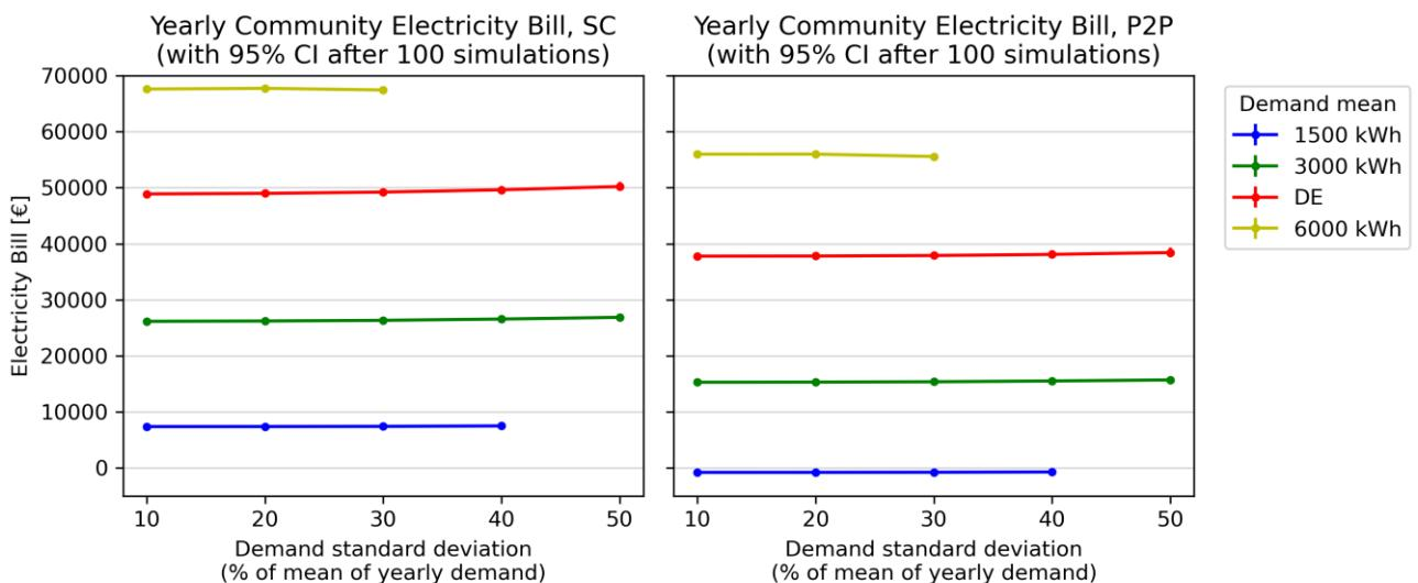
Figure 5.11: Effects of varying the standard deviation of the yearly demand on the community yearly electricity bill, in the case of energy communities with batteries.
