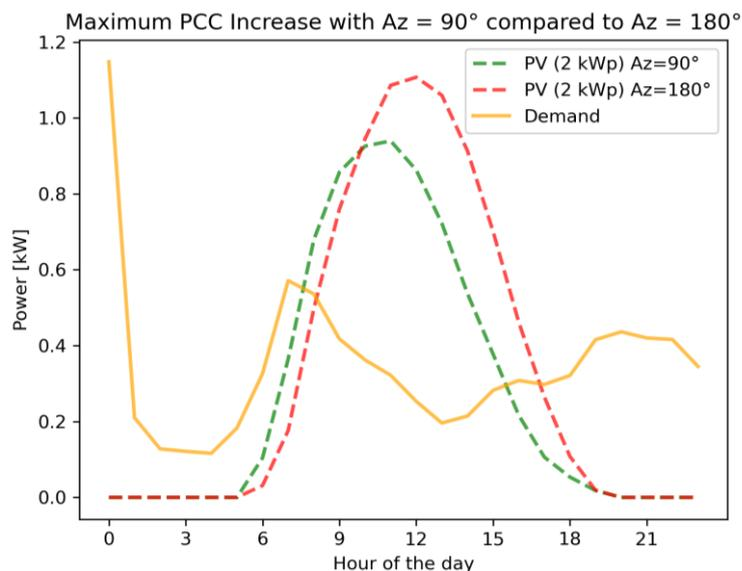
Figure 4.24: Average daily profile of the demand profile whose PCC had the maximum increase for azimuth angle = 90°, together with the average daily generation profiles of South-oriented and East-oriented PV systems with peak power = 2 kW.
