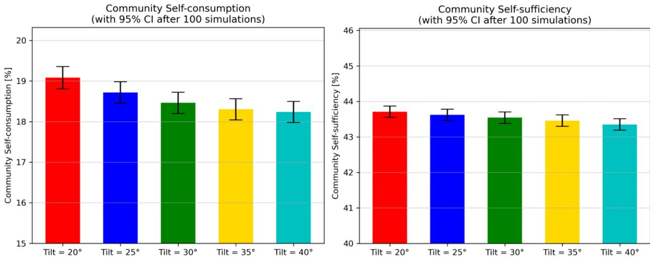
Figure 4.8: Self-sufficiency and self-consumption of the energy community, comparing five different inclinations of PV systems.
