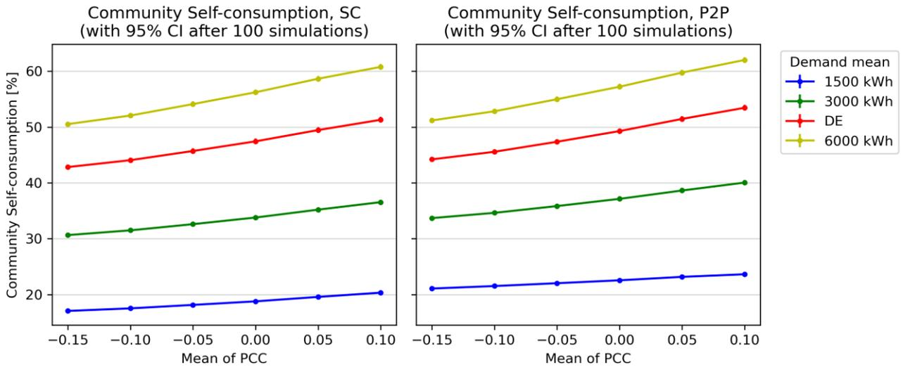
Figure 5.15: Effects of varying the mean of the PCC on the community self-consumption, in the case of energy communities with batteries.
