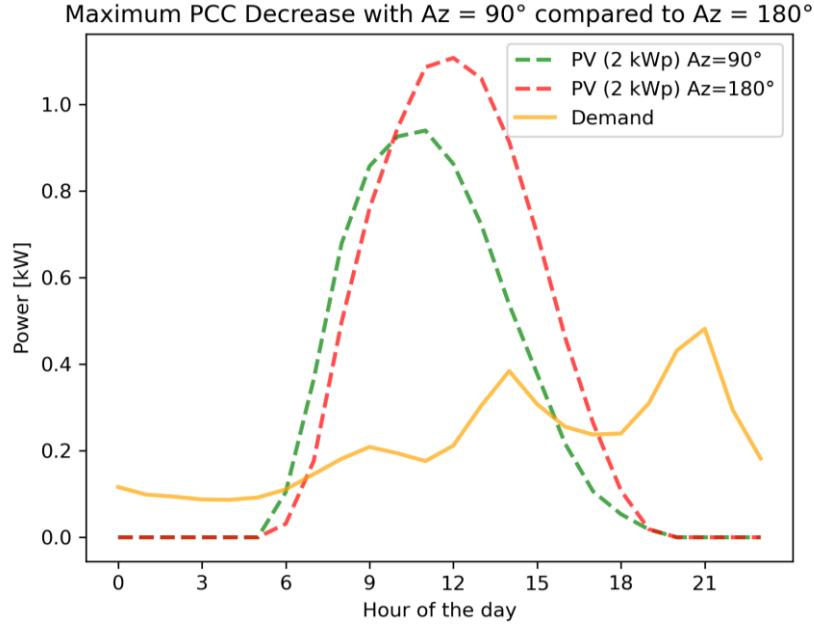
Figure 4.25: Average daily profile of the demand profile whose PCC had the maximum decrease for azimuth angle =  $90^\circ$ , together with the average daily generation profiles of South-oriented and East-oriented PV systems with peak power = 2 kW.
