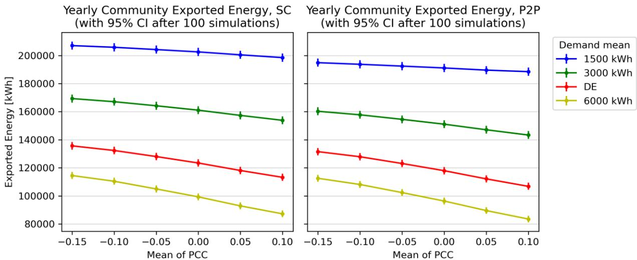
Figure 5.17: Effects of varying the mean of the PCC on the energy exported in a year by the community, in the case of energy communities with batteries.
