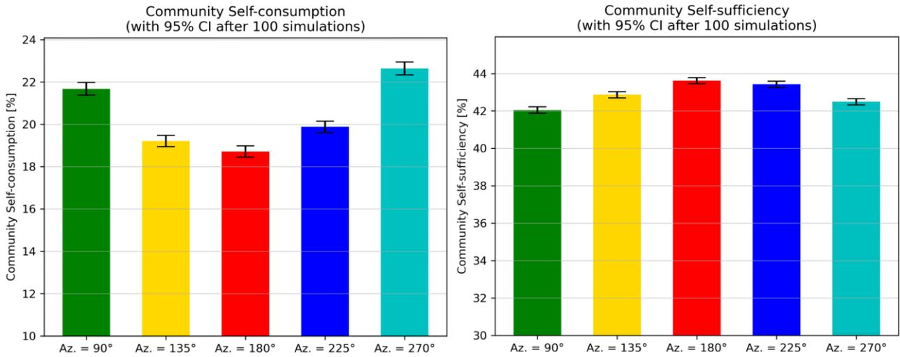
Figure 4.26: Self-sufficiency and self-consumption of the energy community, comparing five different orientations of PV systems.
