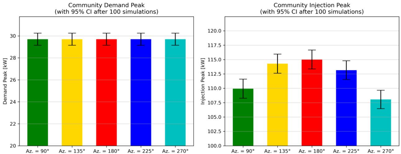
Figure 4.28: Demand peak and injection peak, comparing five different orientations of PV systems.
