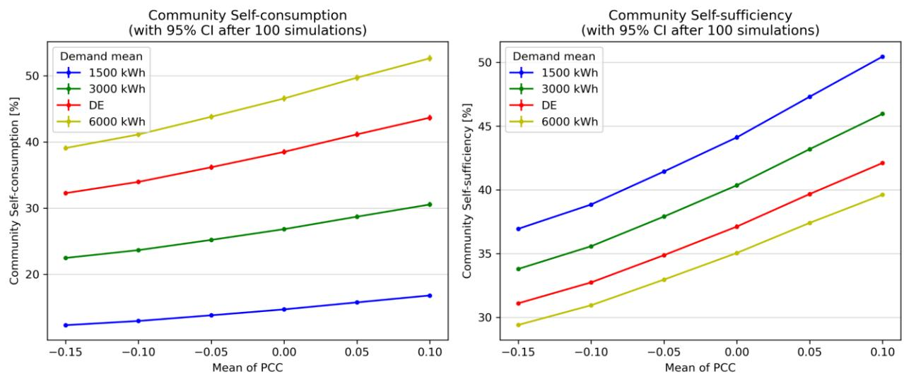
Figure 8.10: Effects of varying the mean of the PCC on the community self-consumption and self-sufficiency, in the case of energy communities without batteries.
