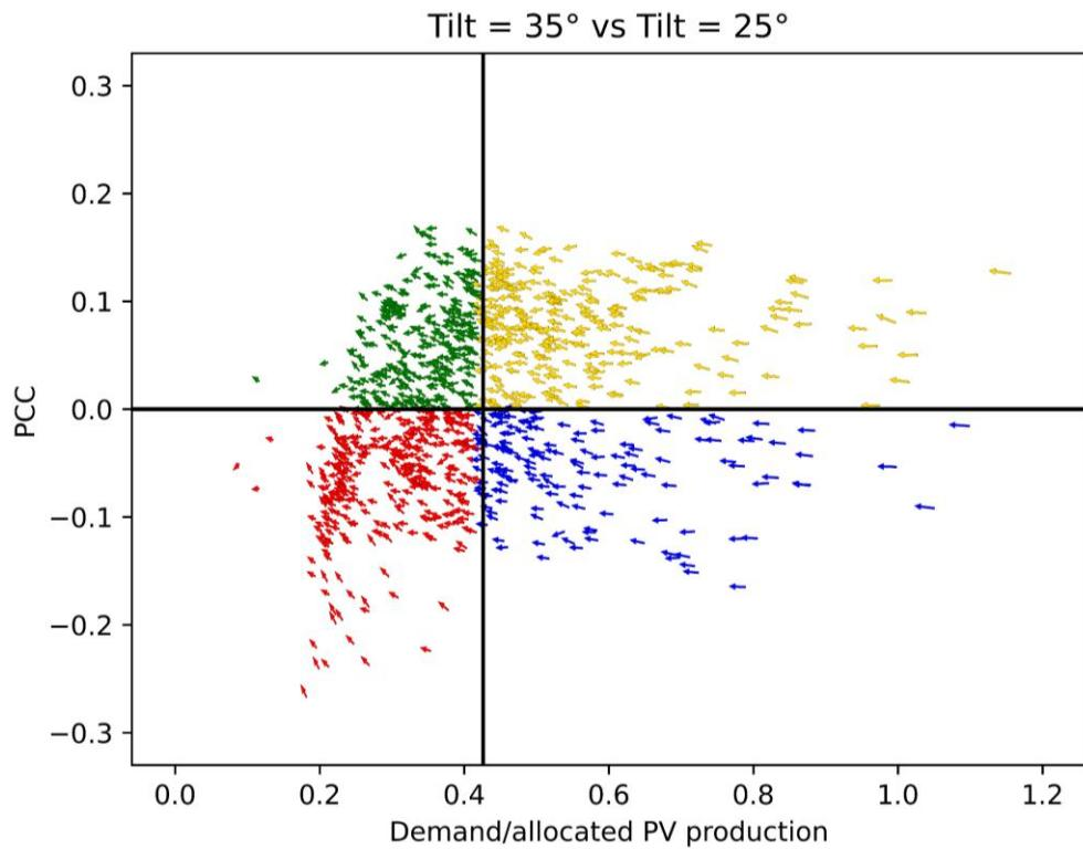
Figure 4.6: Arrow plot in the PCC-demand plane with normalized demand, comparing an inclination of 25° (at the start of the arrows) and an inclination of 35° (at the end of the arrows).
