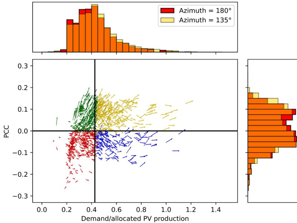
Figure 4.15: Arrow plot (in the PCC-demand plane with normalized demand) and frequency distributions of PCC and normalized demand, comparing South orientation and South-East orientation.
