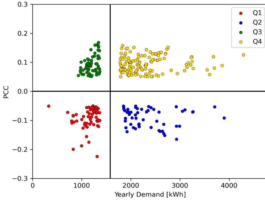
Figure 3.2: Demand profiles selected for the investigation of the effects of belonging to the four different quadrants, after the removal of some profiles from Q1.
