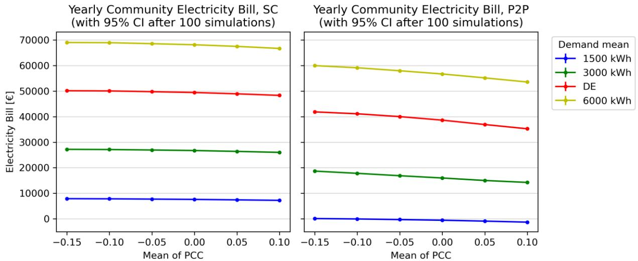
Figure 5.18: Effects of varying the mean of the PCC on the community yearly electricity bill, in the case of energy communities with batteries.
