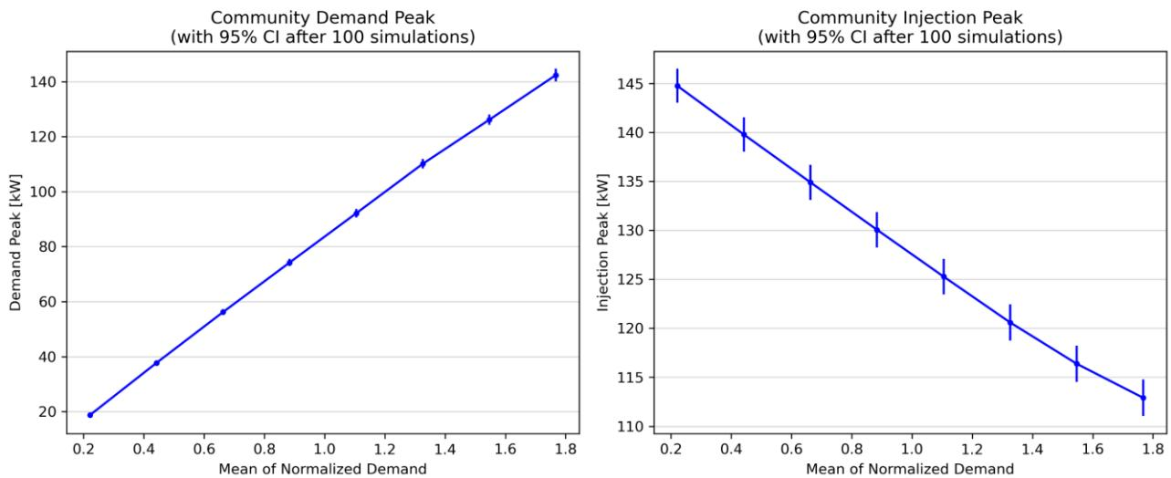
Figure 8.6: Effects of varying the mean of the yearly demand on the community demand peak and injection peak, in the case of energy communities without batteries.
