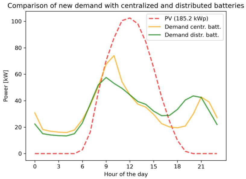
Figure 6.6: Average PV daily generation and average daily trends of the overall new demand for one simulation in the cases of centralized and distributed batteries.
