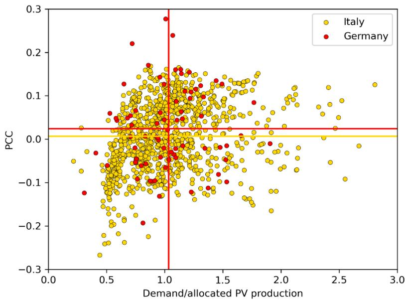
Figure 2.8: Representation on the PCC-demand plane with normalized demand of the German dataset and the Italian dataset, considering an average PV power of 2.06 kW for the latter.
