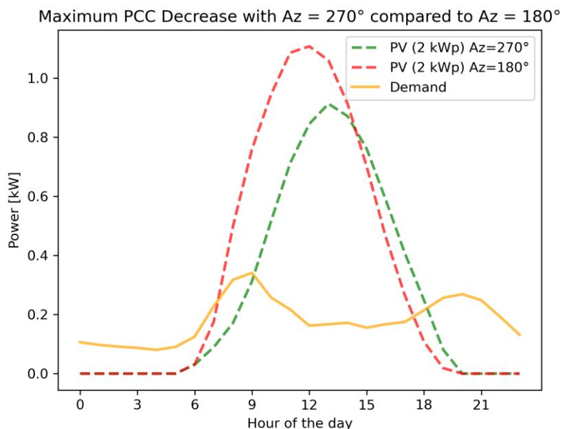
Figure 4.21: Average daily profile of the demand profile whose PCC had the maximum decrease for azimuth angle =  $270^\circ$ , together with the average daily generation profiles of South-oriented and West-oriented PV systems with peak power = 2 kW.
