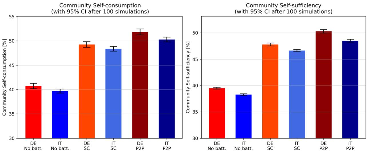
Figure 5.1: Self-sufficiency and self-consumption of the energy community, comparing the German and Italian custom datasets for three subcases relative to batteries.
