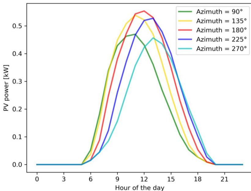
Figure 4.12: Average (over the whole year) daily profiles of PV generation with different orientations, considering a peak power of 1 kW.
