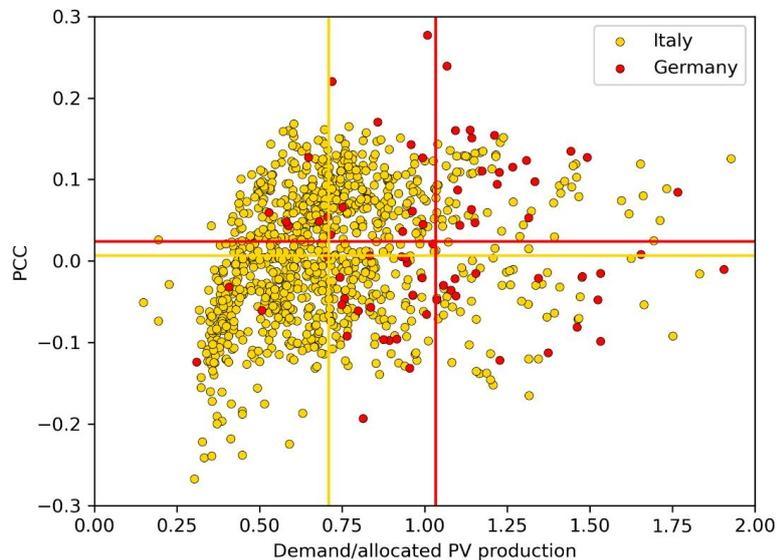
Figure 2.7: Representation on the PCC-demand plane with normalized demand of the German dataset and the Italian dataset, considering an average PV power of 3 kW for the latter.
