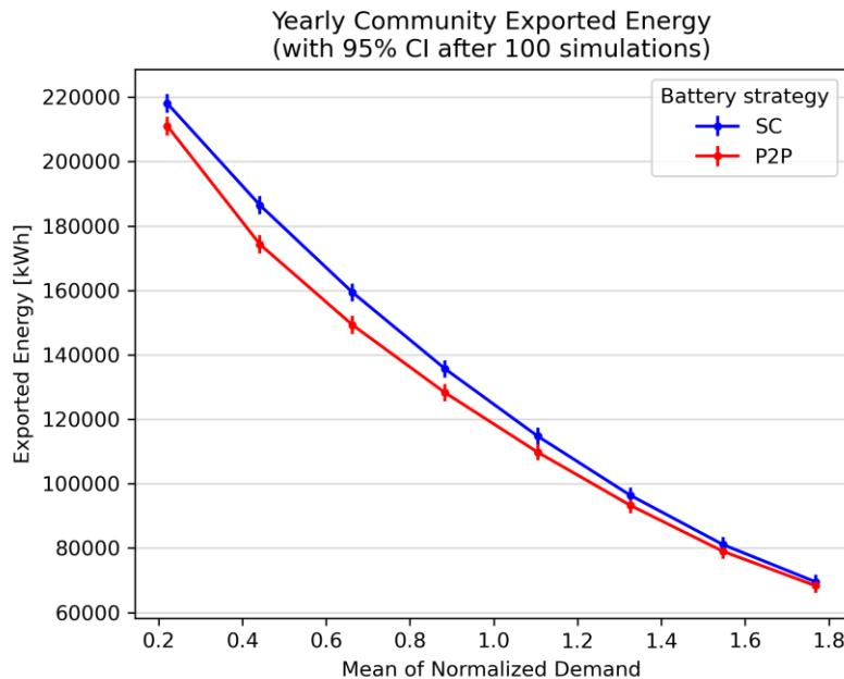
Figure 5.6: Effects of varying the mean of the yearly demand on the yearly energy exported by the community, in the case of energy communities with batteries.
