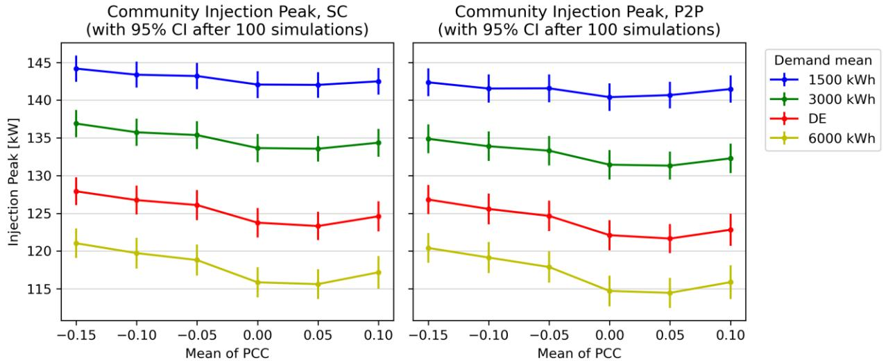
Figure 5.20: Effects of varying the mean of the PCC on the community injection peak, in the case of energy communities with batteries.
