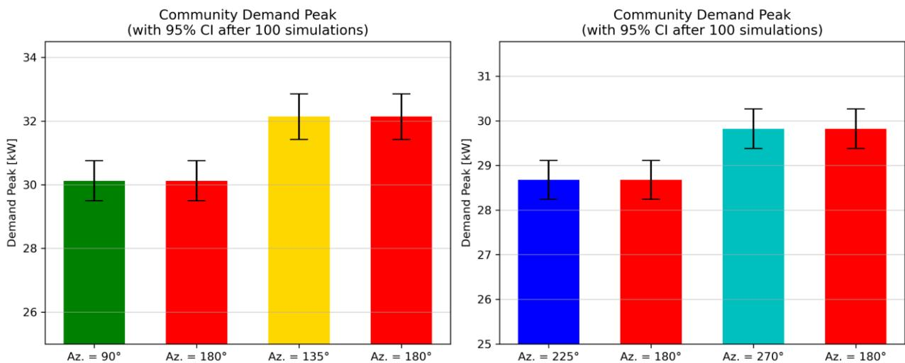
Figure 8.2: Comparisons of demand peak for different PV orientations for the four created datasets with demand profiles whose PCC increased with an orientation different from South.
