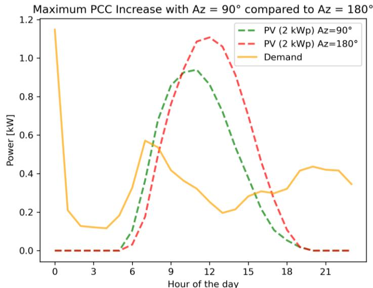
Figure 4.24: Average daily profile of the demand profile whose PCC had the maximum increase for azimuth angle =  $90^\circ$ , together with the average daily generation profiles of South-oriented and East-oriented PV systems with peak power = 2 kW.
