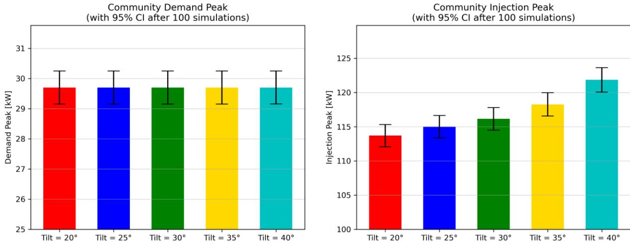
Figure 4.10: Demand peak and injection peak, comparing five different inclinations of PV systems.
