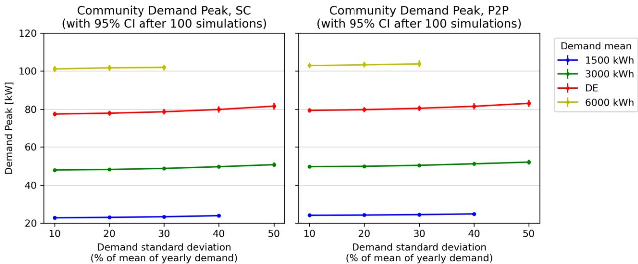
Figure 5.13: Effects of varying the standard deviation of the yearly demand on the community demand peak, in the case of energy communities with batteries.
