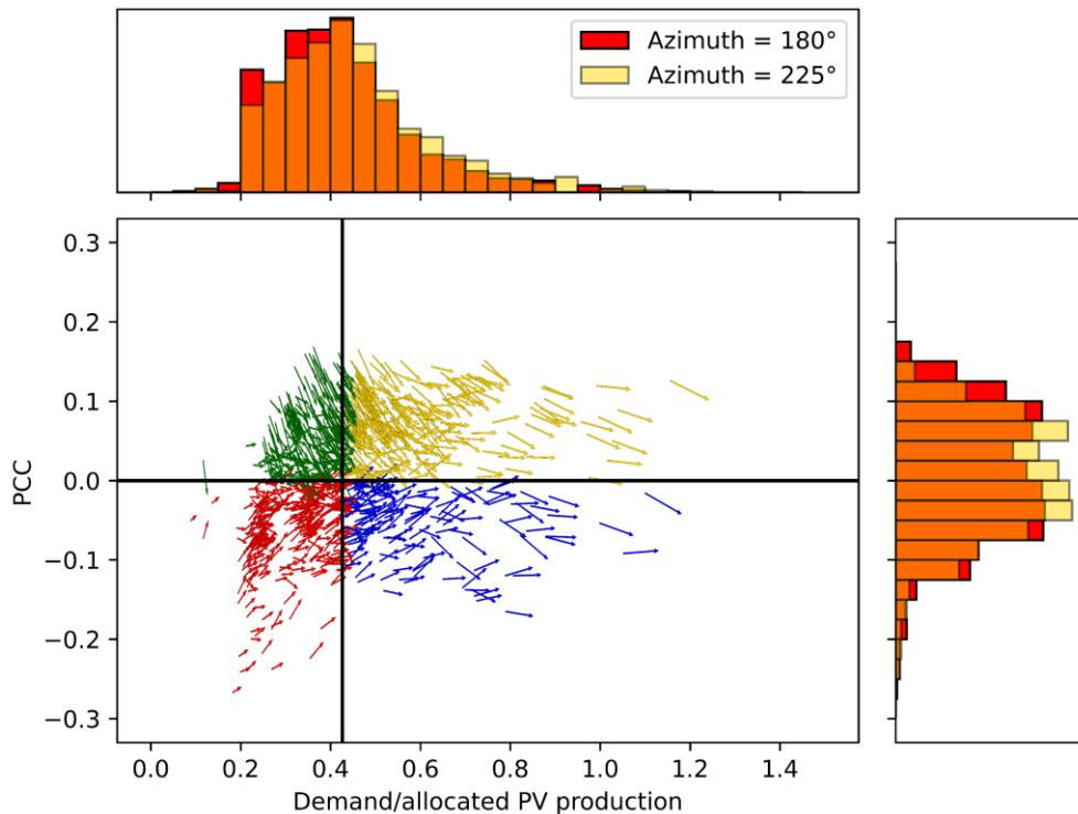
Figure 4.16: Arrow plot (in the PCC-demand plane with normalized demand) and frequency distributions of PCC and normalized demand, comparing South orientation and South-West orientation.
