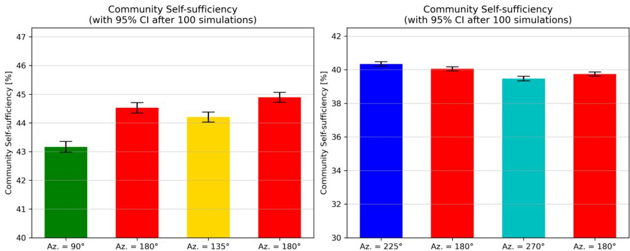
Figure 4.31: Comparisons of community self-sufficiency for different PV orientations for the four created datasets with demand profiles whose PCC increased with an orientation different from South.
