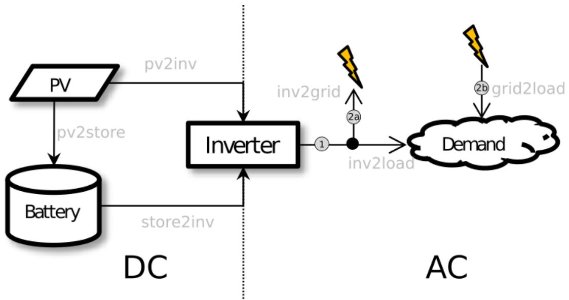
Figure 2.1: Technologies and power flows present in a household with a battery and a PV system [28].
