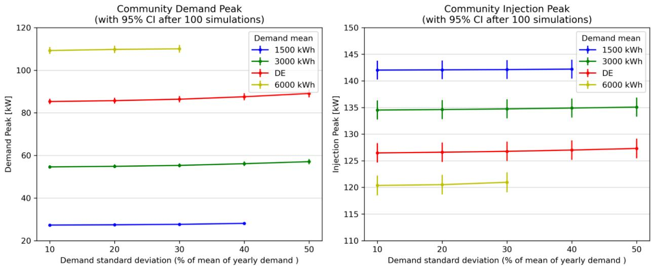
Figure 8.8: Effects of varying the standard deviation of the yearly demand on the community demand peak and injection peak, in the case of energy communities without batteries.
