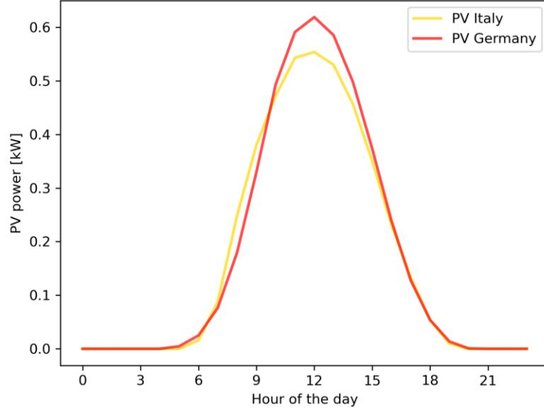
Figure 5.4: Average daily trends of the PV profiles used in the case of the German dataset and of the custom Italian dataset, considering a peak power of 1 kW.
