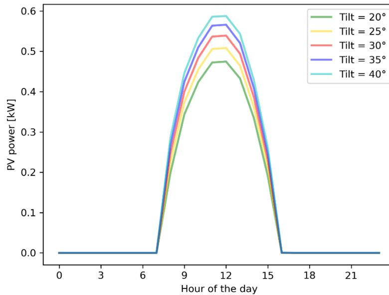
Figure 4.3: Average (over the month of January) daily profiles of PV generation with different inclinations, considering a peak power of 1 kW.
