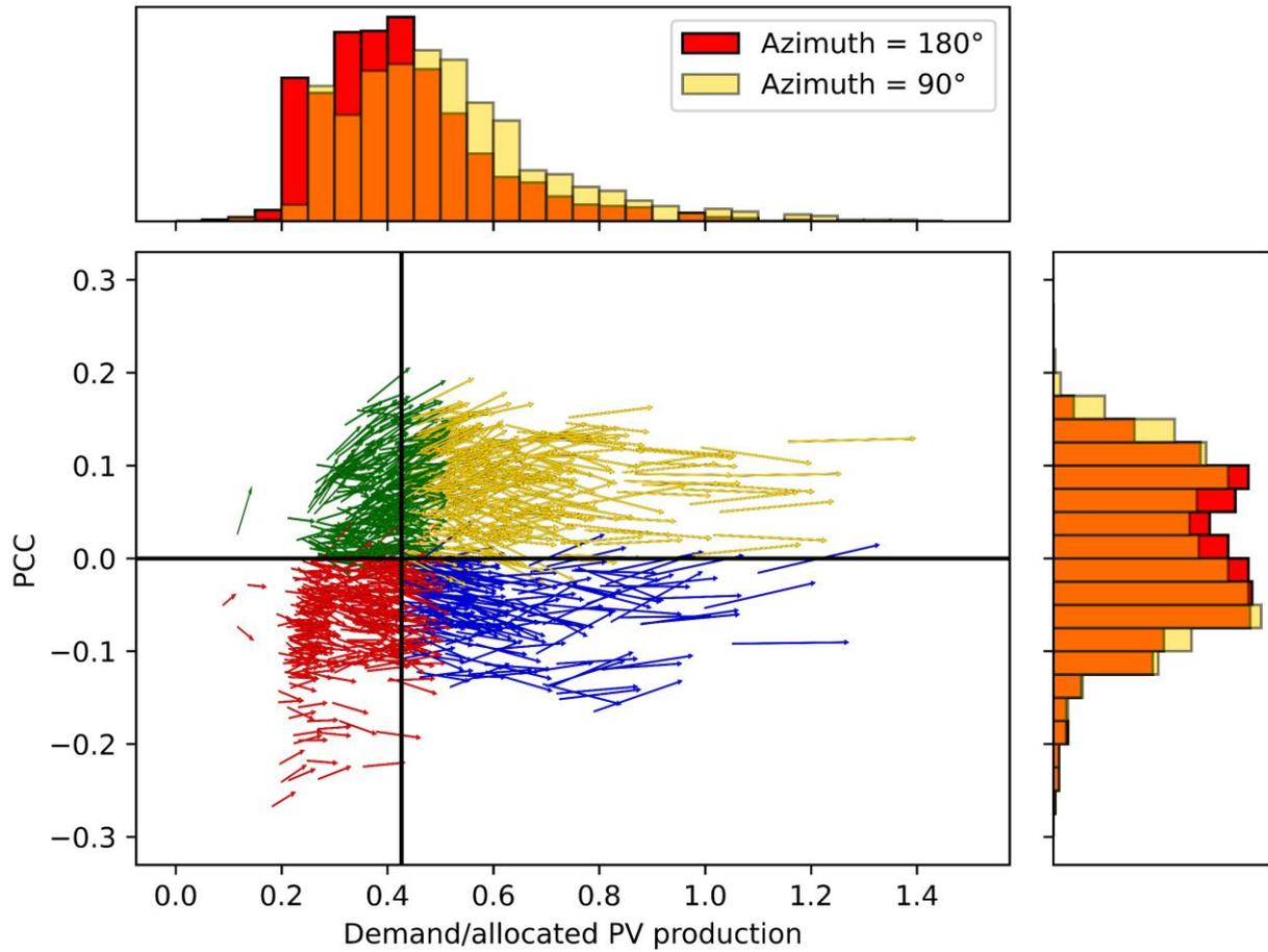
Figure 4.14: Arrow plot (in the PCC-demand plane with normalized demand) and frequency distributions of PCC and normalized demand, comparing South orientation and East orientation.
