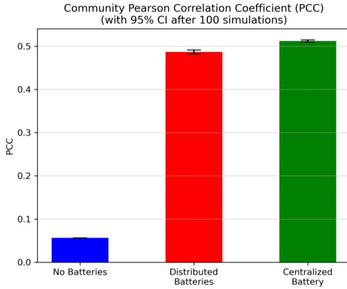
Figure 6.5: overall PCC of the energy community, comparing three cases relative to batteries.
