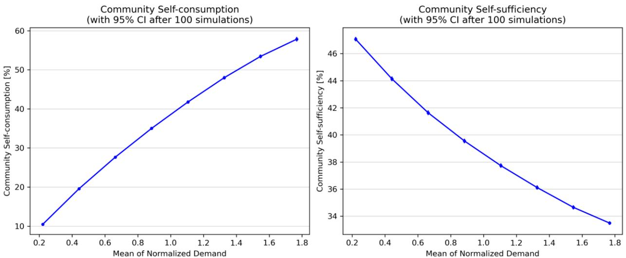
Figure 8.4: Effects of varying the mean of the yearly demand on the community self-consumption and self-sufficiency, in the case of energy communities without batteries.
