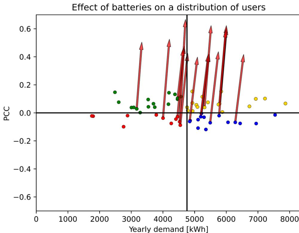
Figure 6.7: Representation of the effect of distributed batteries on users in the PCC-demand plane.
