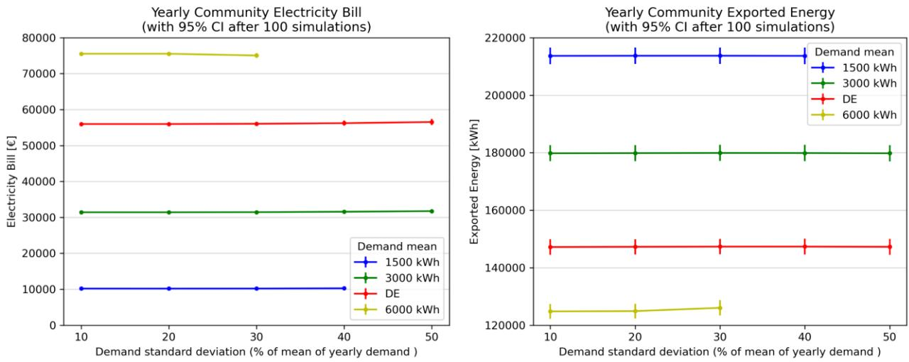
Figure 8.9: Effects of varying the standard deviation of the yearly demand on the yearly electricity bill and energy exported by the community, in the case of energy communities without batteries.
