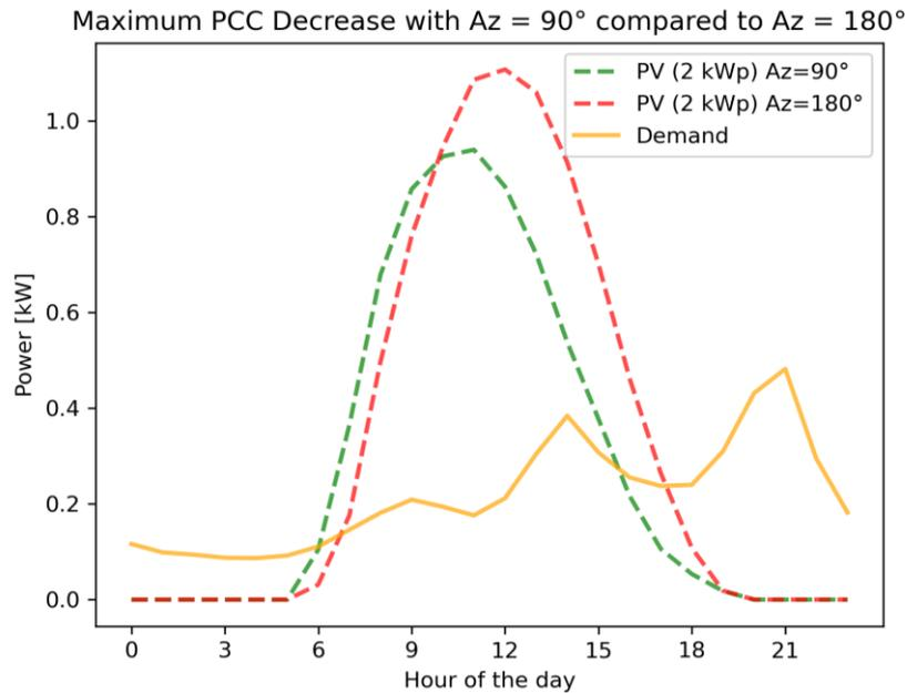
Figure 4.25: Average daily profile of the demand profile whose PCC had the maximum decrease for azimuth angle = 90°, together with the average daily generation profiles of South-oriented and East-oriented PV systems with peak power = 2 kW.
