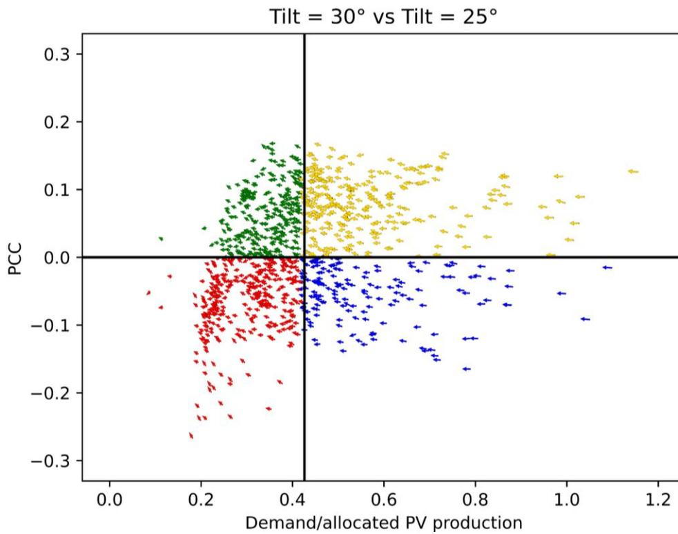
Figure 4.5: Arrow plot in the PCC-demand plane with normalized demand, comparing an inclination of 25° (at the start of the arrows) and an inclination of 30° (at the end of the arrows).
