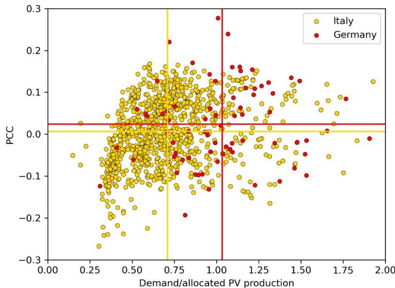
Figure 2.7: Representation on the PCC-demand plane with normalized demand of the German dataset and the Italian dataset, considering an average PV power of 3 kW for the latter.
