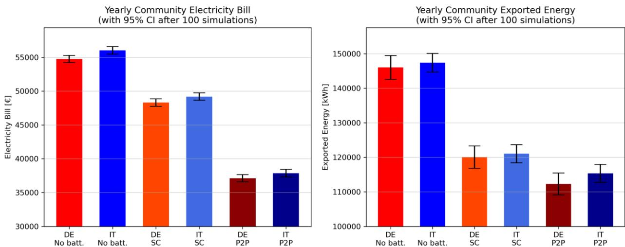
Figure 5.2: Yearly electricity bill and energy exported by the energy community, comparing the German and Italian custom datasets for three subcases relative to batteries.
