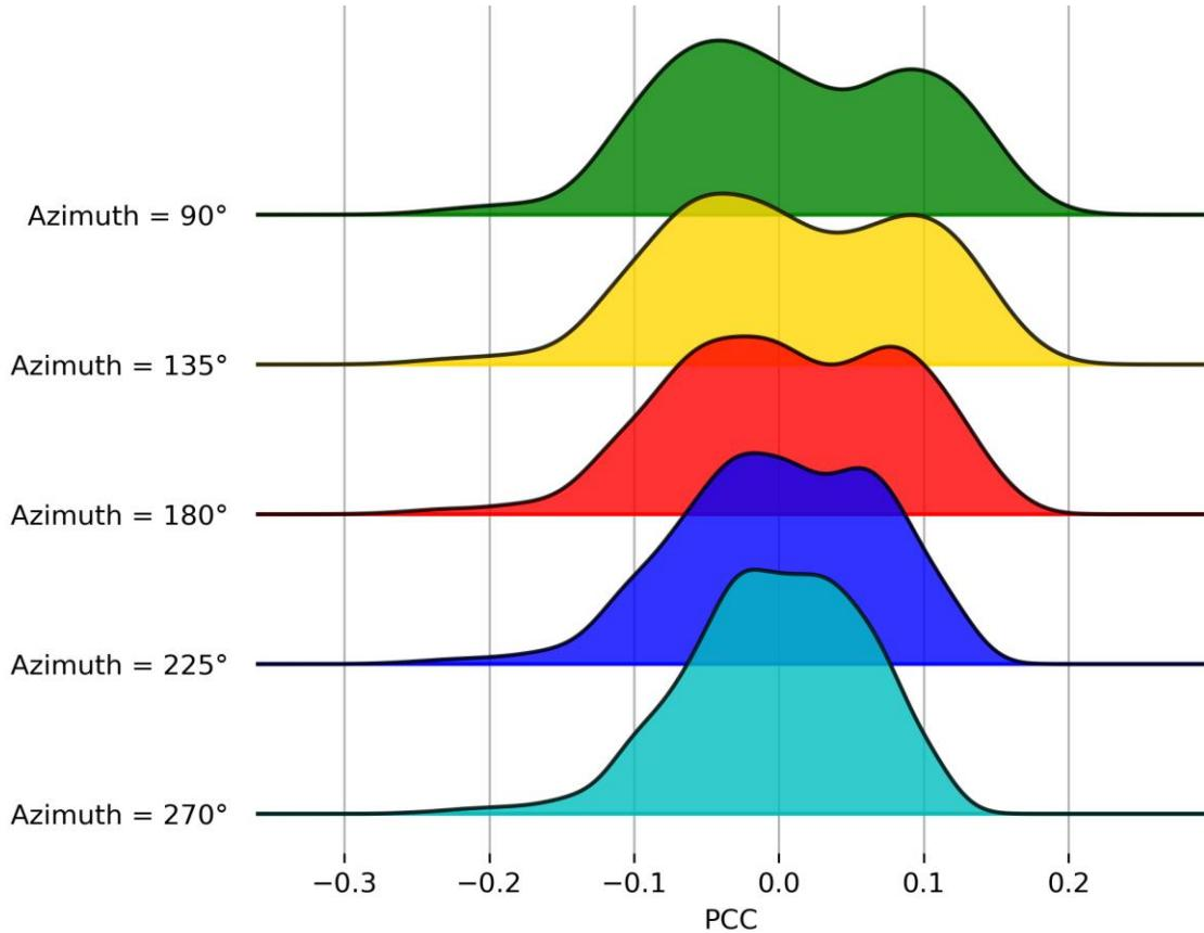
Figure 4.13: Joyplot representing the distributions of PCC corresponding to different orientations of PV systems.
