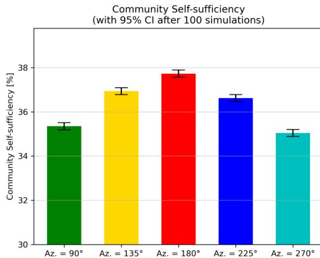
Figure 4.29: Self-sufficiency of an energy community with average PV power equal to 2.06 kW, comparing five different orientations of PV systems.
