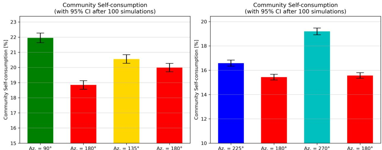
Figure 4.30: Comparisons of community self-consumption for different PV orientations for the four created datasets with demand profiles whose PCC increased with an orientation different from South.
