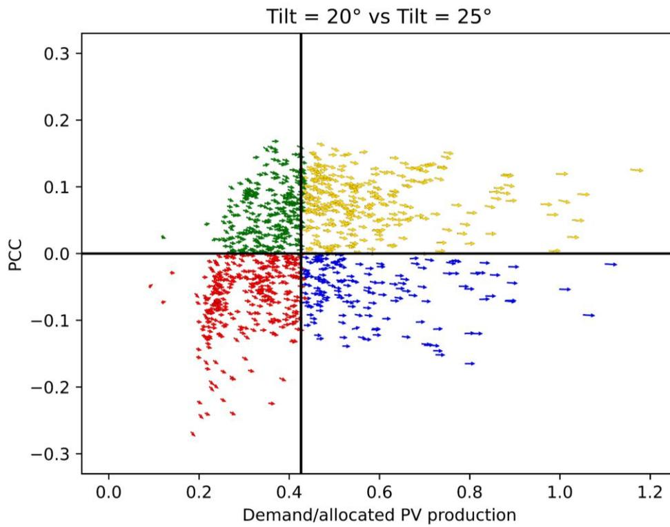
Figure 4.4: Arrow plot in the PCC-demand plane with normalized demand, comparing an inclination of 25° (at the start of the arrows) and an inclination of 20° (at the end of the arrows).
