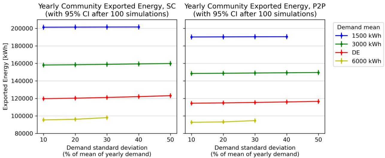
Figure 5.12: Effects of varying the standard deviation of the yearly demand on the energy exported in a year by the community, in the case of energy communities with batteries.
