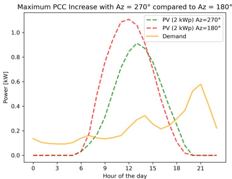
Figure 4.20: Average daily profile of the demand profile whose PCC had the maximum increase for azimuth angle = 270°, together with the average daily generation profiles of South-oriented and West-oriented PV systems with peak power = 2 kW.
