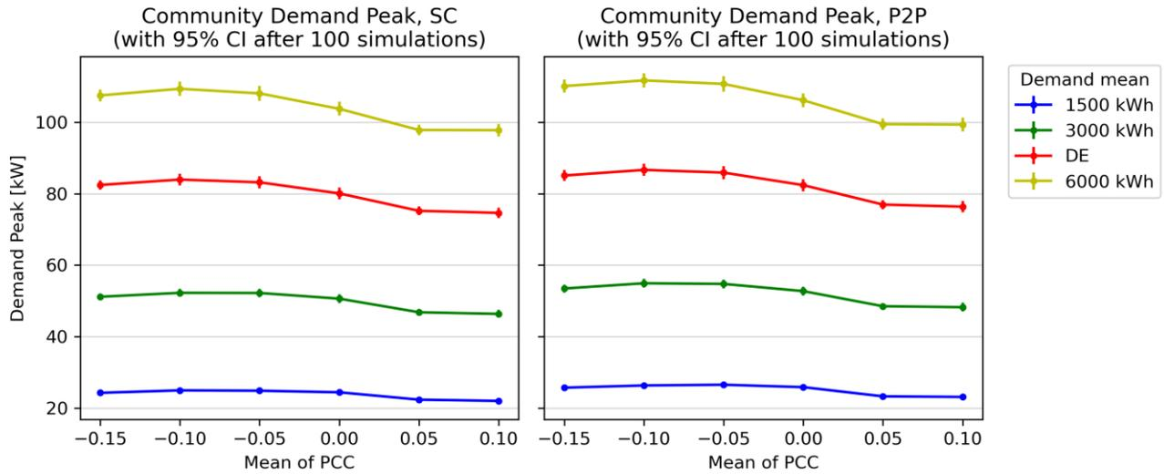
Figure 5.19: Effects of varying the mean of the PCC on the community demand peak, in the case of energy communities with batteries.
