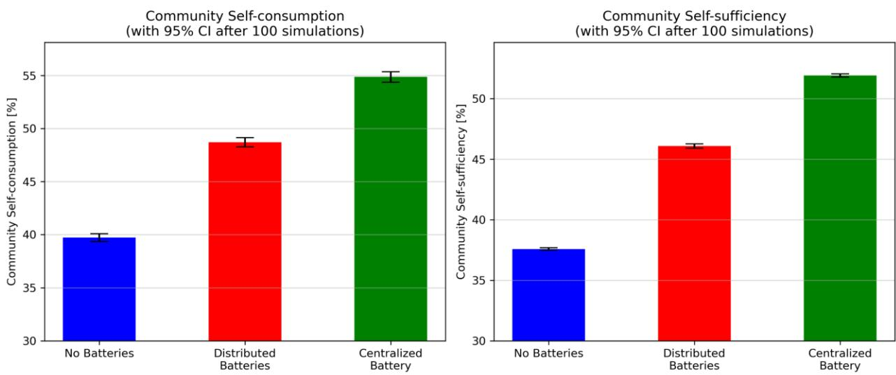
Figure 6.1: Self-sufficiency and self-consumption of the energy community, comparing three cases relative to batteries.
