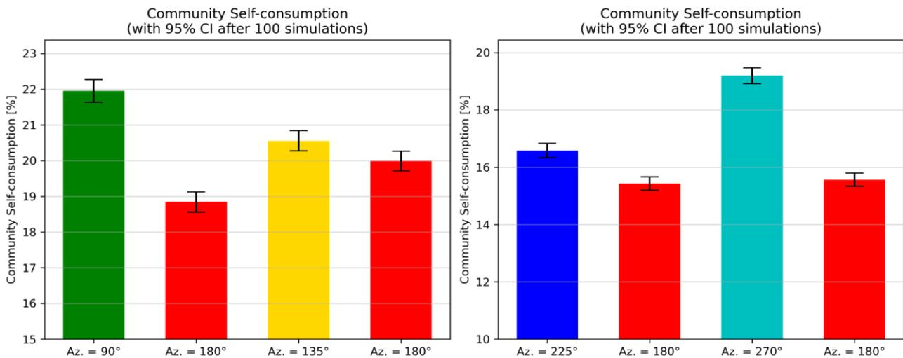
Figure 4.30: Comparisons of community self-consumption for different PV orientations for the four created datasets with demand profiles whose PCC increased with an orientation different from South.
