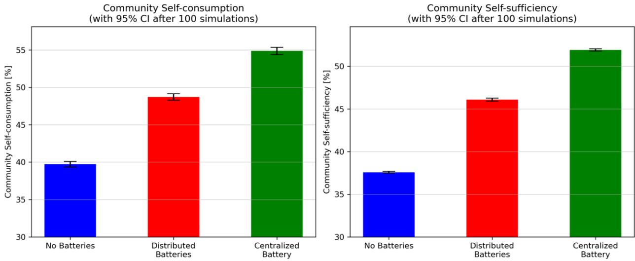
Figure 6.1: Self-sufficiency and self-consumption of the energy community, comparing three cases relative to batteries.
