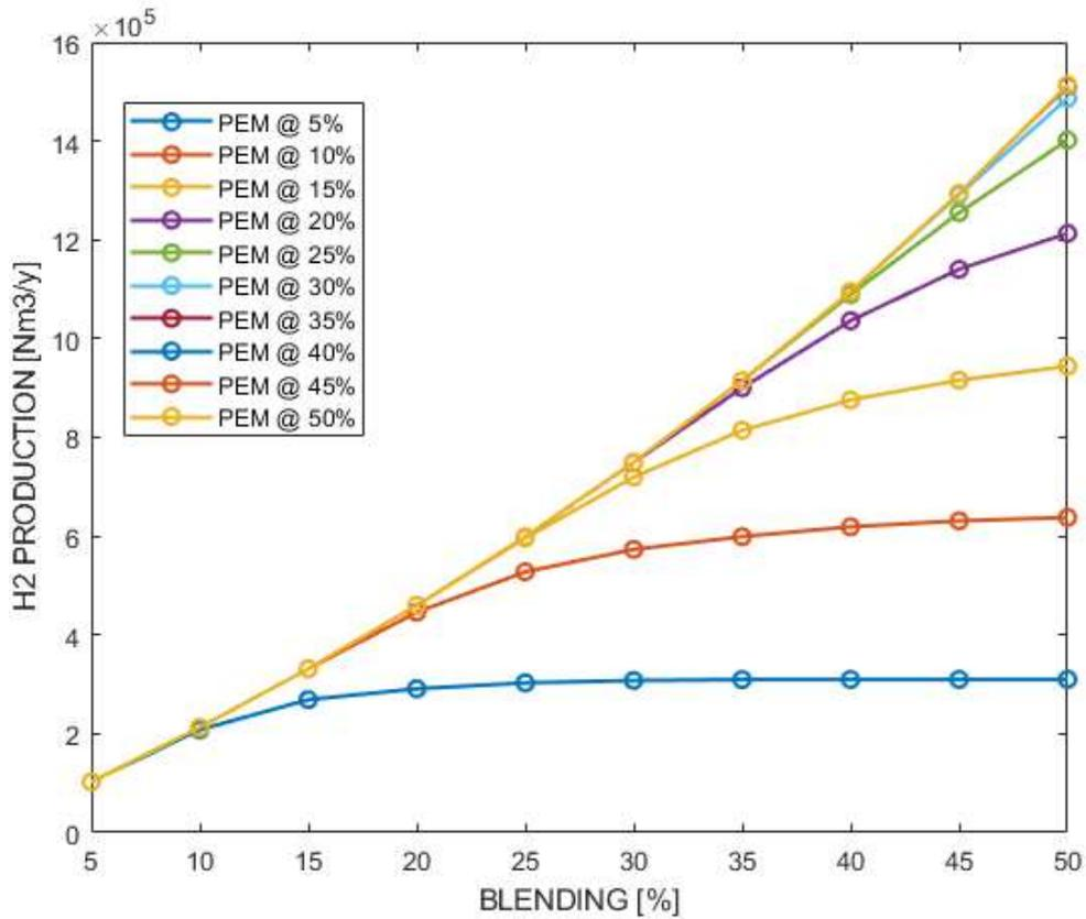
Figure 20. PEM electrolyzers behaviour at every blending.
