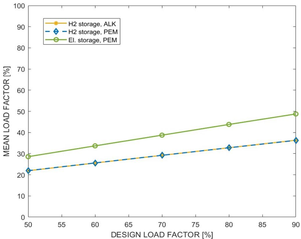
Figure 15. Mean operating load factor by varying the design load factor.
