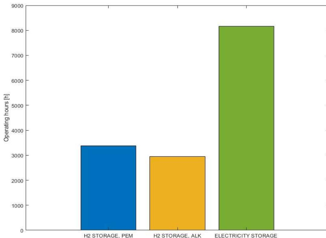
Figure 12. Electrolyzer's operating hours in the reference scenarios.
