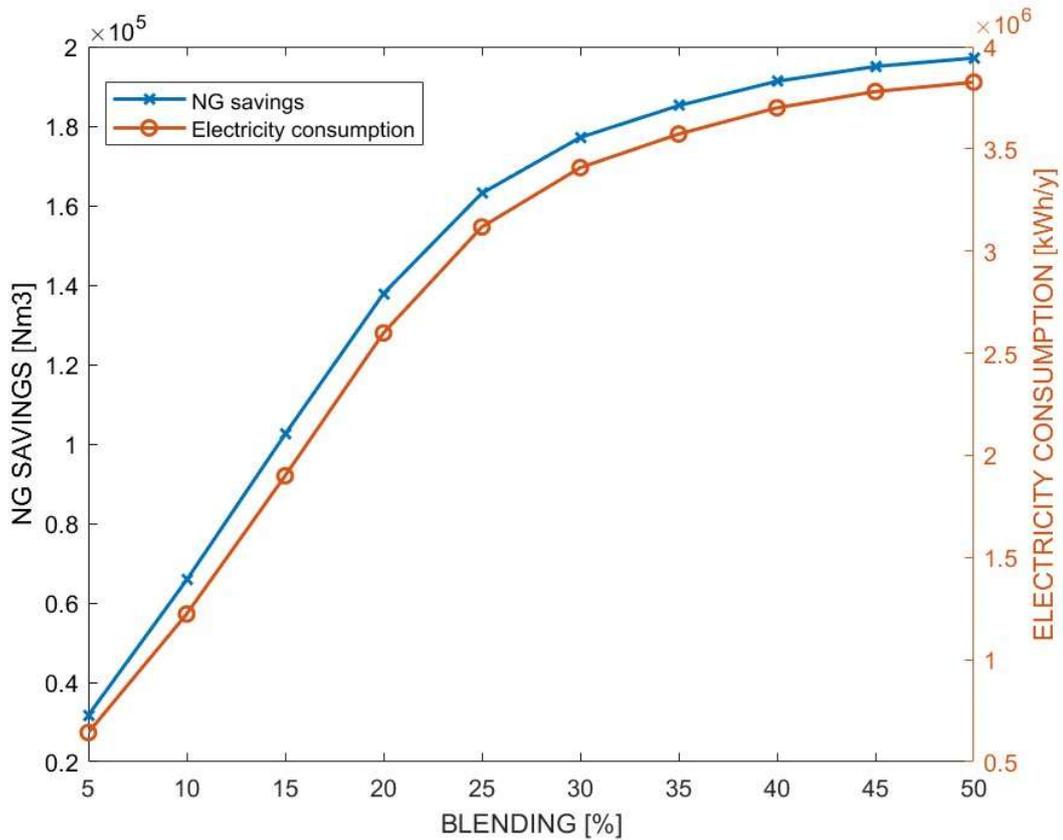
Figure 19. Natural gas savings and electricity consumption at variable blending.
