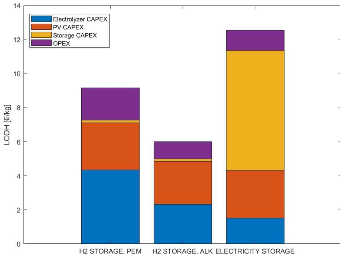
Figure 23. LCOH breakdown in the main scenarios.
