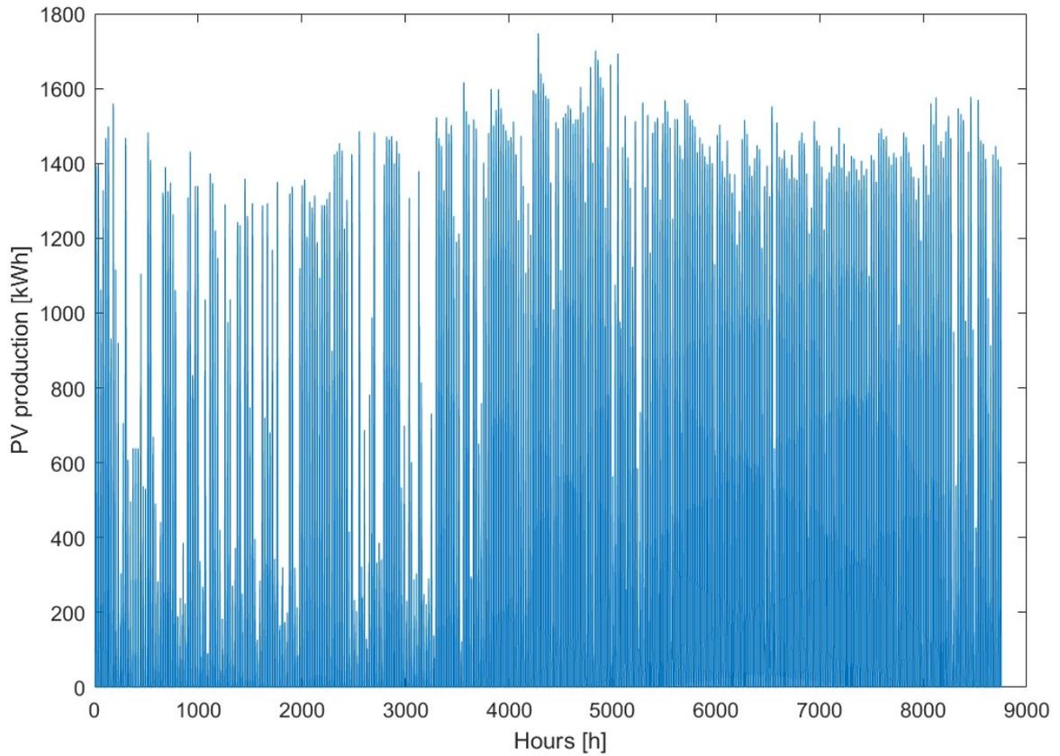
Figure 10. Photovoltaic production hour profile.
