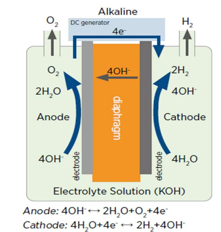
Figure 1. Alkaline electrolytic cell scheme [8].
