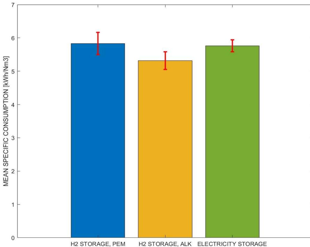
Figure 14. Mean Specific Consumptions and standard deviations (red lines).
