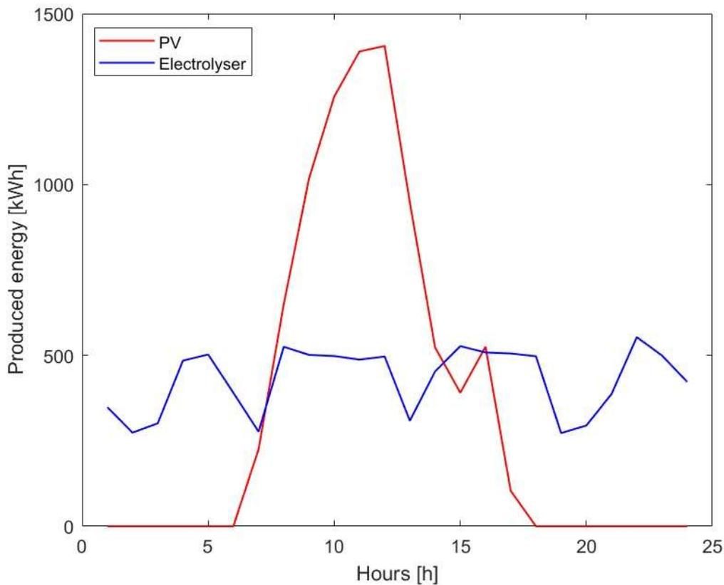
Figure 11. Comparison between photovoltaic and electrolyzer energy profile in a day.
