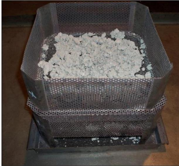
Figura 12 - Miscela post carbolite (solo aggregati e filler)
