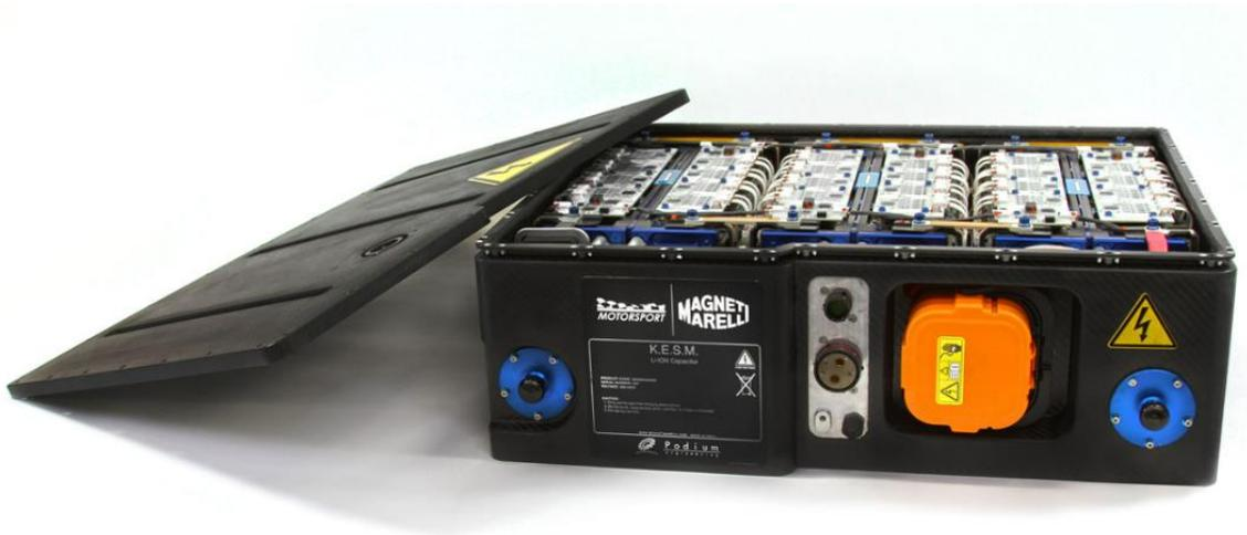
Figure 6 - High Voltage Battery Pack
