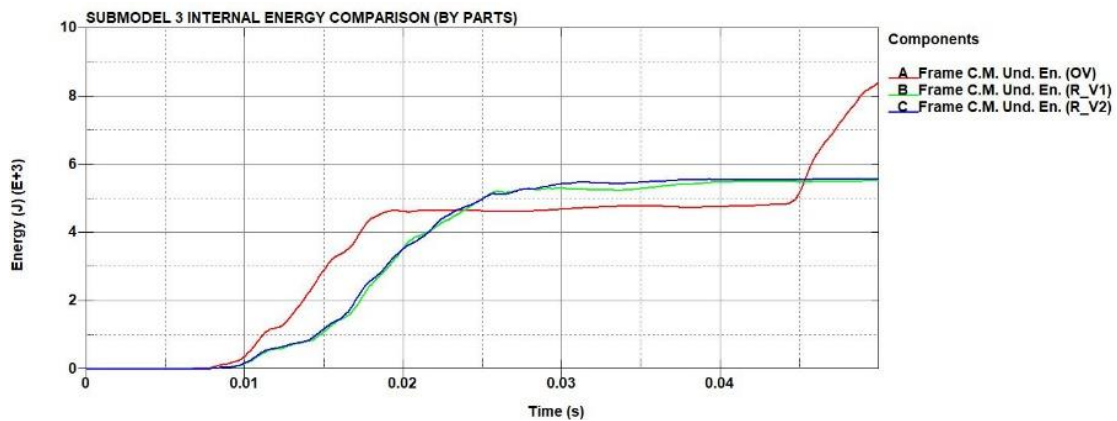
Figure 168 - Submodel 3 remeshing (without transitioning zone) "Frame cross member under engine" internal energy
