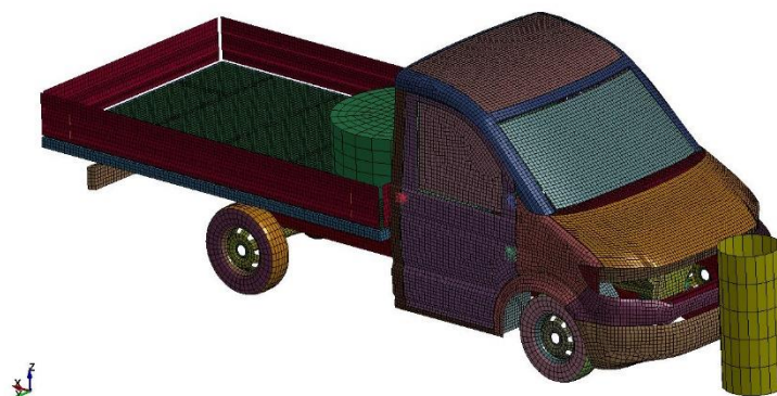
Figure 30 - Vehicle impact on bollard
