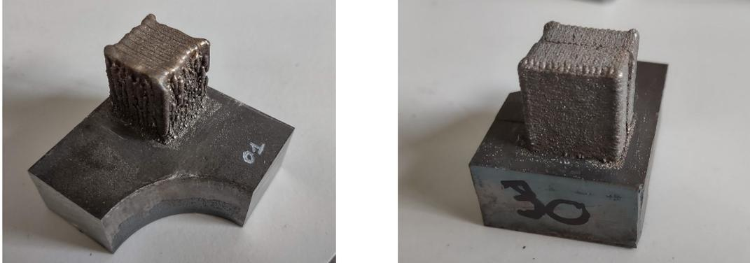
*Figure 28: Sample with poor exterior finish (left) and good exterior finish (right) - (Mariani 2022)*
