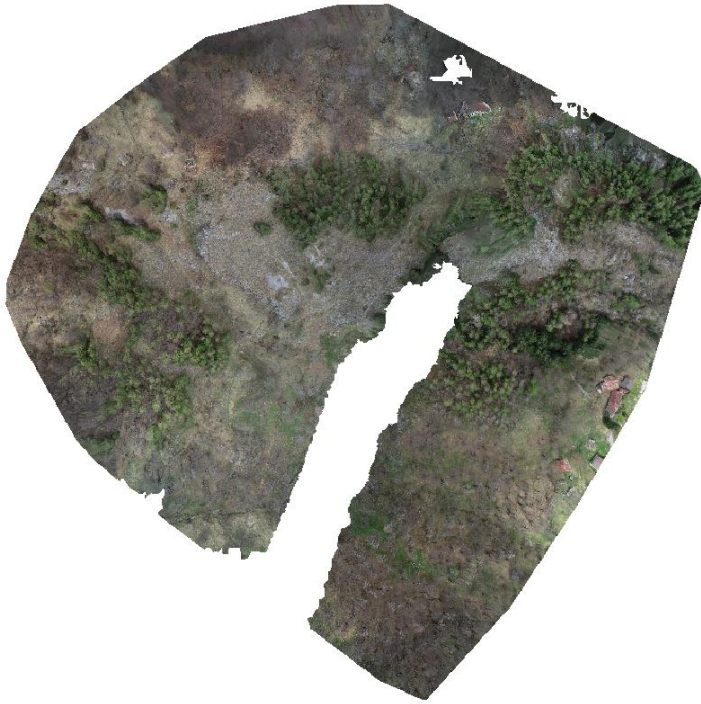
Figure 14: First 150 photos to create an orthophoto of Bossea cave.
