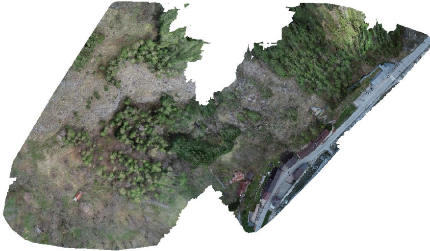
Figure 18: Last 150 photos to create an orthophoto of Bossea cave.
