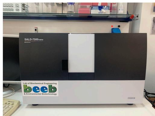
*Figure 3.7. SALD-7500nano by Shimadzu for Dynamic Light Scattering.*
