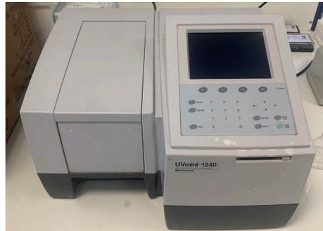
Figure 3.13. Spectrophotometer UVmini-1240 by Shimadzu.
