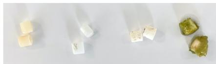
Figure 4.4. Differences between virgin TPS pellets, exposed and cleaned pellets, and pellets with biofilm after 90 days exposure (outdoor pelagic).
