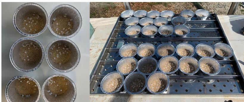
Figure 3.2. Coastal setup: metallic cups filled with sand and plastic pellets.
