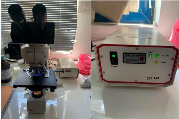
*Figure 3.6. Fluorescence microscope.*
