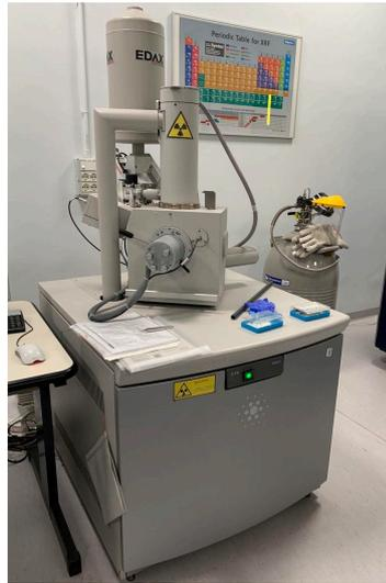
*Figure 3.11. Scanning electron microscope (FEI Inspect S50).*
