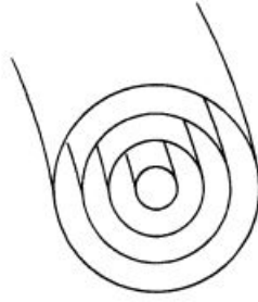
Figure 1: Magnetic surfaces forming nested toroids [5].
