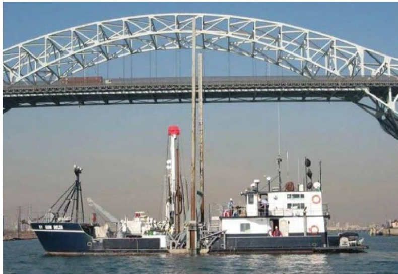
Figure 5 – Gregg Quinn Delta ship with spuds
