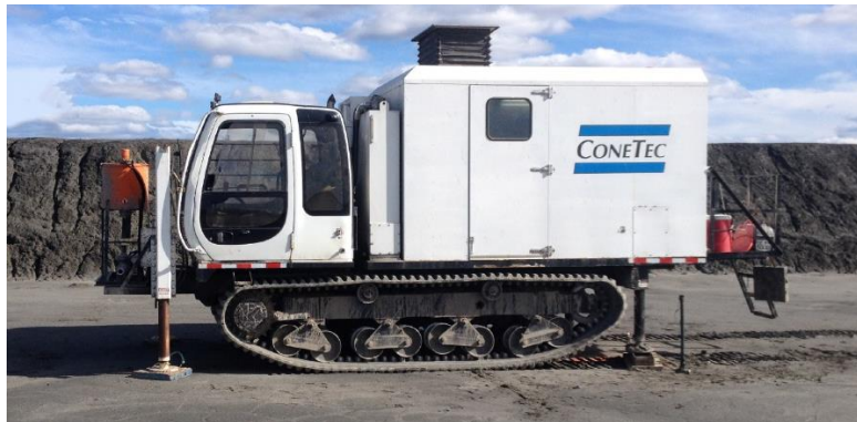
Figure 3 – CPT on track operated by ConeTec
