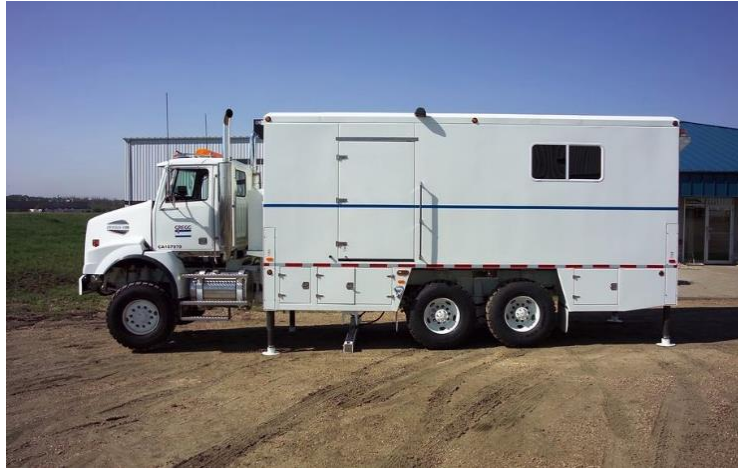
Figure 2 – CPT truck operated by the Gregg
