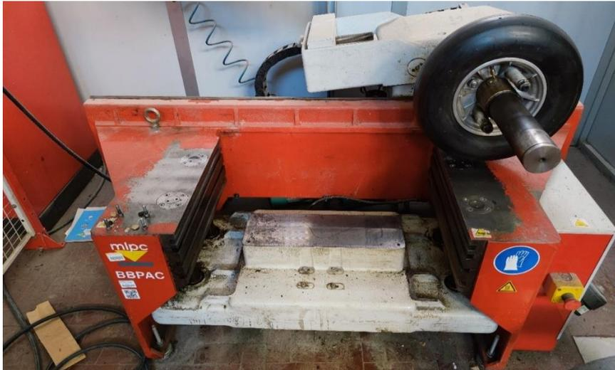
Figure 36 The roller compactor without the auxiliary elements
