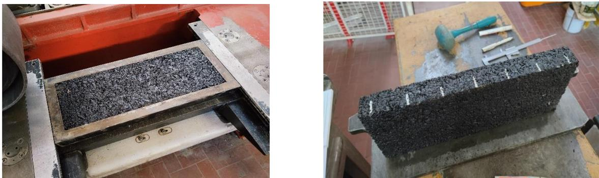
Figure 38 finishing of the slab compaction and removing from the mould
