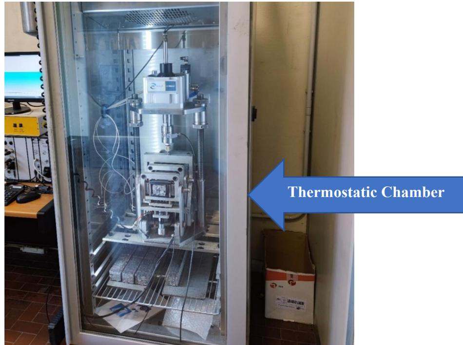
Figure 49 Four point bending machine with thermostatic chamber
