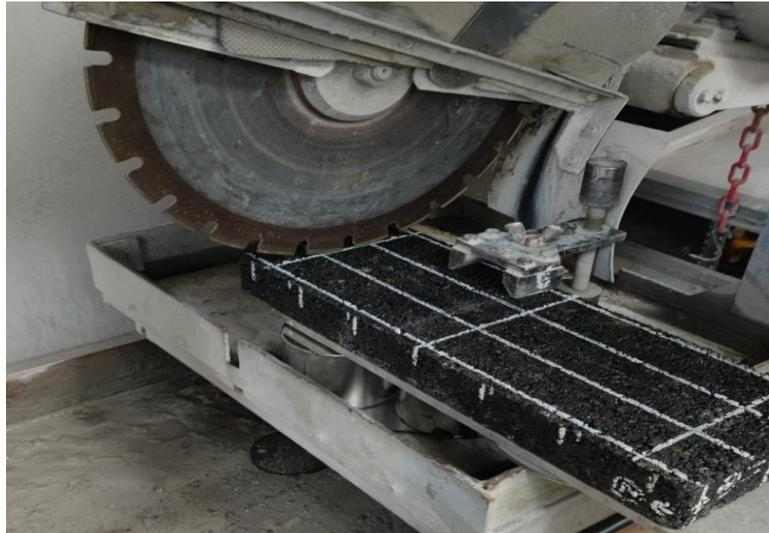
*Figure 40 Slab sawing*
