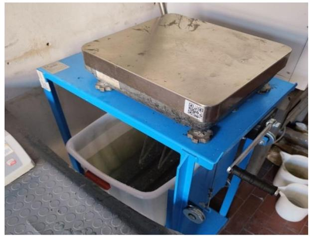
Figure 46 The water bath and the balance
