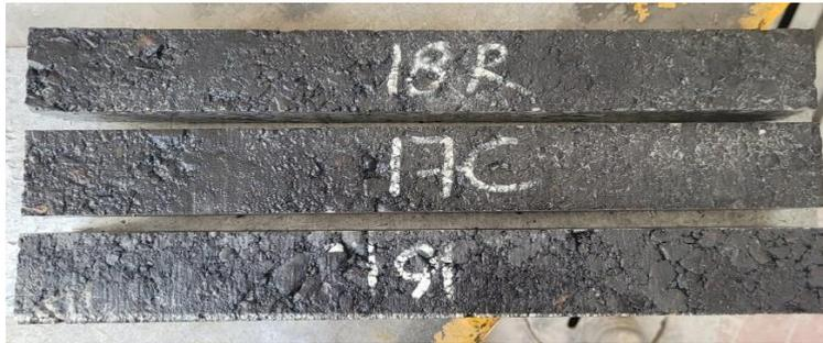
Figure 41 Four point bending beams
