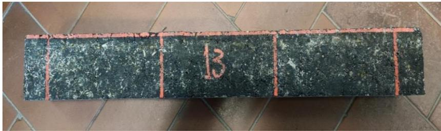
Figure 42 4PB measurement points
