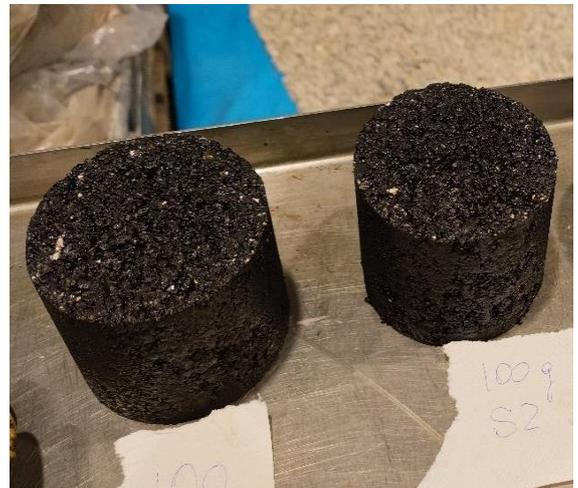
Figure 33 Typical gyratory molds and samples
