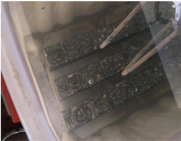
Figure 45 The 4PB beams inside the water bath
