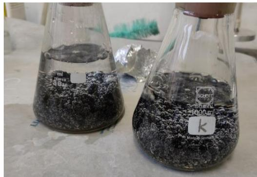
*Figure 26 Asphalt particles inside the pycnometer*
