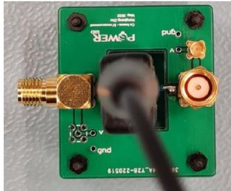
**Figure 3.3:** PCB with the Current Probe already connected
