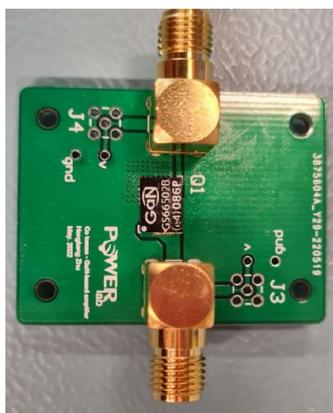
**Figure 3.2:** My class A amplifier, GS66502B: a GaN on SI power MOSFET
