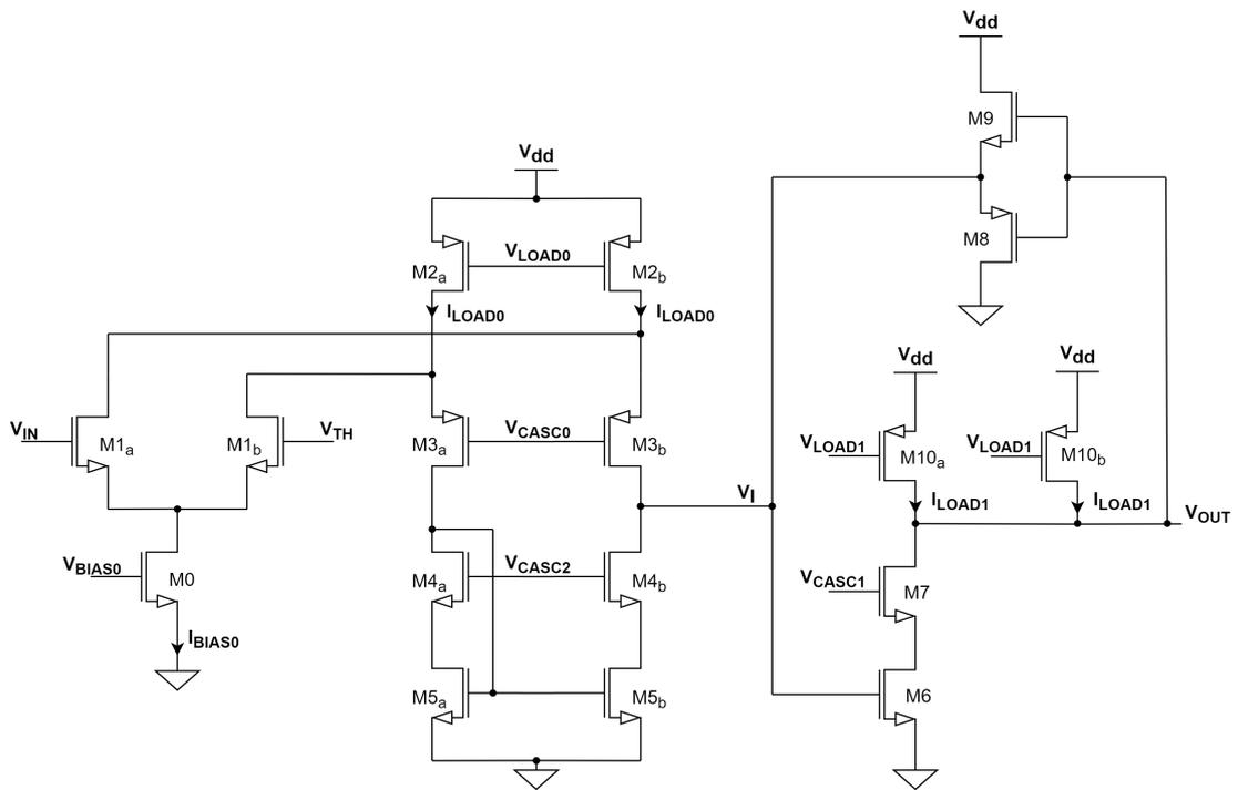
Figure 3.4: Schematic of current based discriminator.
