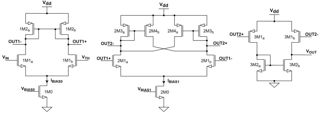
**Figure 3.6:** Schematic of cross-coupled positive feedback discriminator.
