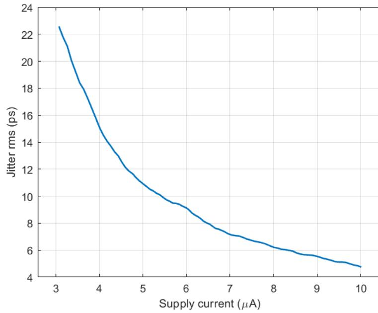
**Figure 4.9:** Jitter vs supply current for 10 ke<sup>-</sup> input (CURR).
