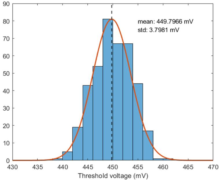
**Figure 4.4:** Threshold voltage distribution (CURR).
