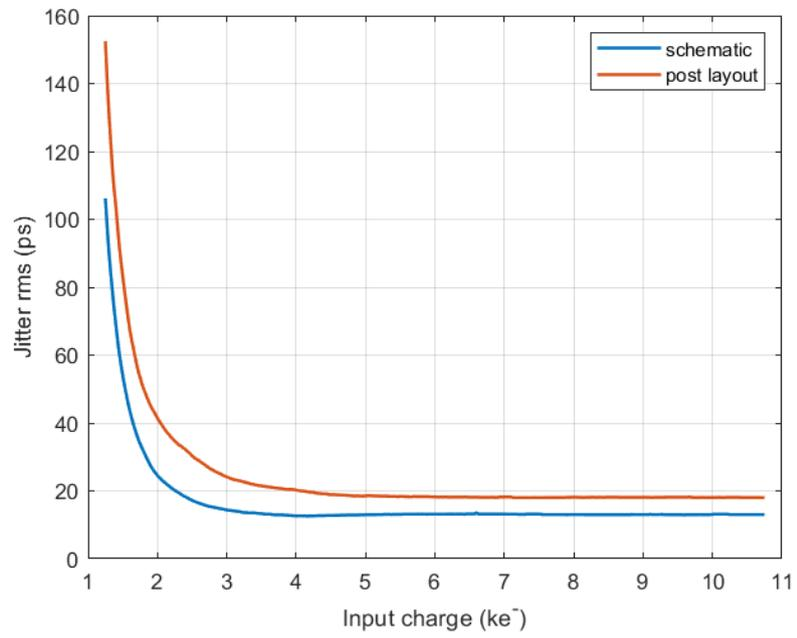
**Figure 4.11:** Post-layout simulation (CURR).
