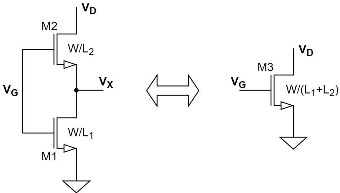
**Figure A.1:** Representation of the equivalence between two stacked transistors and a single transistor.
