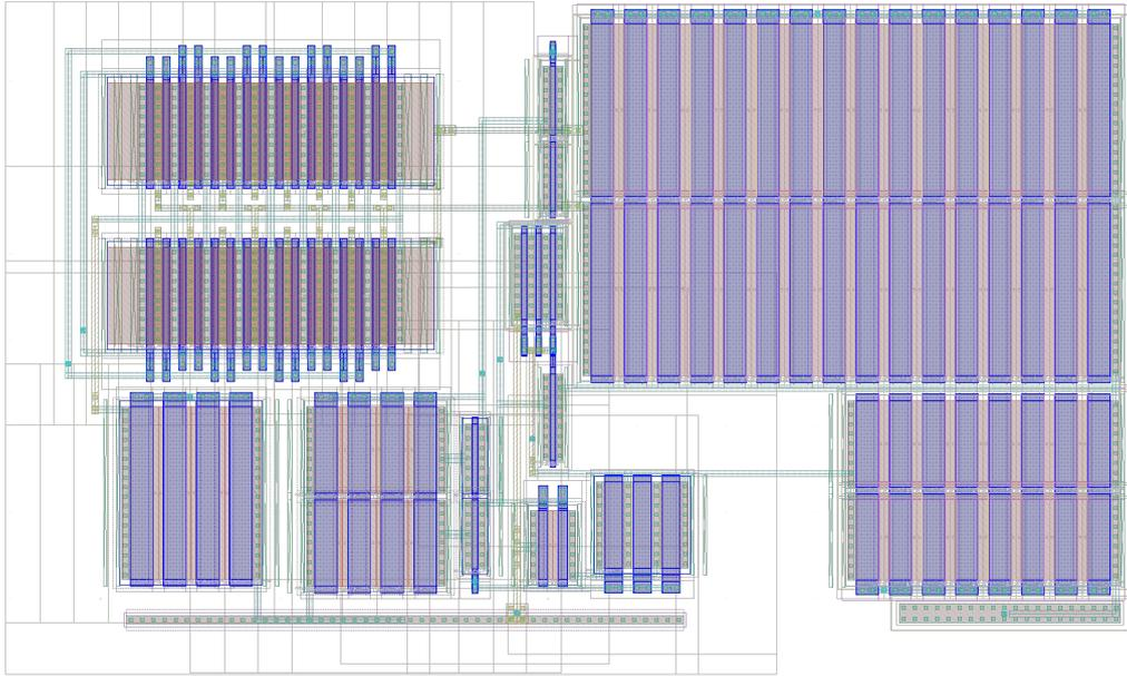
**Figure 3.5:** Layout of current based discriminator ( $11.98 \mu\text{m} \times 7.26 \mu\text{m}$ ).
