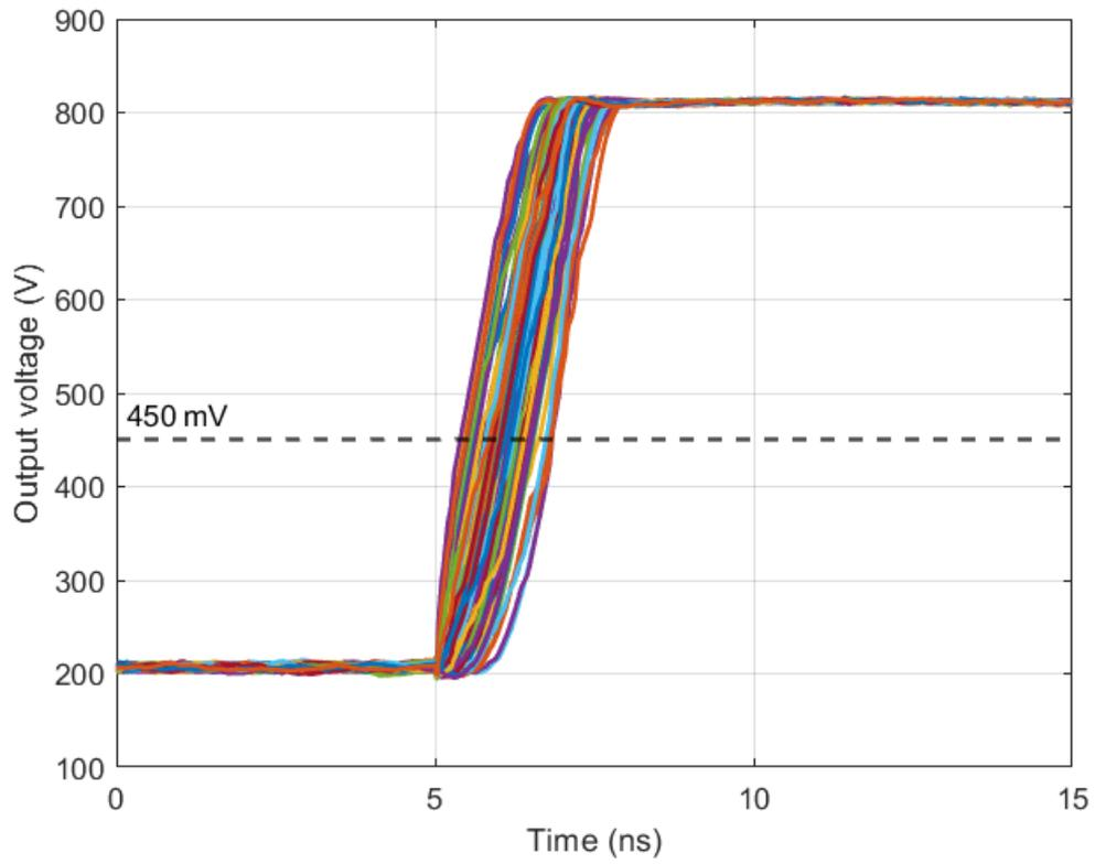
**Figure 4.5:** Jitter simulation output voltage at  $10 \text{ ke}^-$  (CURR).
