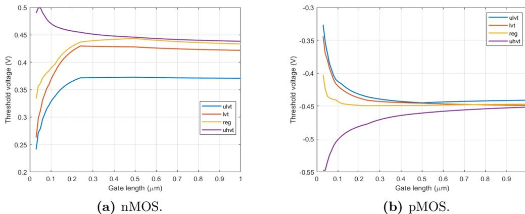
**Figure 2.4:** Threshold voltage variation with gate length.
