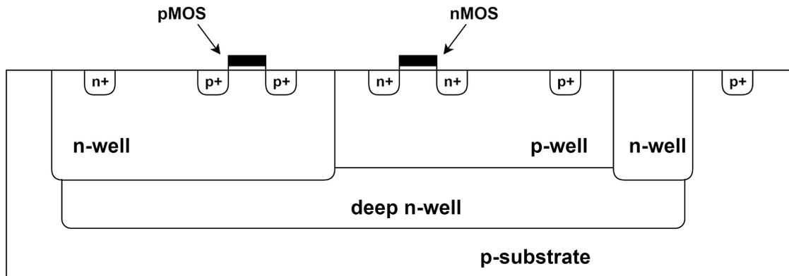
Figure 3.3: Triple-well structure.
