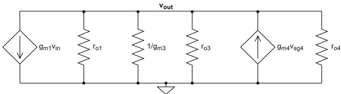
(b) Small signal equivalent circuit.
