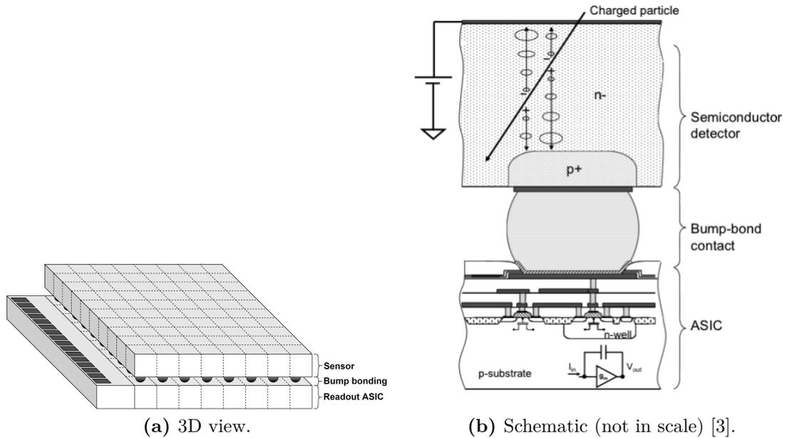
**Figure 1.2:** Hybrid pixel detector.
