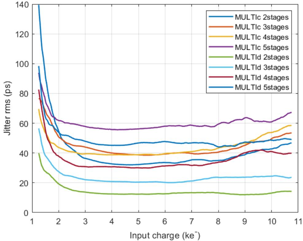
**Figure 4.6:** Jitter comparison for MULTI topology.
