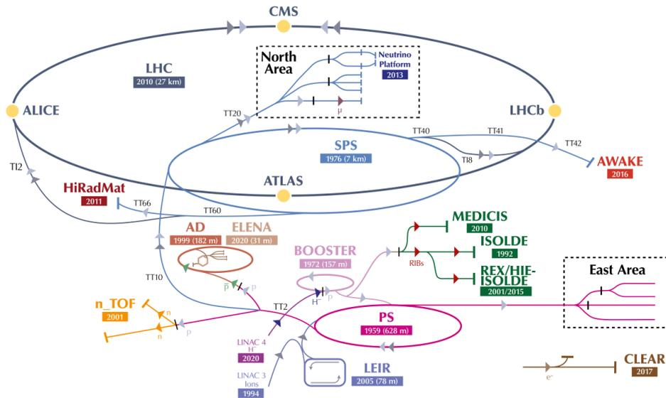
Figure 1.1: CERN accelerator complex [1].
