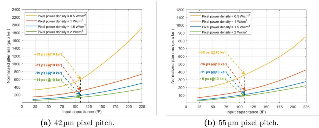
**Figure 4.12:** Jitter at the output of CSA and discriminator chain versus the input capacitance.
