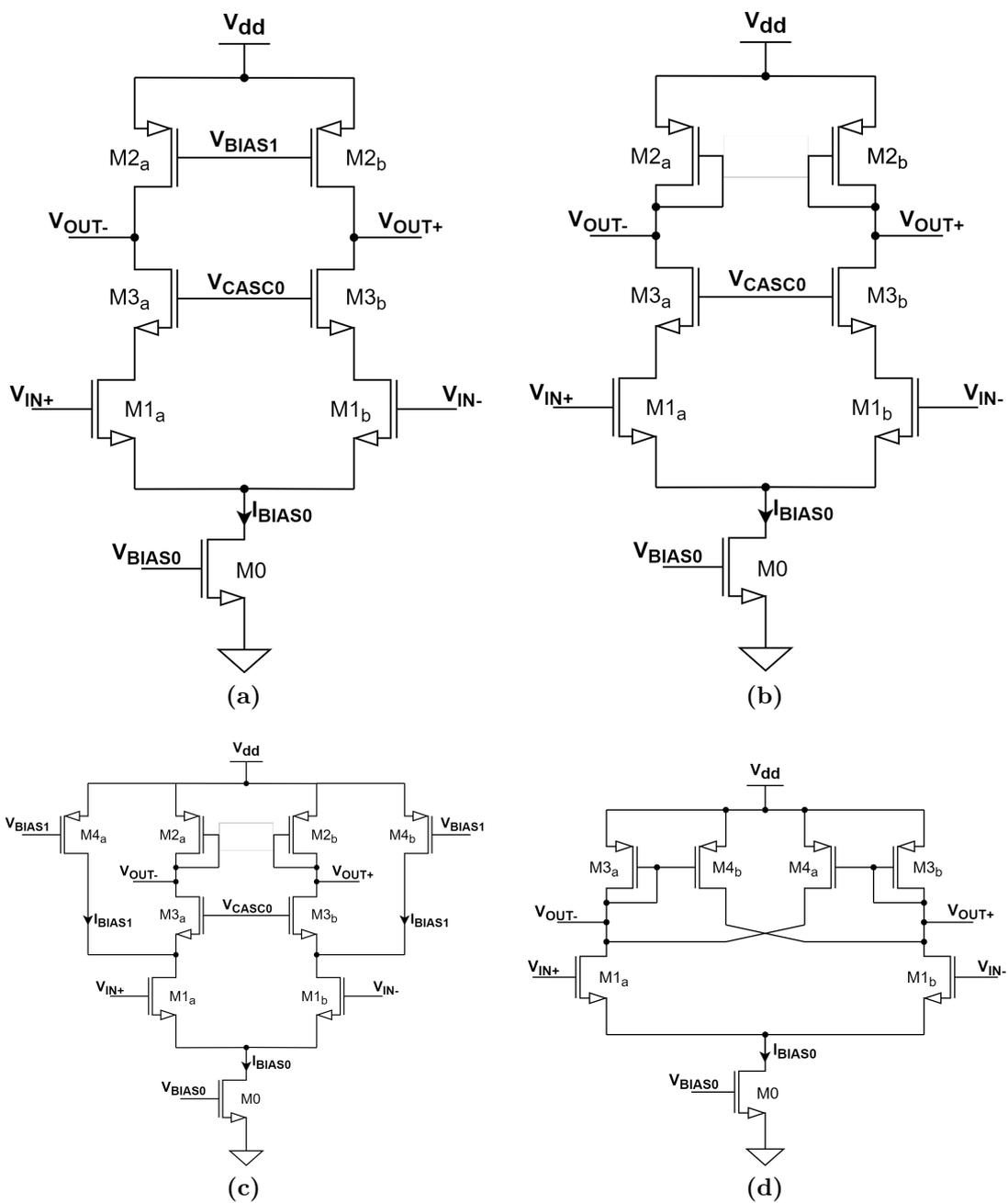
Figure 3.9: Topology options for fully differential OTA.
