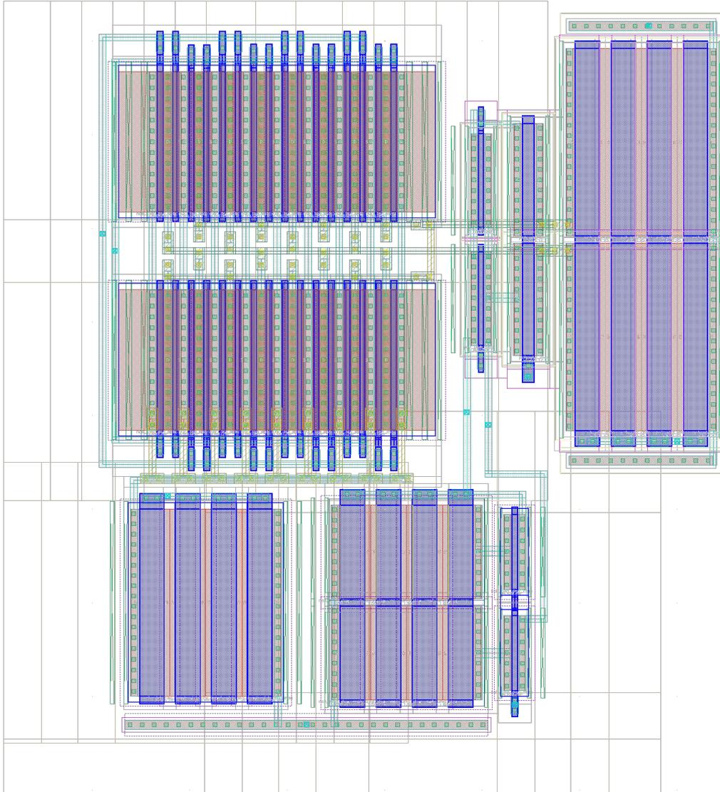
**Figure 3.2:** Layout of clamped folded cascode discriminator ( $6.46 \mu\text{m} \times 7.72 \mu\text{m}$ ).
