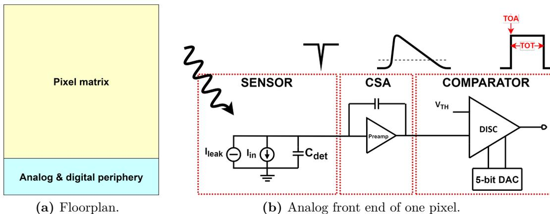
**Figure 1.3:** Concept of PicoPix chip and its analog front end.
