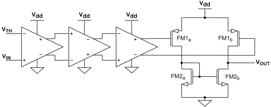
**Figure 3.8:** Schematic of multi-low-gain-stage discriminator.
