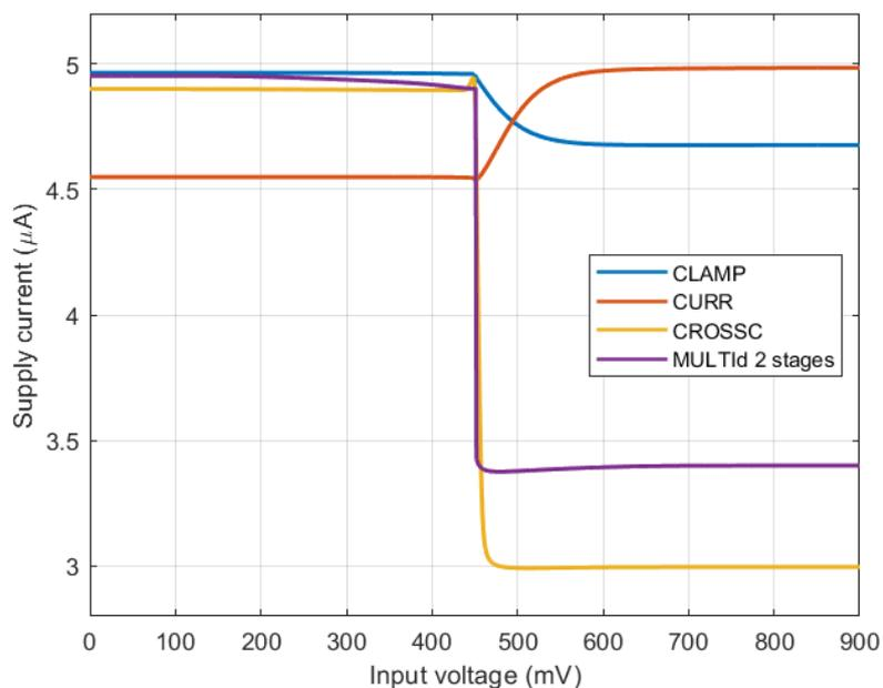
**Figure 4.8:** DC sweep current comparison.
