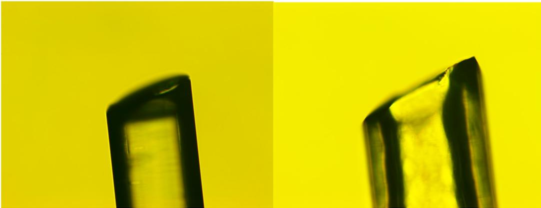
*Figure 38: pictures taken with the optical microscope of fiber (left) and hollow fiber (right) samples cleaved by imposing a rotation of 45° to the right clamp.*
