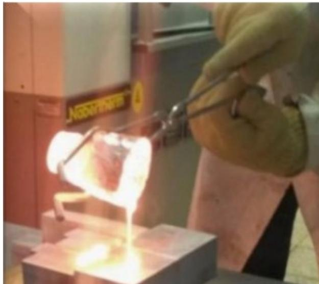
*Figure 15: Cast of the melt*
