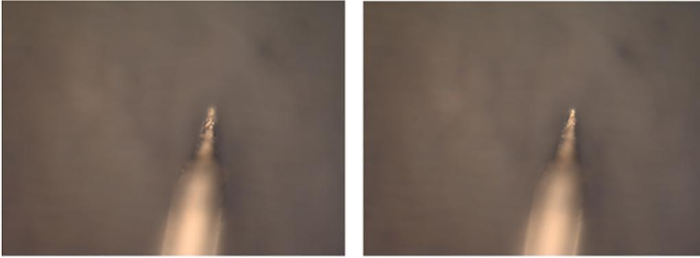
**Figure 4.12:** Optical microscope image of PtBlack coated  $\mu$ electrodes.
