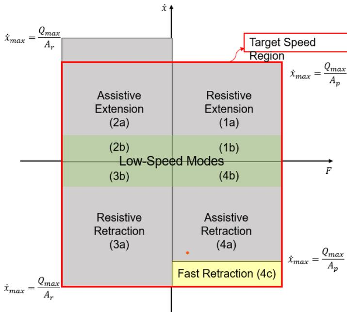
Figure 3.4: Working modes algorithm
