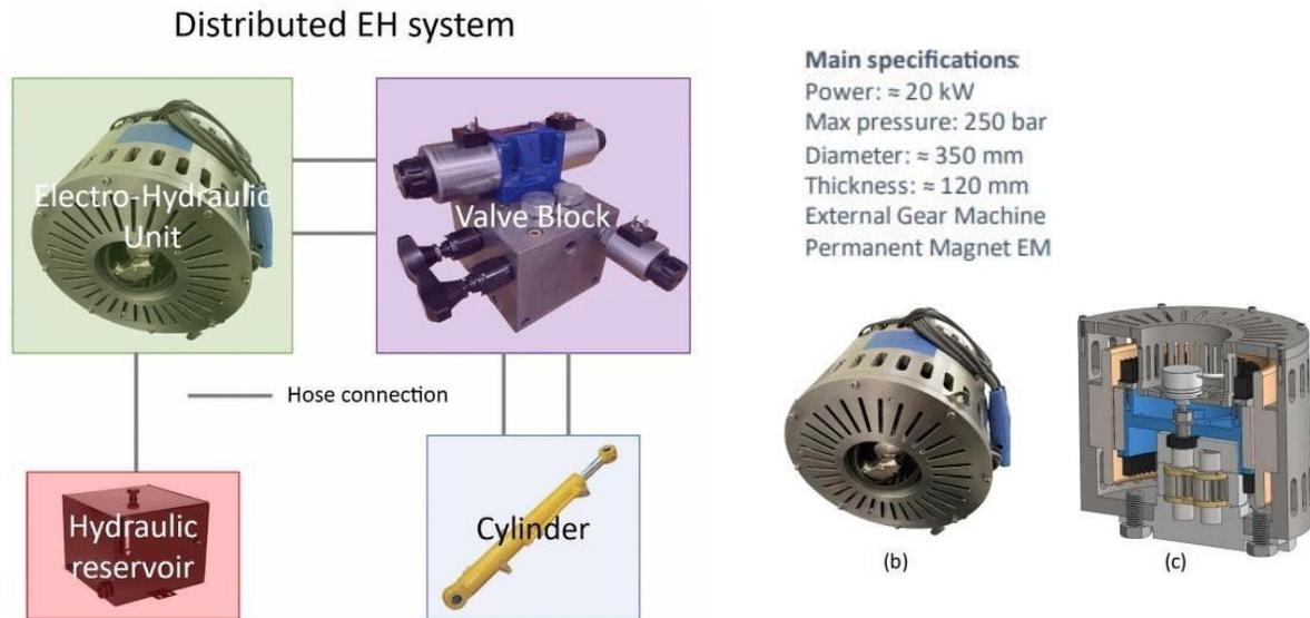
Figure 3.2: Distributed Electro-Hydraulic system and EHU
