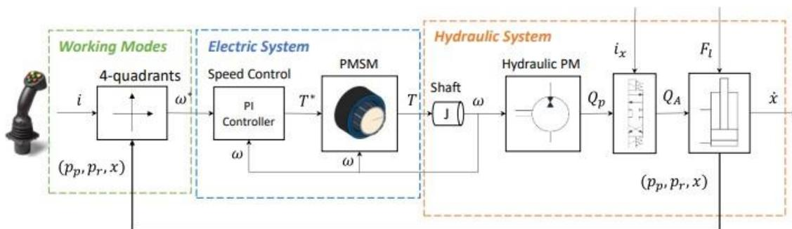
Figure 3.6: Control algorithm of Electro-hydraulic system
