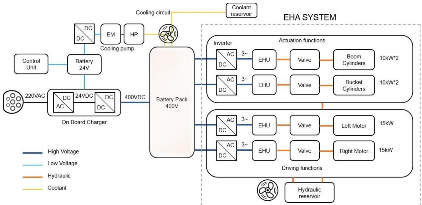
Figure 3.1: Overall schematic of electrified skid steer
