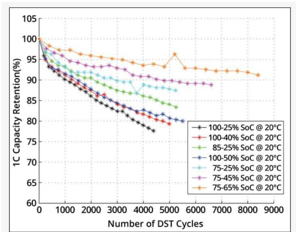
Figure 5.6: State of charge for different DST cycles at 20 degree
