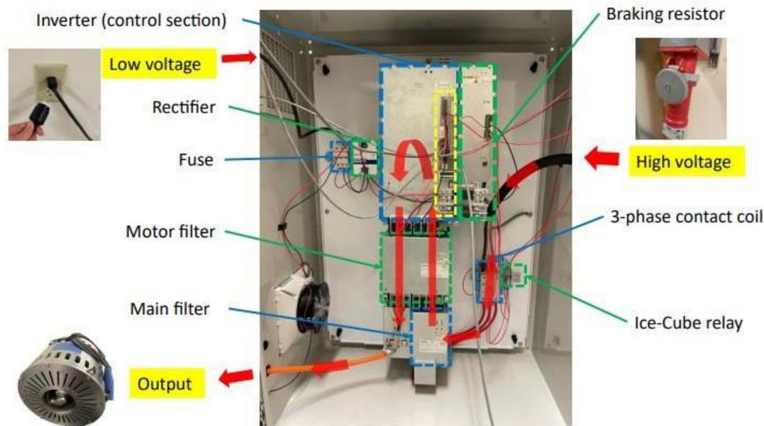
Figure 3.5: Power electronic setup
