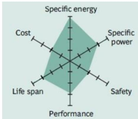
Figure 5.11: Lithium Nickel Cobalt Aluminum Oxide (NCA) characteristics
