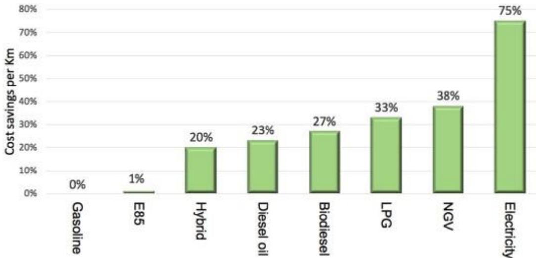
Figure 2.4: Cost saving comparison between different fuel type
