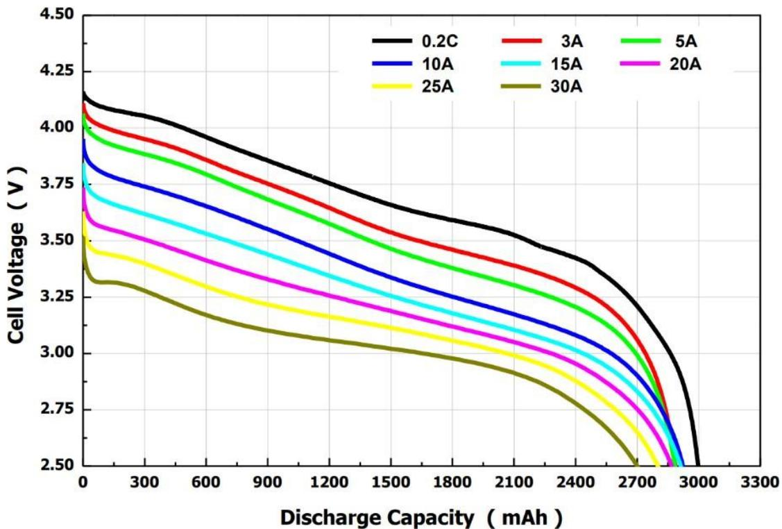
Figure 5.2: Discharge rating of lithium-ion cell
