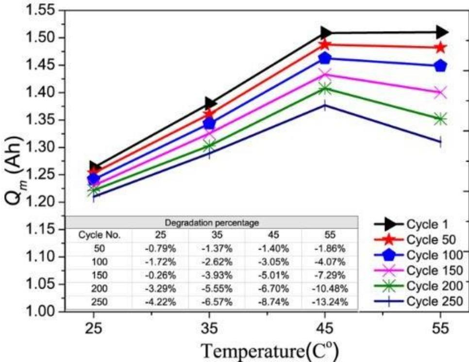
Figure 5.5: Degradation percentage at different Temp ranges
