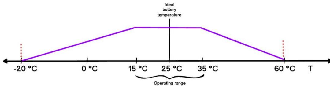
Figure 5.3: Temperature ranges for Li-ion cells
