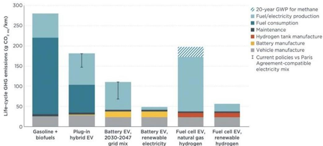
Life-cycle GHG emissions of SUV segment gasoline ICEVs, PHEVs, BEVs, and FCEVs projected to be registered in the United States in 2030. A graph from the ICCT report: A global comparison of the life-cycle greenhouse gas emissions of combustion engine and electric passenger cars
