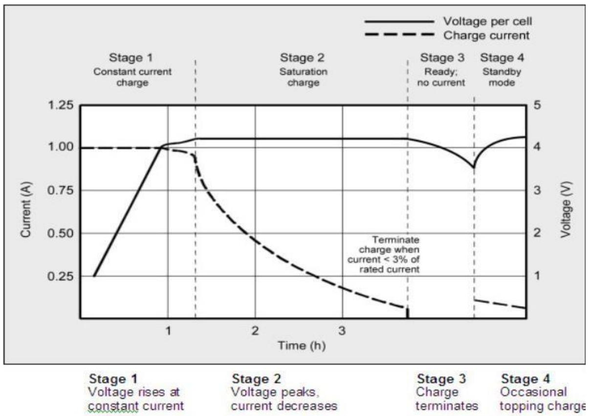
Figure 4.1: Constant Current and Constant Voltage
