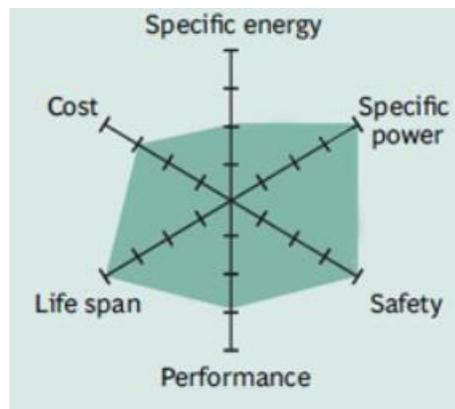
Figure 5.10: Lithium Iron Phosphate characteristics
