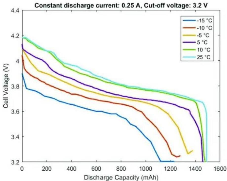
Figure 5.4: Discharging rate w.r.t to different temperature ranges
