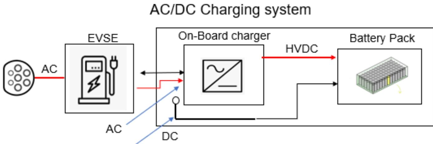
Figure 4.3: Schematic of AC/DC charging system
