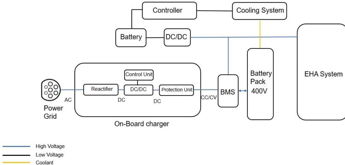
Figure 4.4: On-Board charge schematic
