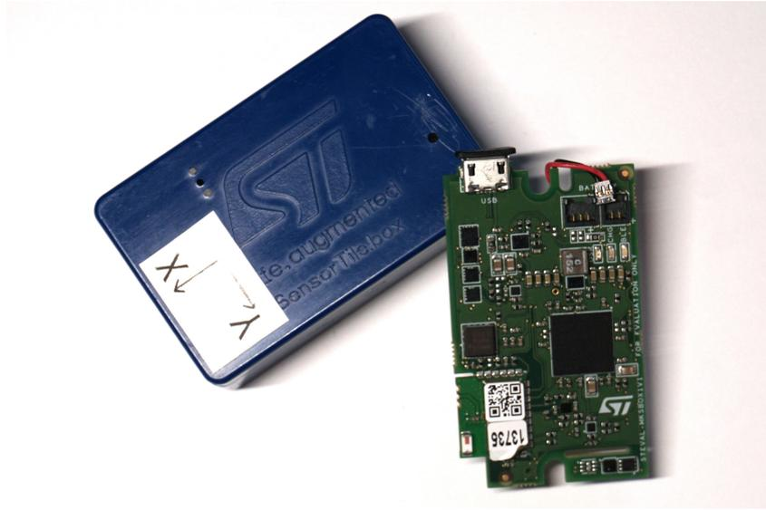
Figure 2.1: Image of the SensorTile.box, with the included case.
