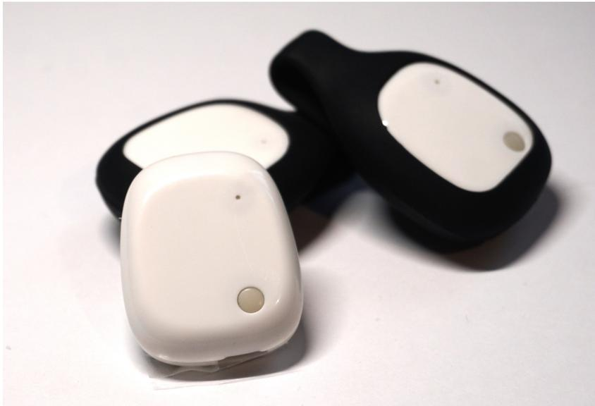
Figure 2.3: Image of the MetaMotionS devices, with and without the clip accessory.
