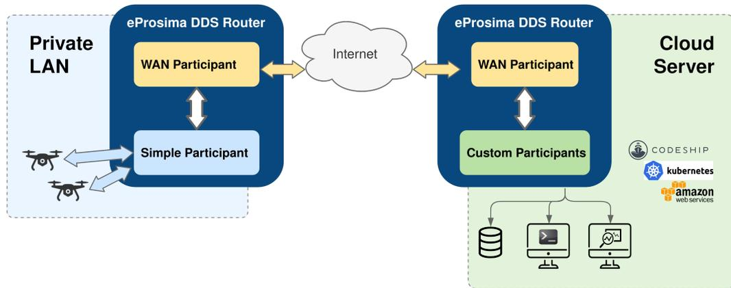
**Figure 6.4:** WAN communication with the DDS Router
