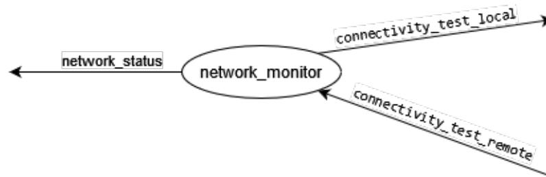
Figure 4.6: The `network_monitor` node
