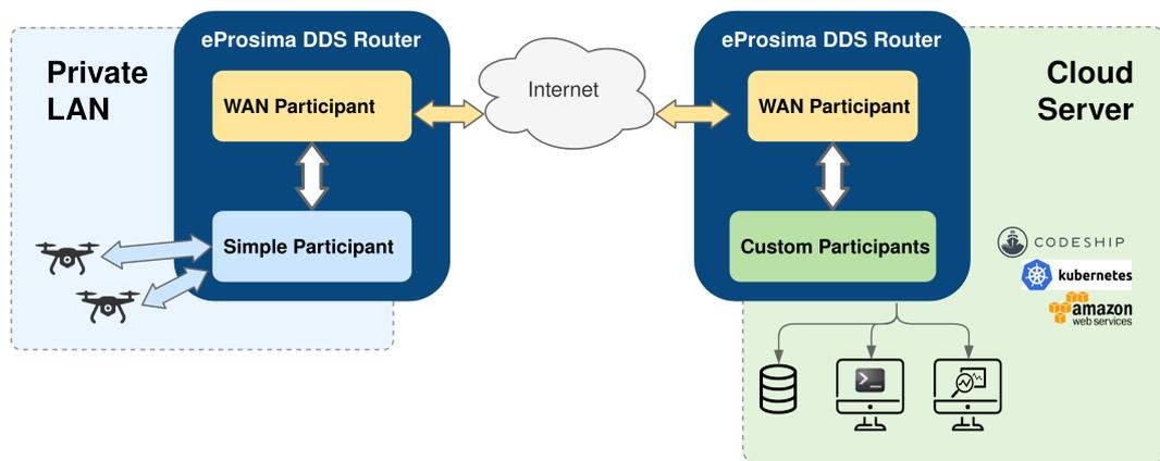
**Figure 4.3:** WAN communication with the DDS Router
