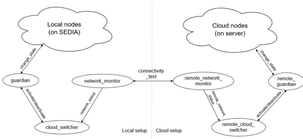
**Figure 4.5:** Switching mechanism architecture
