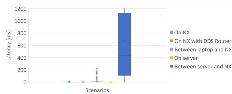
**Figure 7.15:** Latency distributions with remote communication
