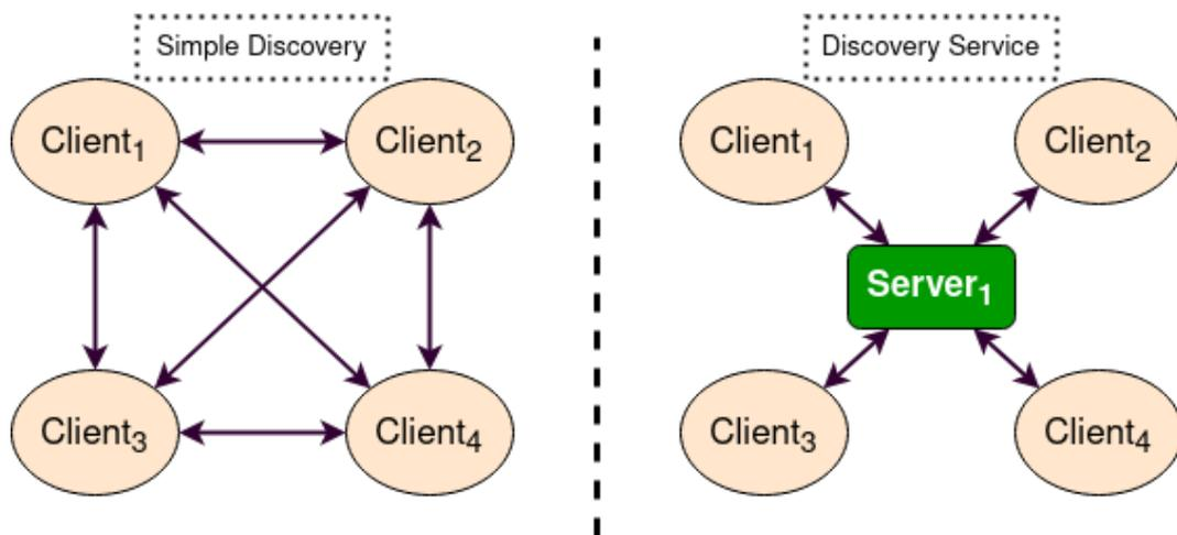
**Figure 6.3:** Fast DDS Discovery Server
