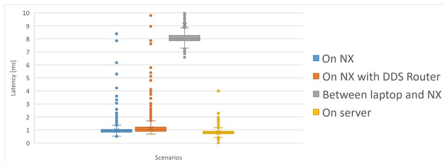
**Figure 7.14:** Latency distributions without remote communication
