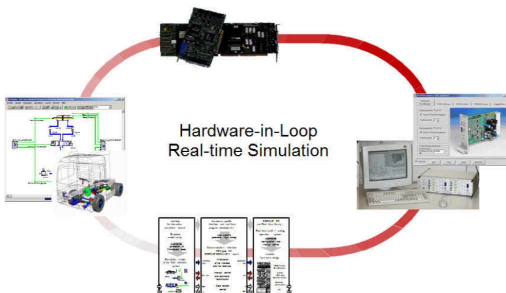
Figure 2.1 - Hardware-the-loop Simulation
