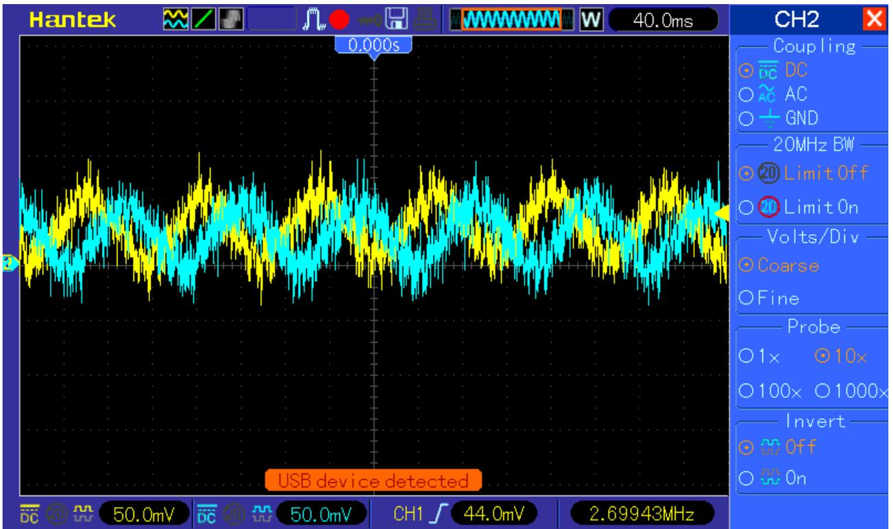
Figure 10.7 – Clarke & Park transform through Oscilloscope
