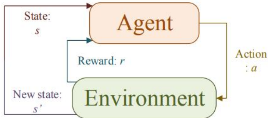
Figure 3.1: General diagram of a RL process. Taken from [26]
