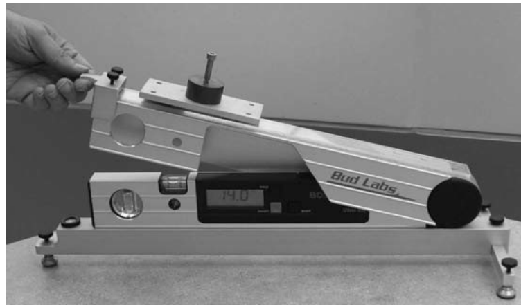
Figure 2.3: Commercial static friction test bench [1].
