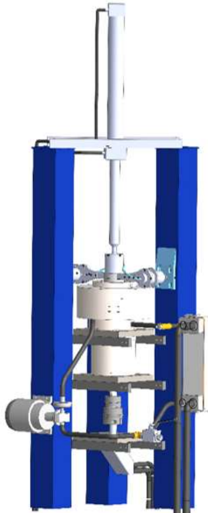
Figure 2.14: Test bench: disc on disc tribometer [21]
