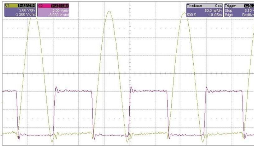
Figure 3.9 –  $V_{DS}$ -time characteristic of the prototype at nominal operation
