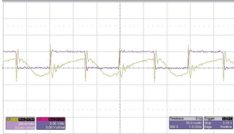
Figure 3.7 –  $I_{inv}$ -time characteristic of the prototype at nominal operation
