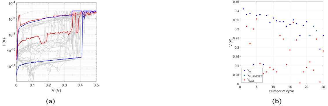
**Figure A.5:** Sample Pt/10nm SiO<sub>2</sub>/2.5nm Al<sub>2</sub>O<sub>3</sub>/Ag. On the left (a), the current response to voltage sweep, with  $I_{CC} = 10\mu A$ , is plotted for each cycle (y-axis in logarithmic scale). I-Vs in blue and red highlight two typical kinds of response. On the right (b), the evolution of  $V_{th}$  (blue) and  $V_{hold}$  (red) as function of number of cycles.
