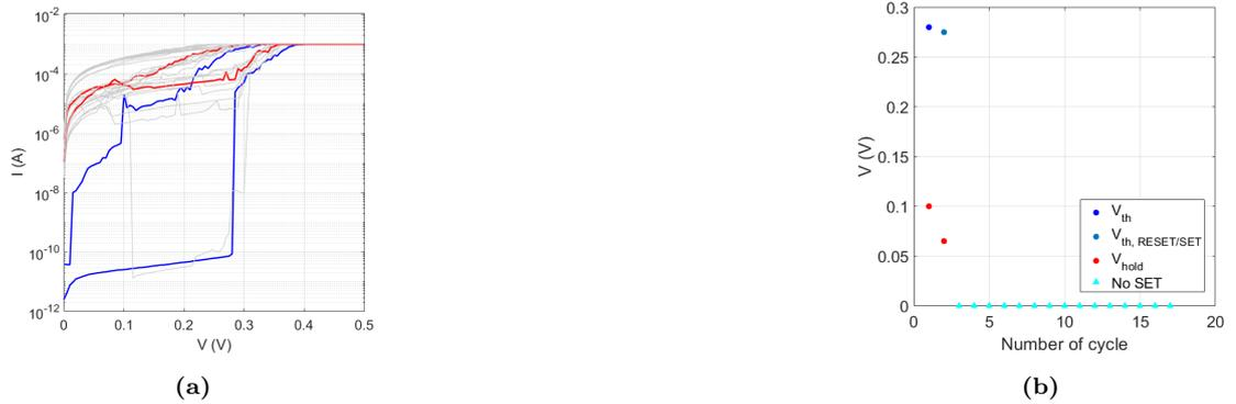
**Figure A.3:** Sample Pt/10nm SiO<sub>2</sub>/1nm Al<sub>2</sub>O<sub>3</sub>/Ag. (a) Current response to voltage sweep, with  $I_{CC} = 1mA$ , is plotted for each cycle (y-axis in logarithmic scale). I-Vs in blue and red highlight two kinds of response. (b) Evolution of  $V_{th}$  (blue) and  $V_{hold}$  (red) as function of number of cycles.
