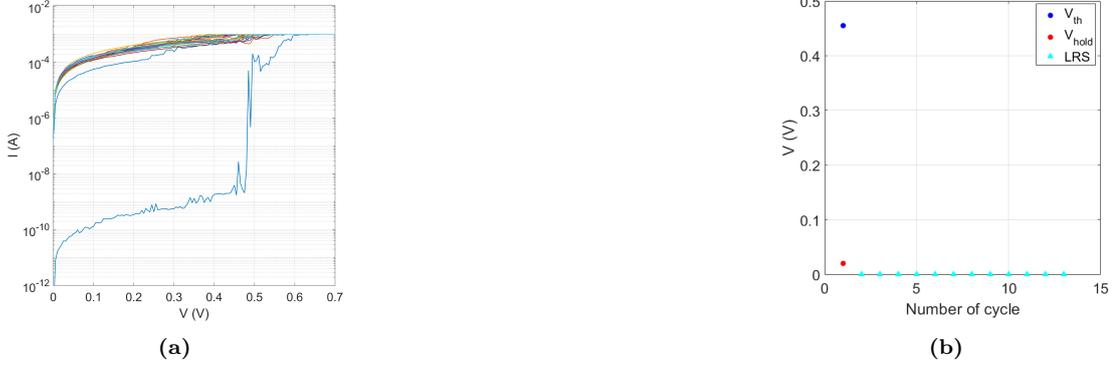
**Figure A.6:** Sample Pt/10nm SiO<sub>2</sub>/2.5nm Al<sub>2</sub>O<sub>3</sub>/Ag. (a) Current response to voltage sweep, with  $I_{CC} = 1\text{mA}$ , is plotted for each cycle (y-axis in logarithmic scale). (b) Evolution of  $V_{th}$  (blue) and  $V_{hold}$  (red) as function of number of cycles.
