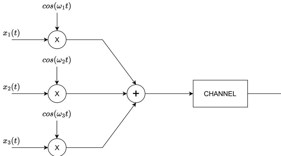
Figure 5.4: Frequency Division Multiplexing basic scheme
