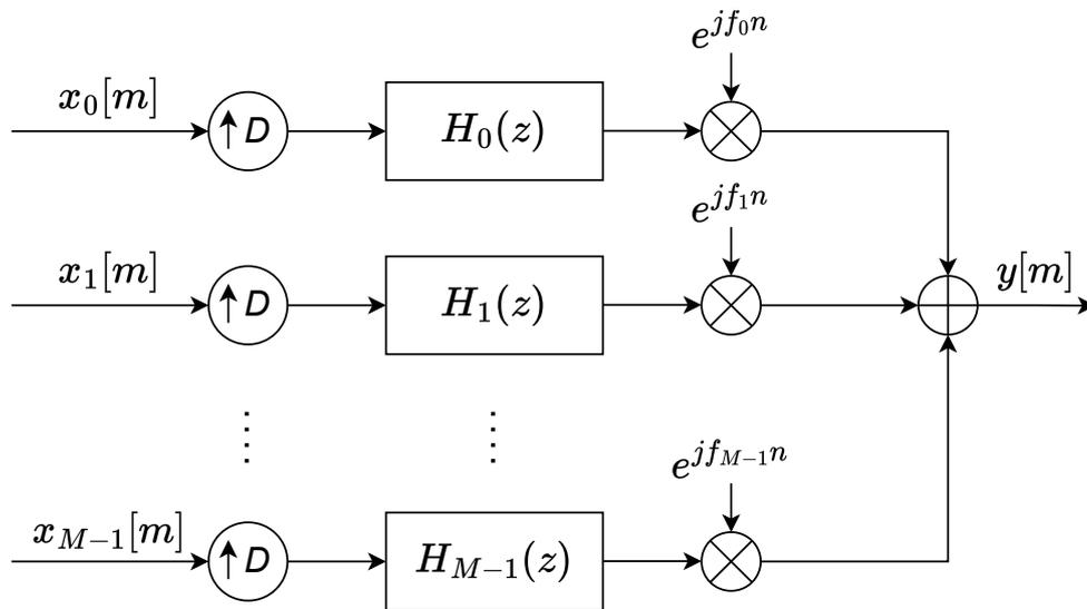
Figure 5.5: Synthesis filter bank conceptual diagram
