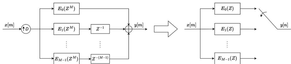
Figure 5.7: Example of noble identity application to a low-pass polyphase filter (polyphase interpolator)
