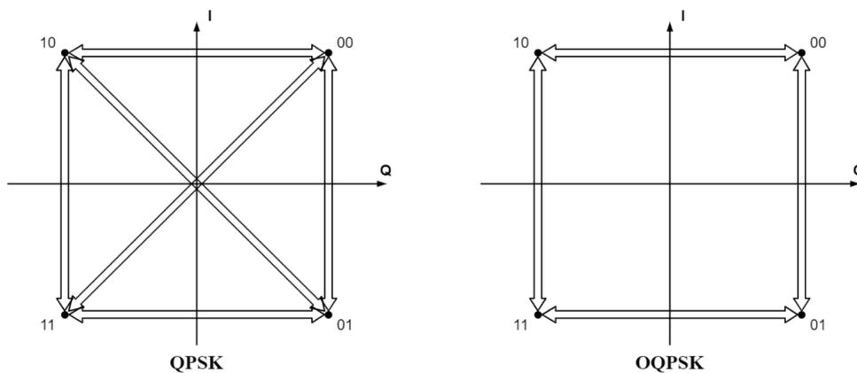
Figure 5.3: Possible phase changes in QPSK and OQPSK
