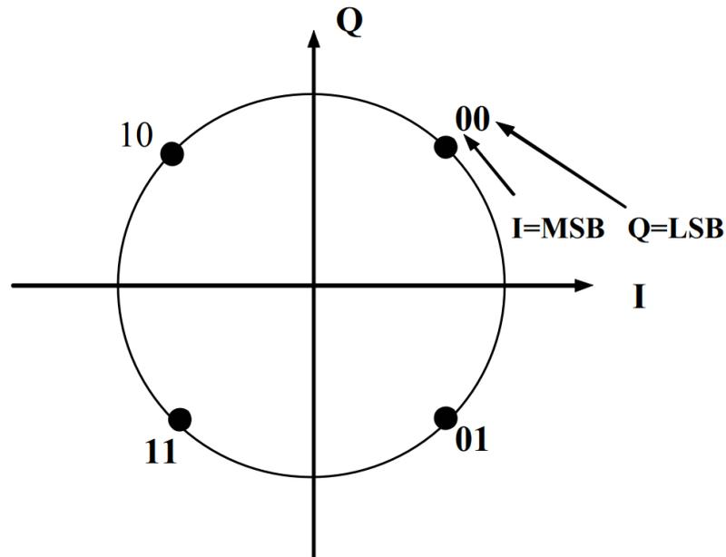
Figure 5.2: Gray mapping for the QPSK constellation
