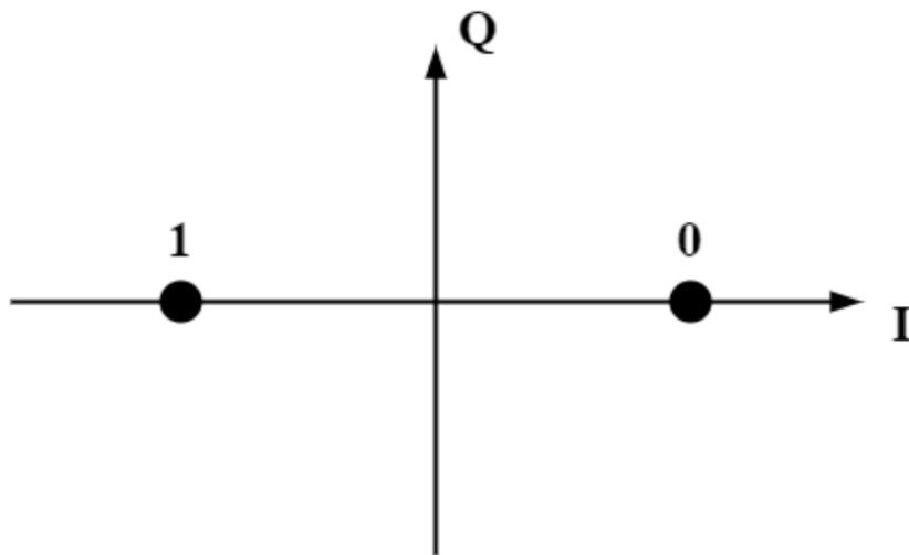
Figure 5.1: Mapping for the BPSK constellation
