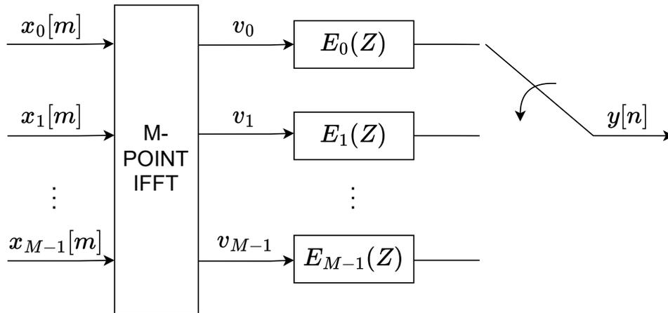
Figure 5.8: Polyphase synthesizer schematic
