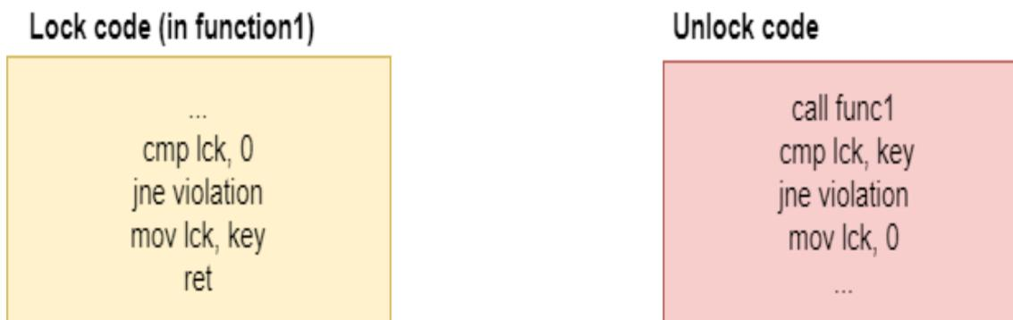
Figure 3.3: Label-based instrumentation code
