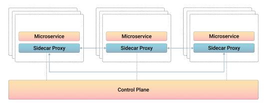
Figure 4.2: Service Mesh Architecture.
