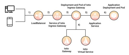
Figure 6.2: Basic flow of a request.
