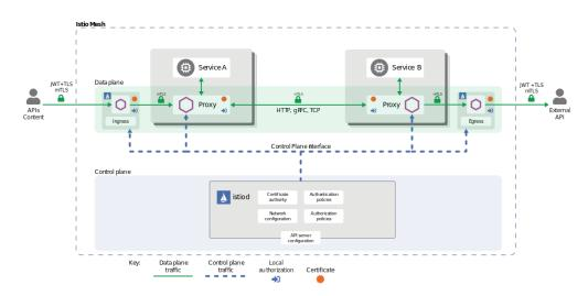
Figure 6.3: Istio Security Architecture [19].
