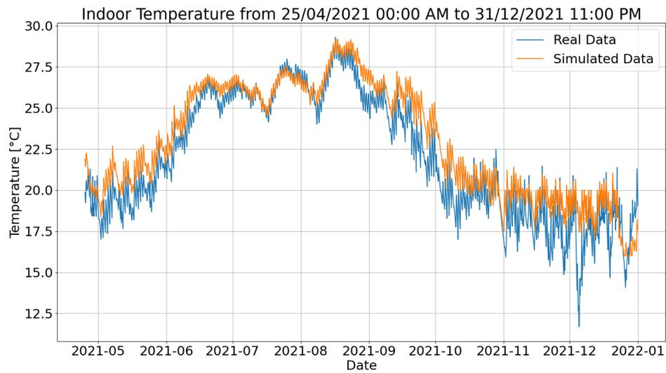
Figure 5.11: Simulated temperature behavior of the room *act201bc* in 2021
