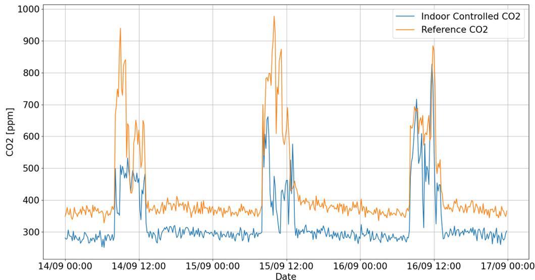
Figure 13.58: Controlled and reference carbon dioxide concentration in the room *act201cc* with the 800ppm single threshold approach
