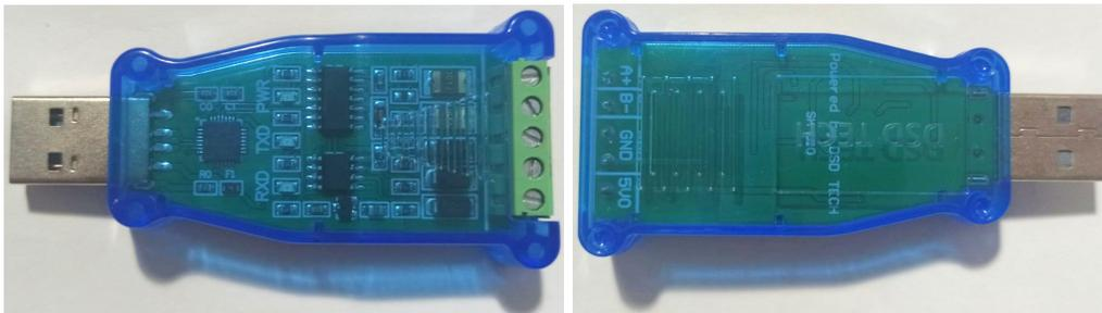
Figure 10.4: USB to RS485 Converter
