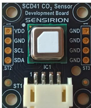
Figure 10.5: Sensirion SEK-SCD41 CO2 Sensor Evaluation Kit
