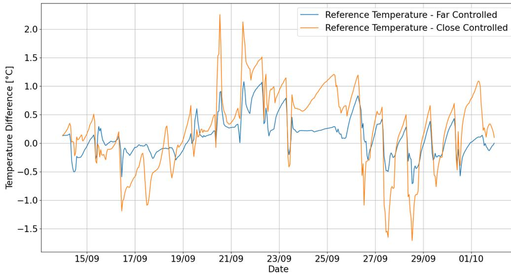
Figure 13.42: Difference between reference room temperature and controlled one from far and near the mechanical ventilation unit
