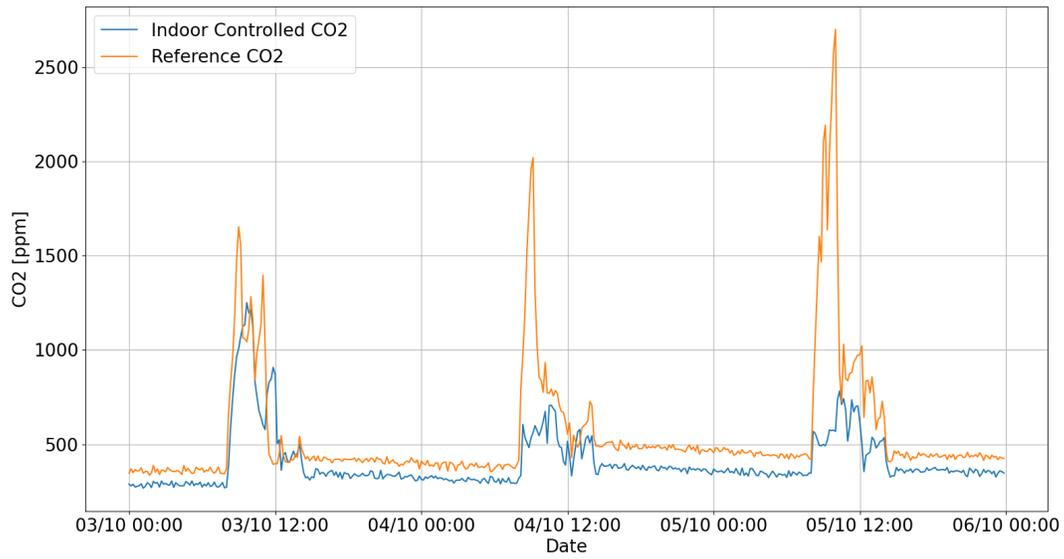
Figure 13.49: Controlled and reference carbon dioxide concentration in the room *act201bc* with the  $600ppm$  double threshold approach on the second floor
