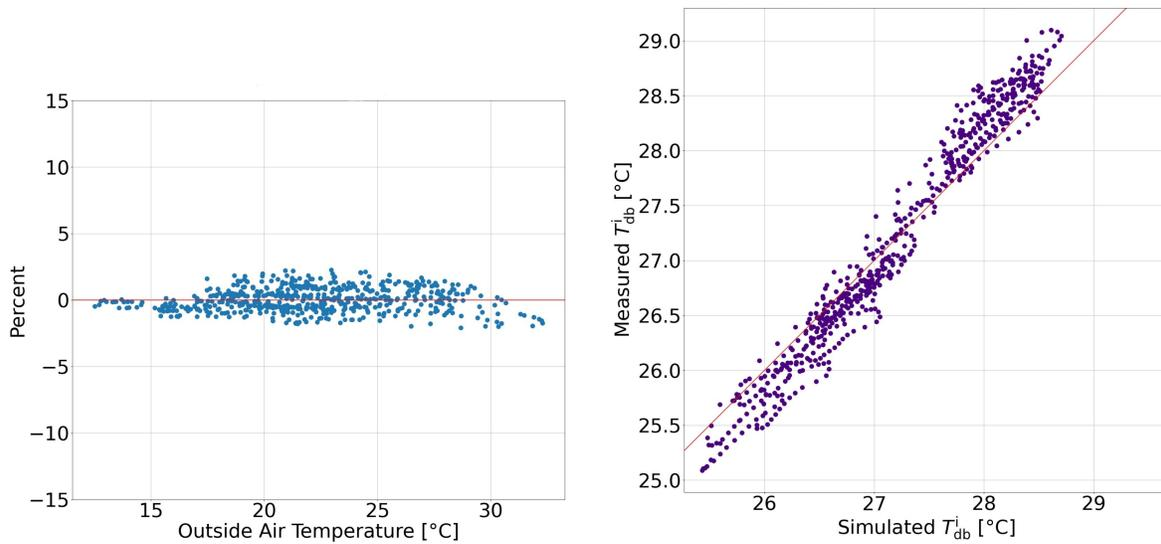
Figure 5.6: Calibration signature on the left and measured vs simulated data on the right for the room *act201cc*
