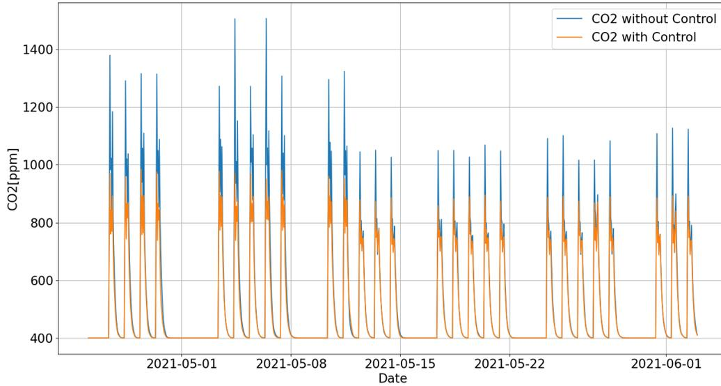
Figure 9.12: Indoor CO<sub>2</sub> behavior of the free-running building compared with the controlled one over the selected period
