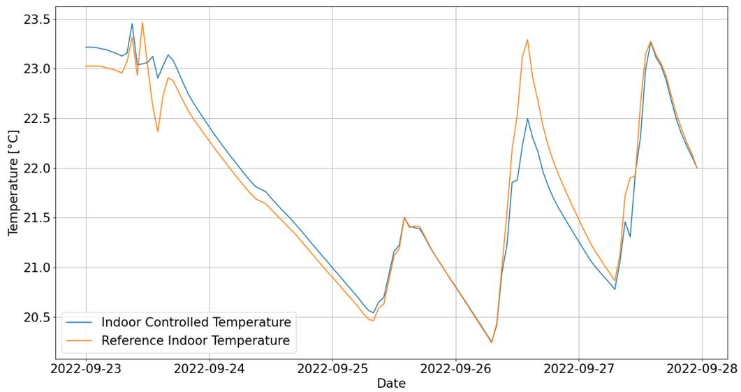
Figure 13.57: Temperature in the room *act201bc* and in the reference one with the 1000ppm single threshold approach
