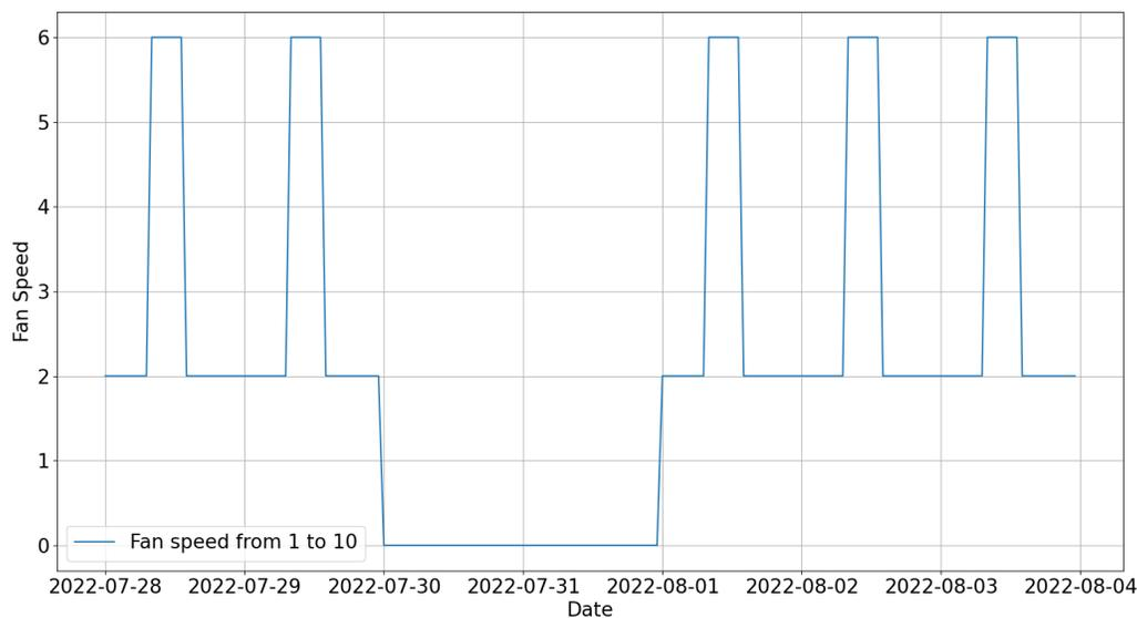
Figure 13.33: Ventilation rate of the mechanical ventilation system in the room *acr208da* during the third week
