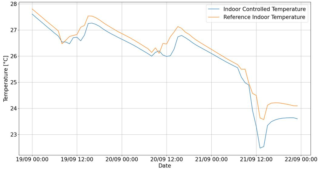
Figure 13.63: Temperature in the room *act201bc* and in the reference one with the 800ppm double threshold approach
