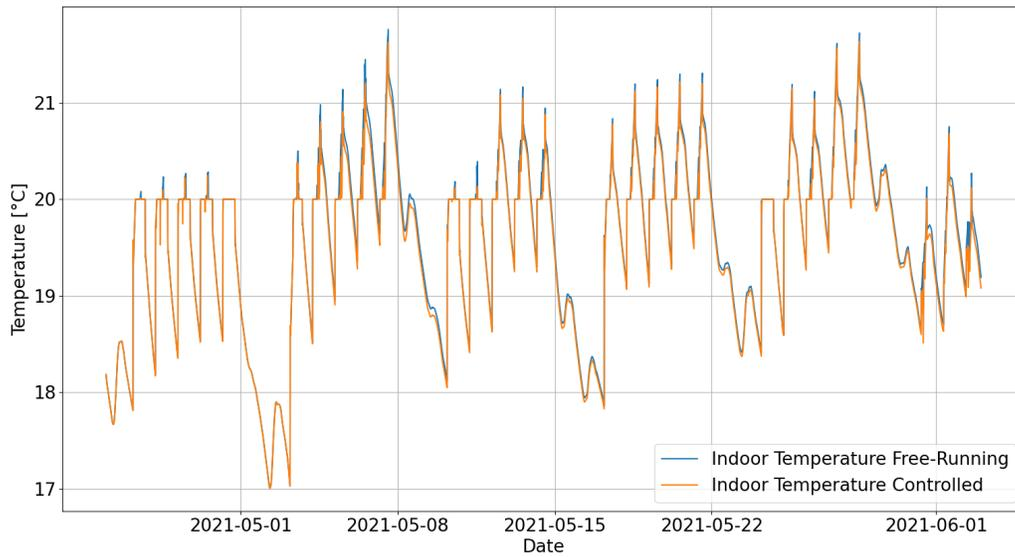
Figure 9.19: Indoor temperature behavior of the free-running building compared with the controlled one over the selected period
