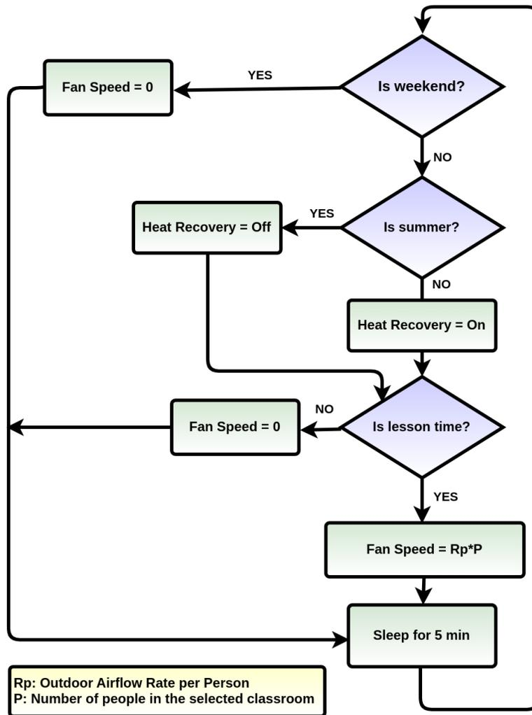
Figure 8.1: Ventilation algorithm recommended from the ASHRAE 62
