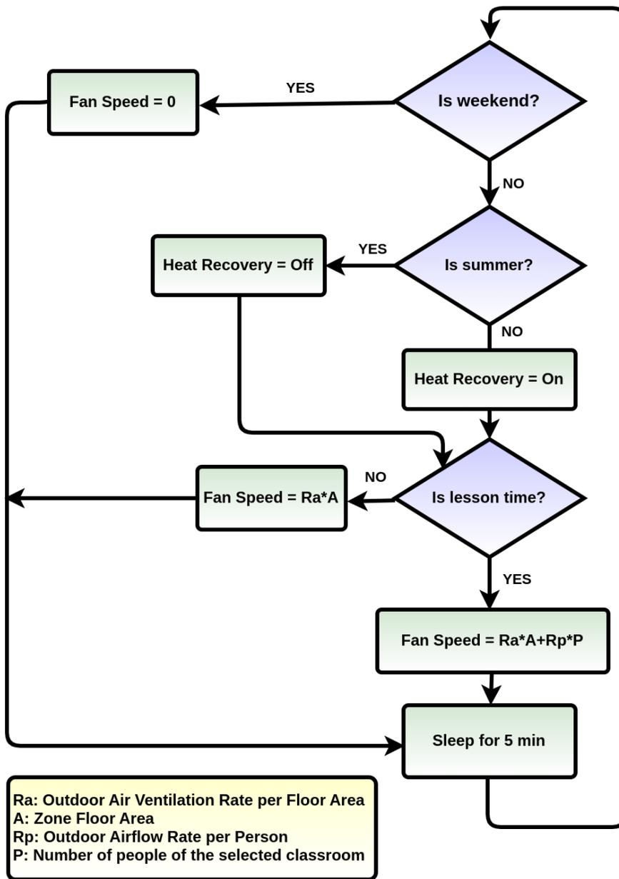
Figure 12.7: Ventilation algorithm recommended from the ASHRAE 62.1
