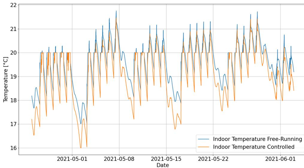
Figure 9.7: Indoor temperature behavior of the free-running building compared with the controlled one over the selected period
