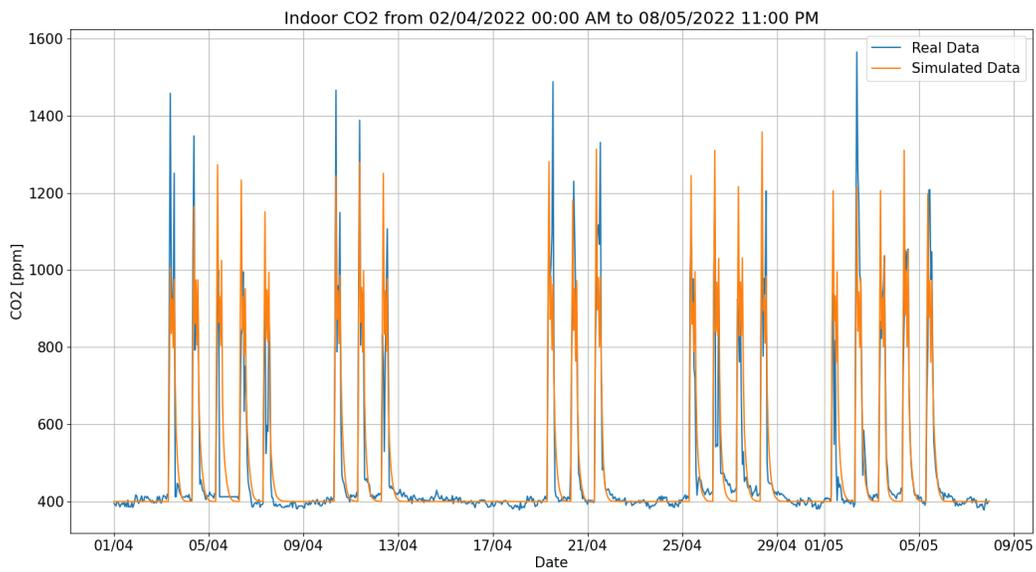
Figure 5.22: Simulated  $CO_2$  behavior of the room *act201bc* after mechanical ventilation calibration
