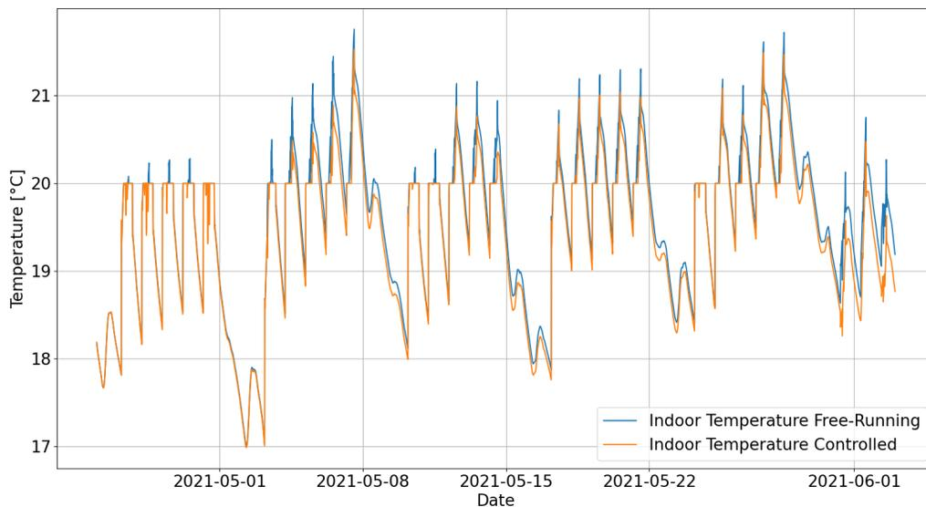
Figure 9.4: Indoor temperature behavior of the free-running building compared with the controlled one over the selected period
