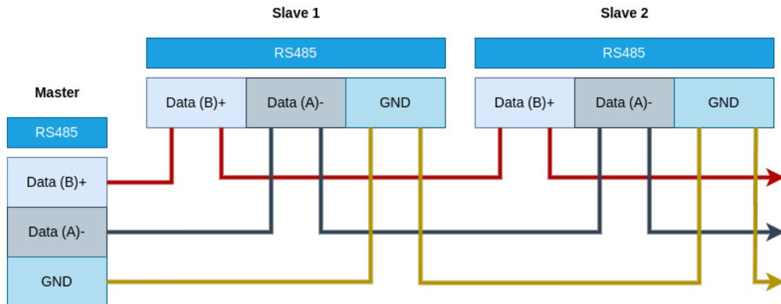
Figure 4.1: Modbus RS485 connection scheme
