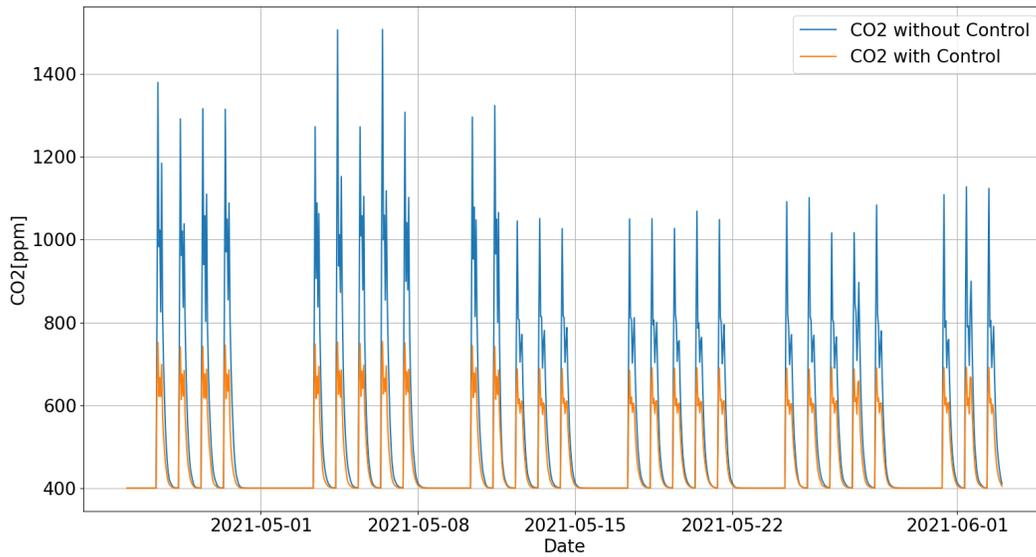
Figure 9.3: Indoor  $CO_2$  behavior of the free-running building compared with the controlled one over the selected period
