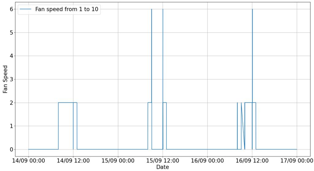
Figure 13.44: Ventilation rate of the mechanical ventilation system in the room *act201bc* with the  $600ppm$  single threshold approach
