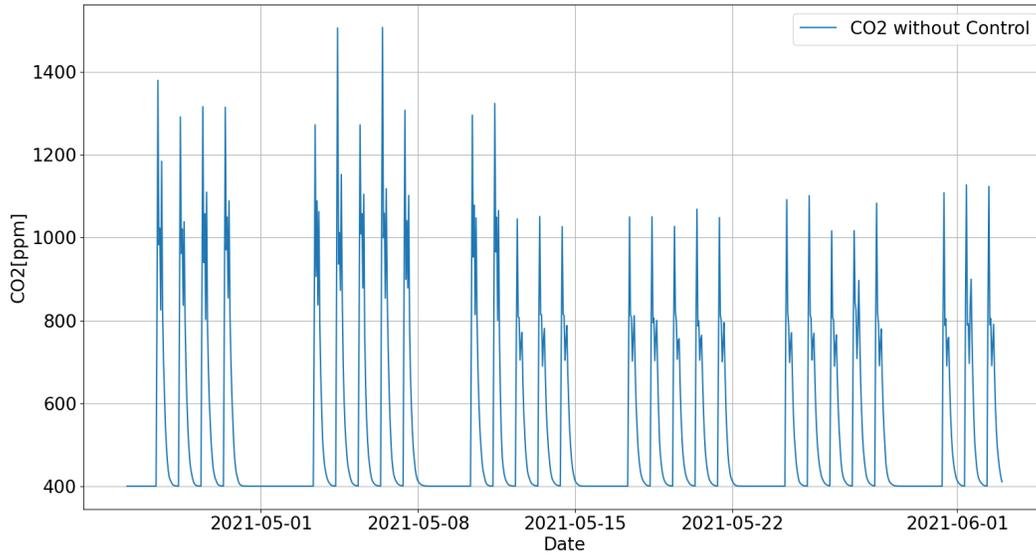
Figure 9.2: Indoor  $CO_2$  behavior of the free-running building over the selected period
