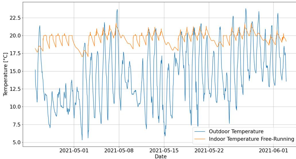
Figure 9.1: Indoor and outdoor temperature behavior of the free-running building over the selected period
