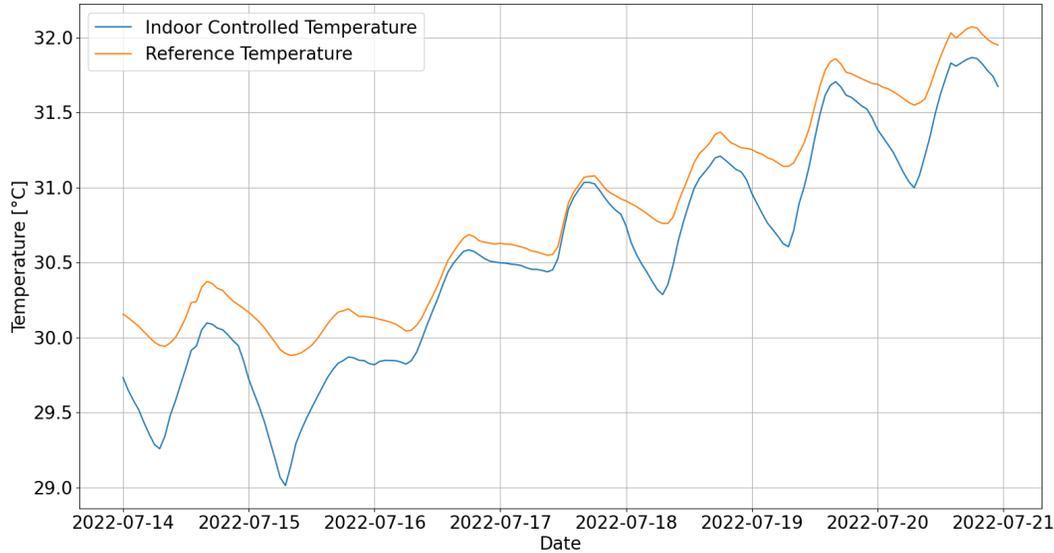
Figure 13.25: Controlled and reference temperature of *act208da* in the first week
