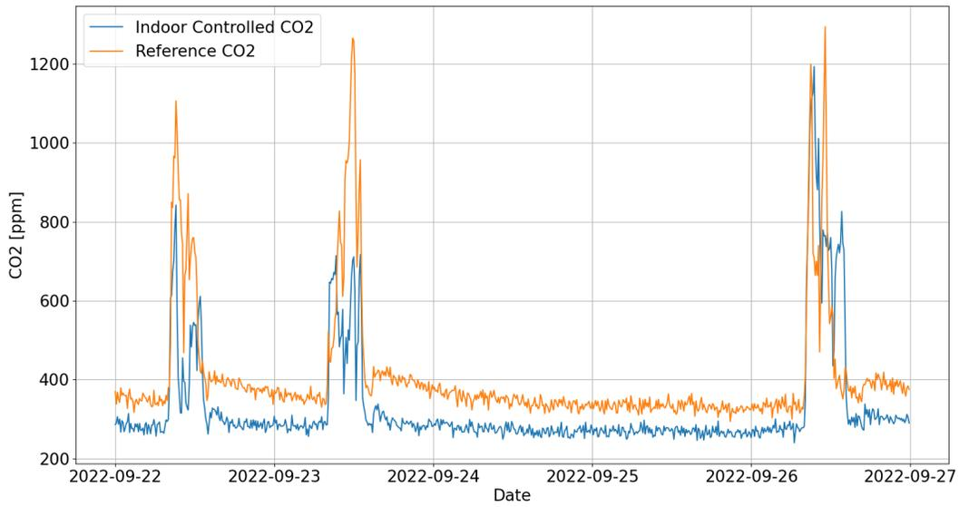
Figure 13.64: Controlled and reference carbon dioxide concentration in the room *act201cc* with the ASHRAE 62.1 approach
