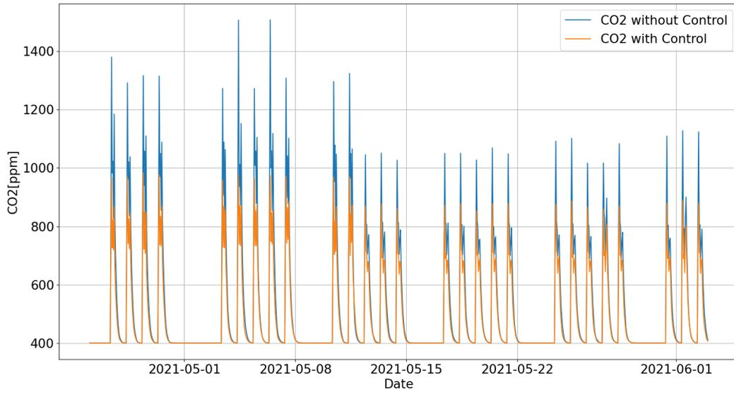
Figure 9.9: Indoor  $CO_2$  behavior of the free-running building compared with the controlled one over the selected period
