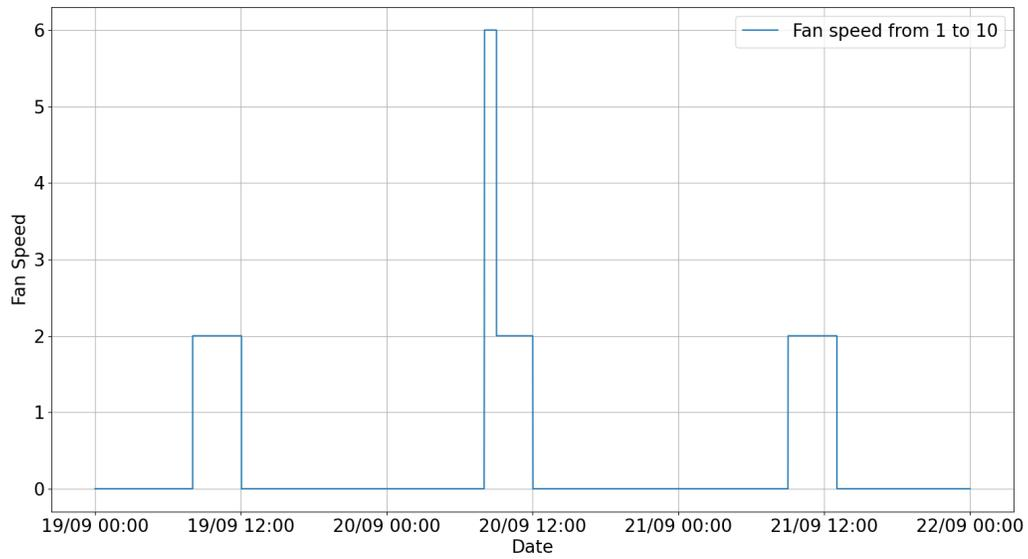
Figure 13.62: Ventilation rate of the mechanical ventilation system in the room *act201cc* with the  $800ppm$  double threshold approach
