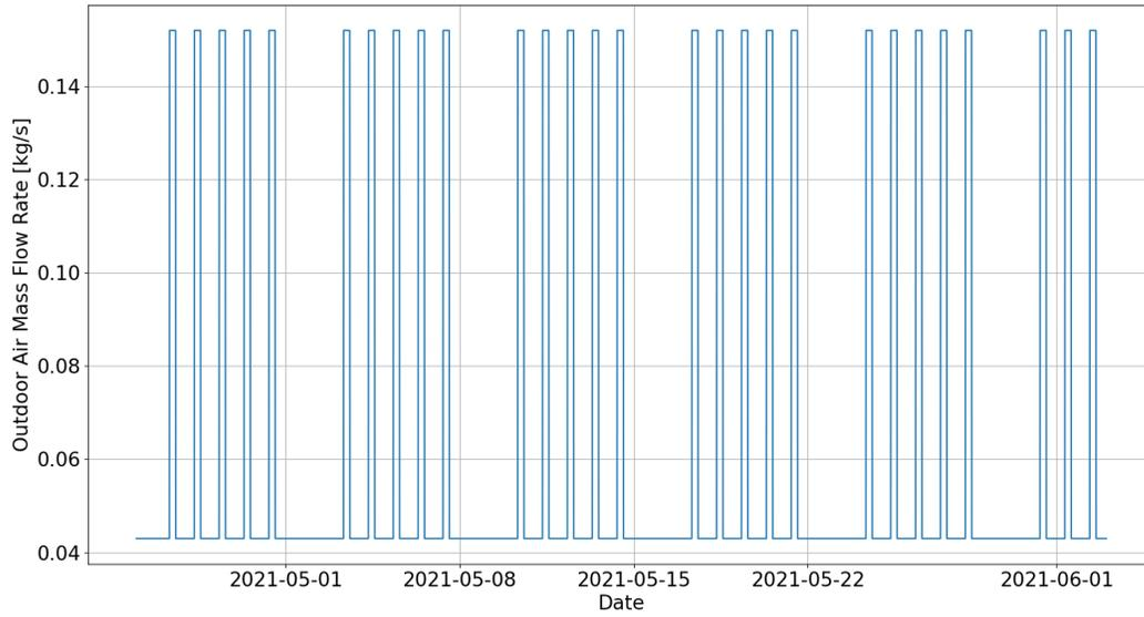
Figure 9.8: Ventilation airflow rate over the selected period
