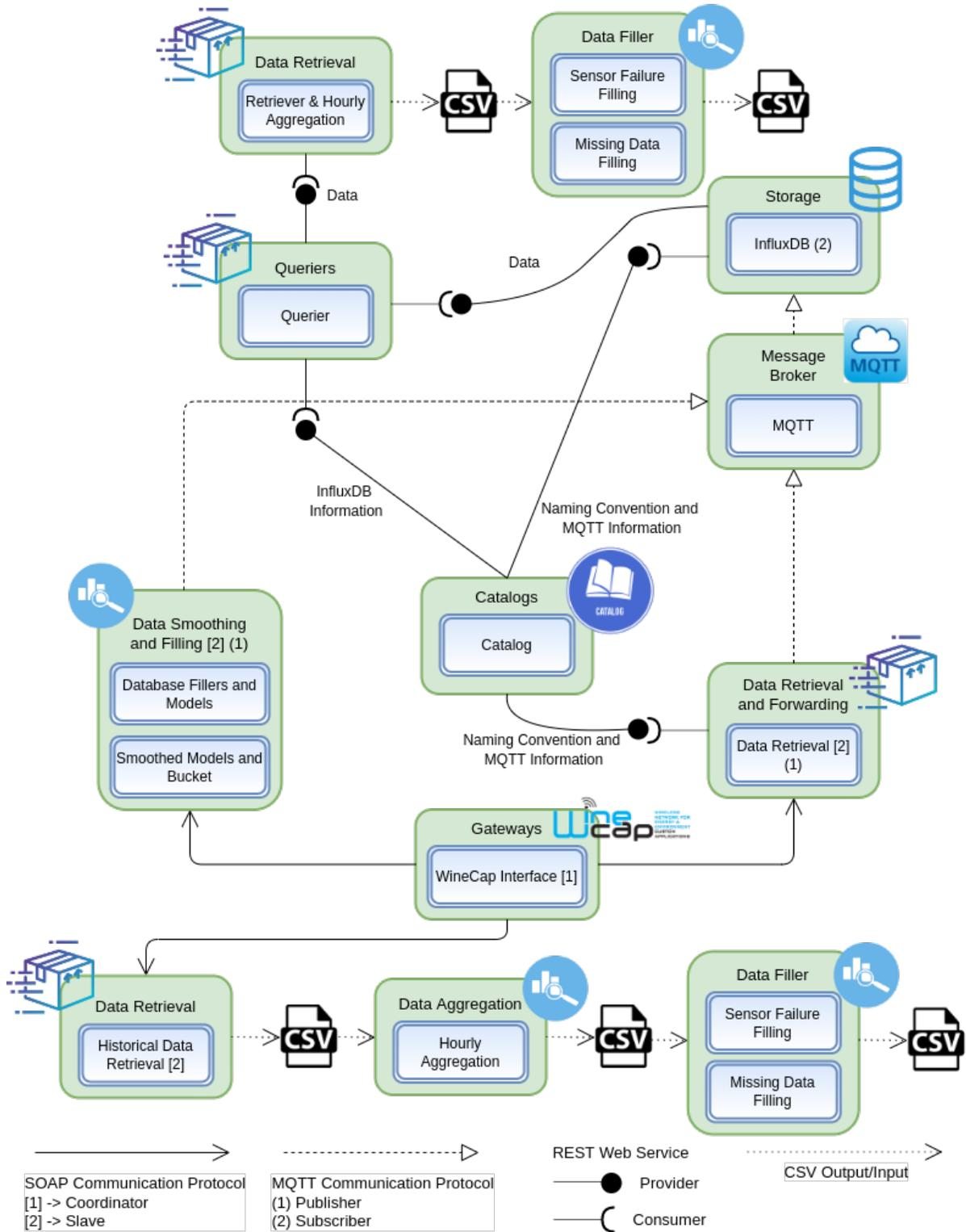
Figure 7.1: General software structure for retrieving data to calibrate the models
