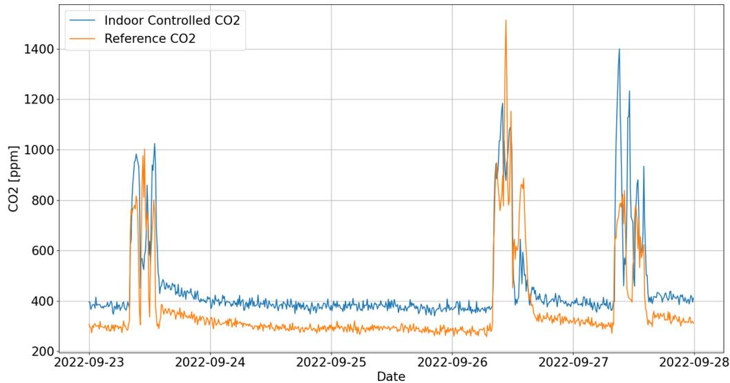
Figure 13.55: Controlled and reference carbon dioxide concentration in the room *act201cc* with the 1000ppm single threshold approach
