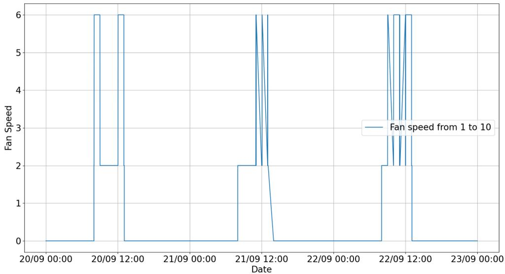
Figure 13.47: Ventilation rate of the mechanical ventilation system in the room *act201bc* with the 600ppm double threshold approach
