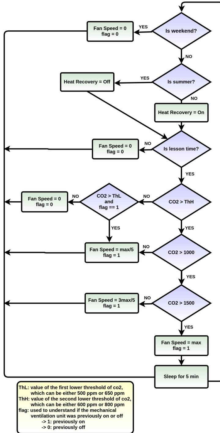
Figure 8.3: Ventilation algorithm based on a double  $CO_2$  threshold
