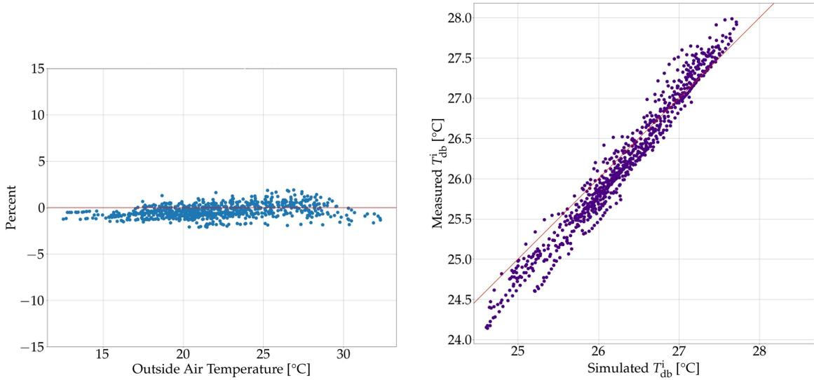
Figure 5.5: Calibration signature on the left and measured vs simulated data on the right for the room *act201bc*
