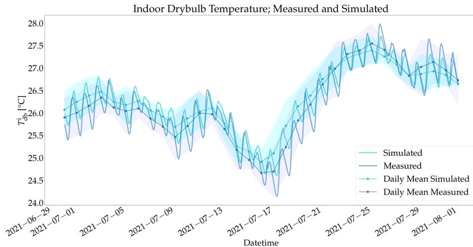
Figure 5.8: Simulated vs measured temperature behavior in the calibration period for the room *act201bc*
