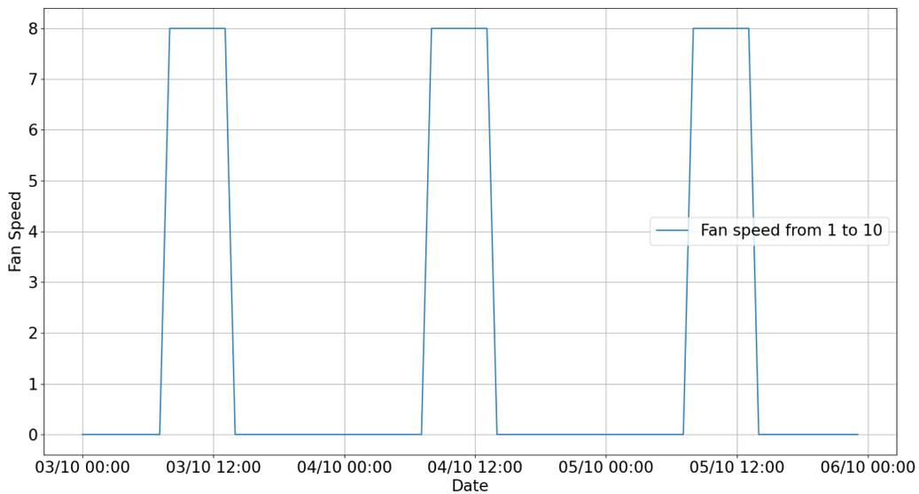
Figure 13.53: Ventilation rate of the mechanical ventilation system in the room *act201bc* with the ASHRAE 62 approach
