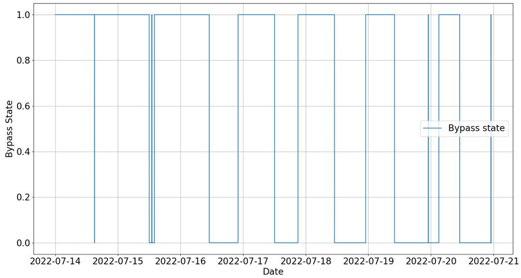
Figure 13.8: Heat recovery bypass of *act201bc* in the first week
