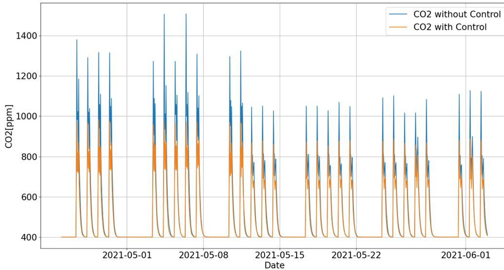
Figure 9.15: Indoor  $CO_2$  behavior of the free-running building compared with the controlled one over the selected period
