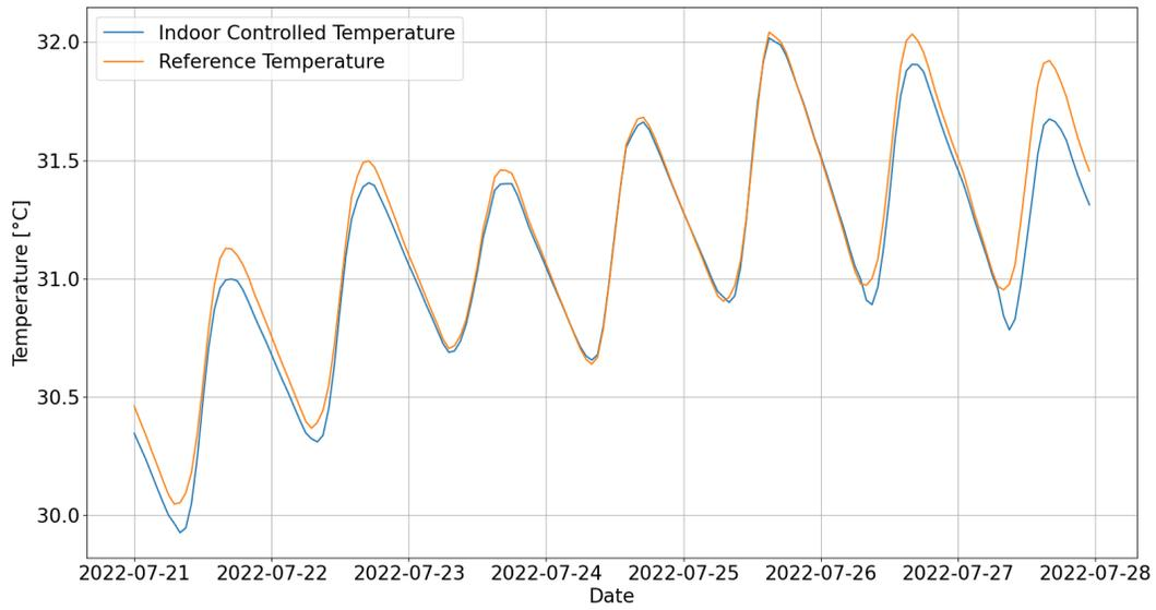
Figure 13.10: Controlled and reference temperature of *act201bc* in the second week
