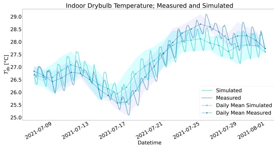
Figure 5.9: Simulated vs measured temperature behavior in the calibration period for the room *act201cc*
