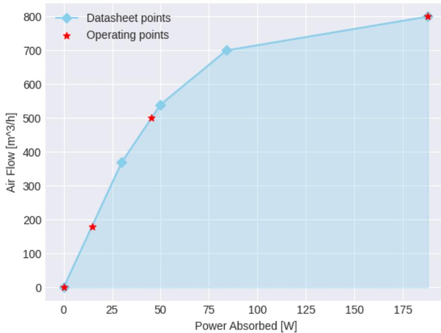
Figure 5.20: Air flow with respect to the absorbed power
