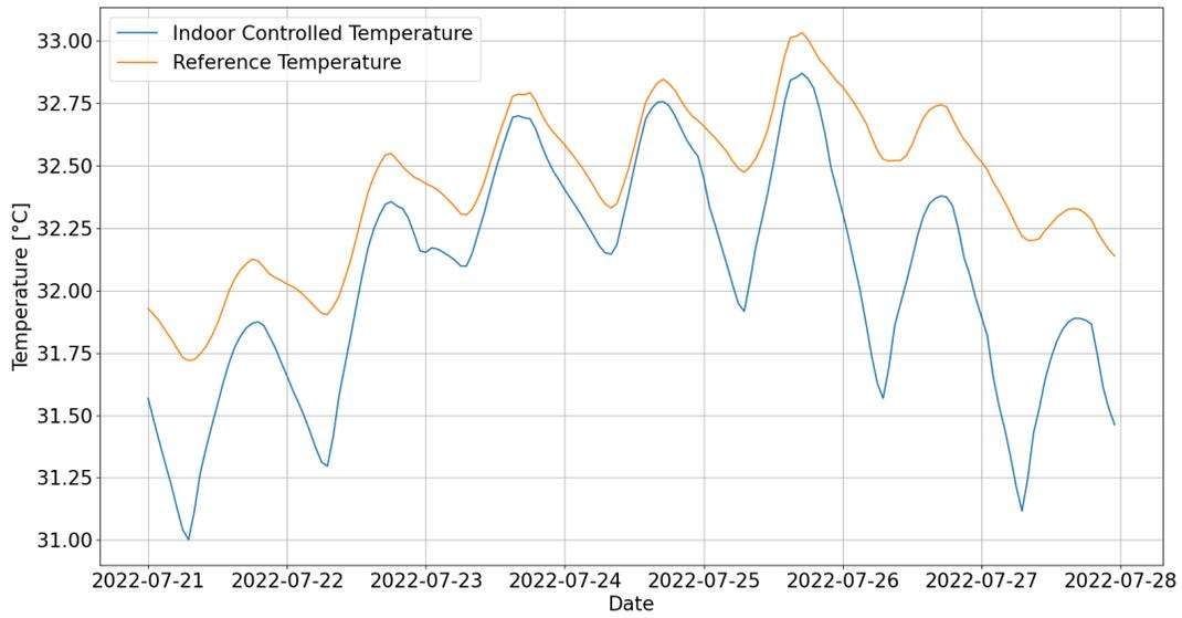
Figure 13.28: Controlled and reference temperature of *act208da* in the second week
