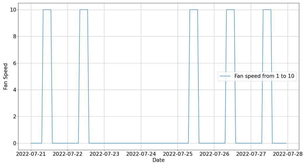
Figure 13.21: Ventilation rate of the mechanical ventilation system in the room *act201cc* during the second week
