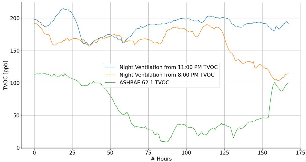
Figure 13.37: Comparison of the TVOC reduction in the room *act208da* in all the testing weeks
