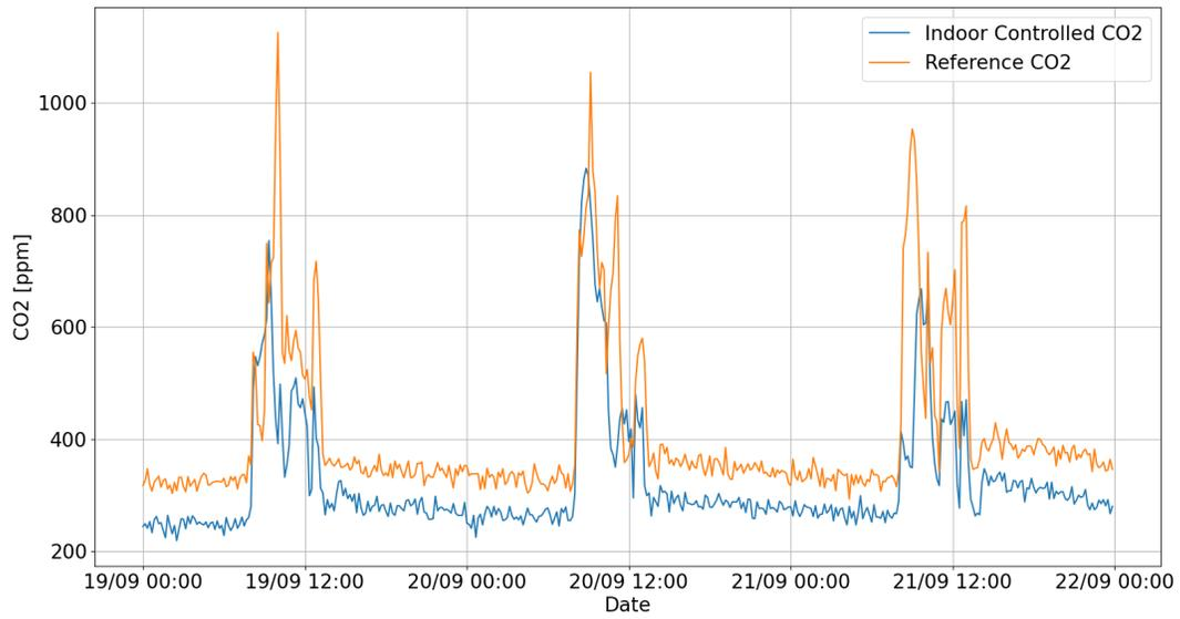
Figure 13.61: Controlled and reference carbon dioxide concentration in the room *act201cc* with the  $800ppm$  double threshold approach
