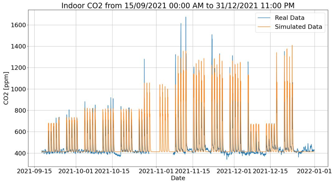
Figure 5.18: Simulated  $CO_2$  behavior of the room *act201bc* in the second part of 2021
