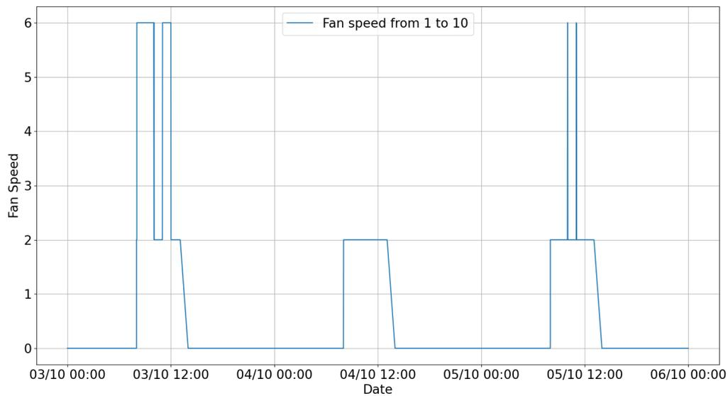
Figure 13.50: Ventilation rate of the mechanical ventilation system in the room *act201bc* with the  $600ppm$  double threshold approach on the second floor
