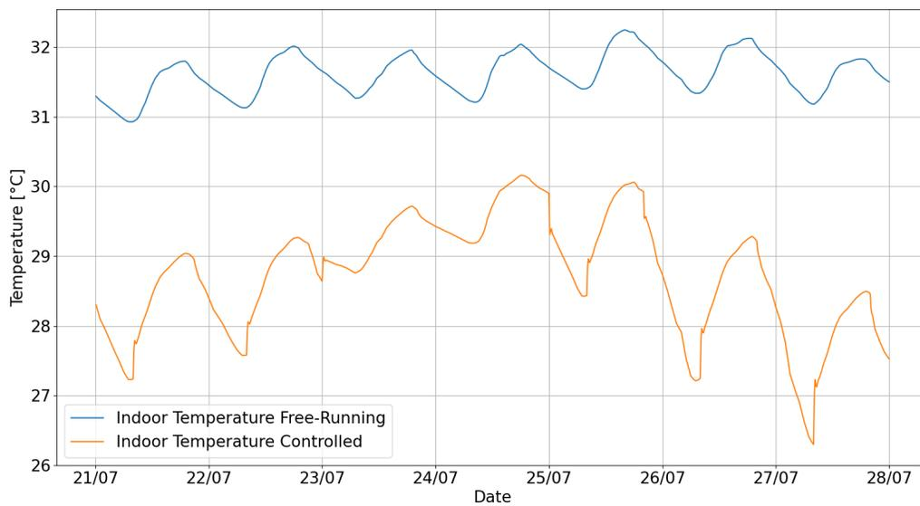
Figure 13.39: Free-running and controlled indoor temperatures behaviors
