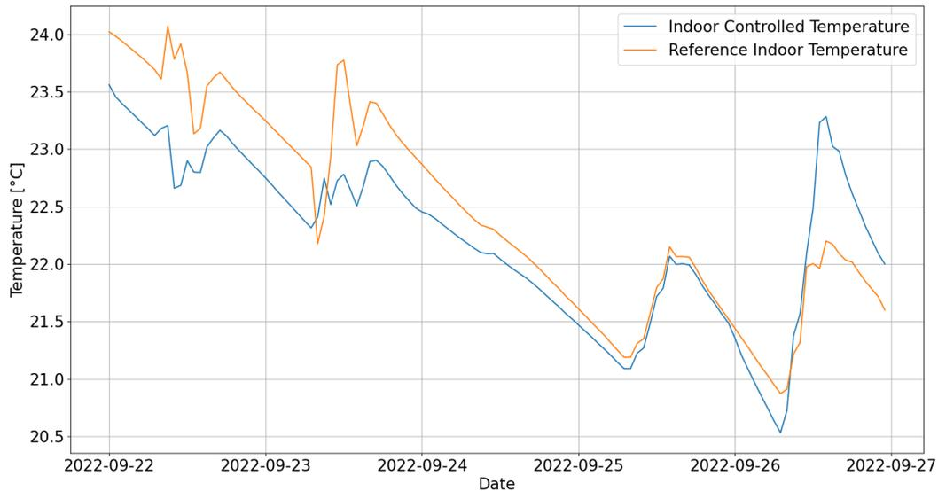
Figure 13.66: Temperature in the room *act201bc* and in the reference one with the ASHRAE 62.1 approach
