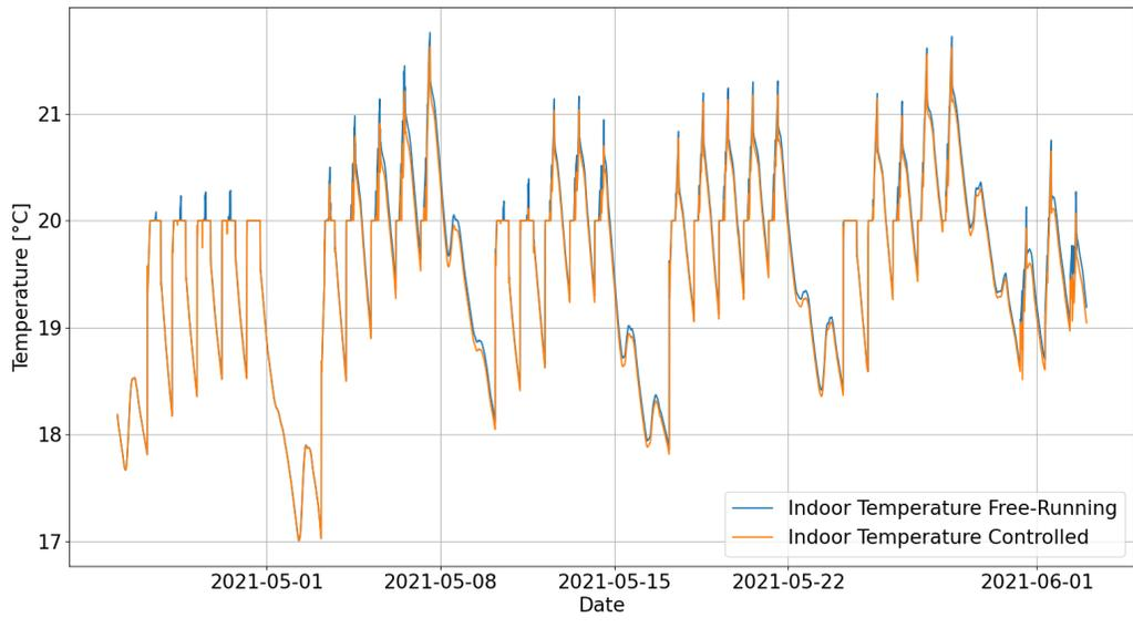
Figure 9.16: Indoor temperature behavior of the free-running building compared with the controlled one over the selected period
