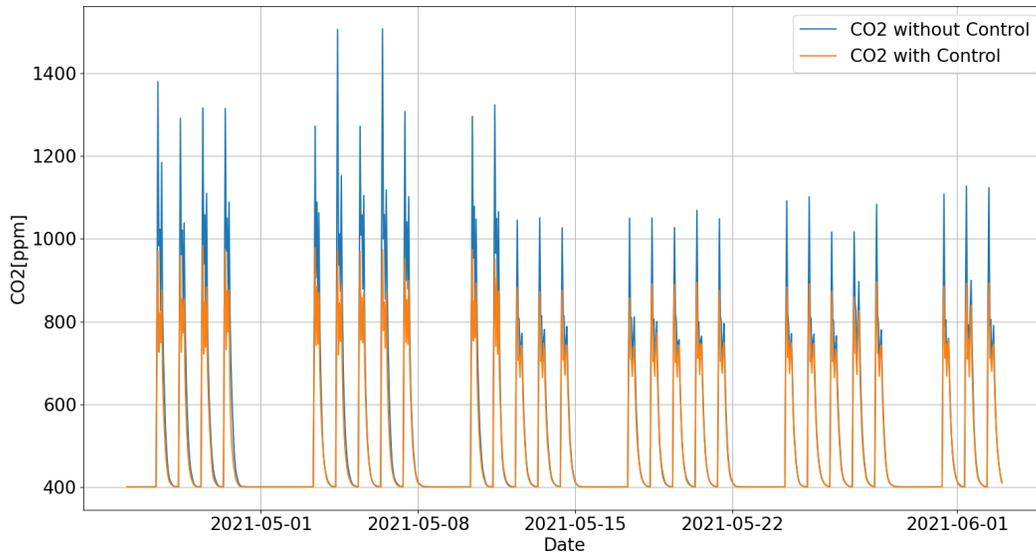
Figure 9.18: Indoor CO<sub>2</sub> behavior of the free-running building compared with the controlled one over the selected period
