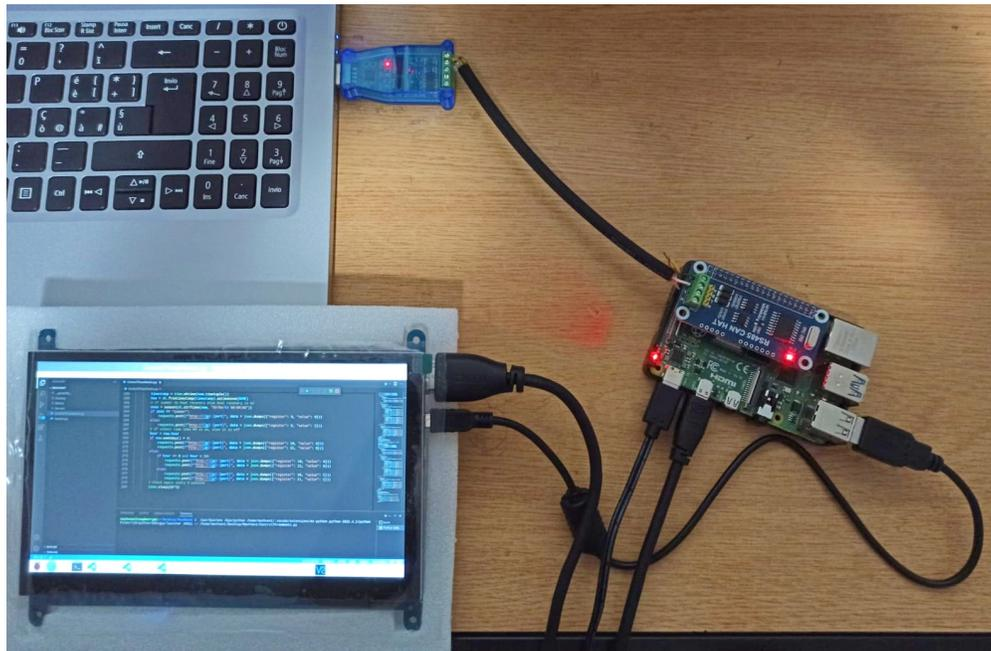
Figure 10.1: Hardware structure for testing the Modbus communication with the laptop
