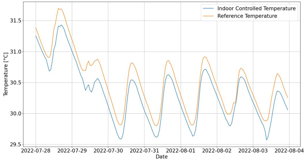
Figure 13.13: Controlled and reference temperature of *act201bc* in the third week
