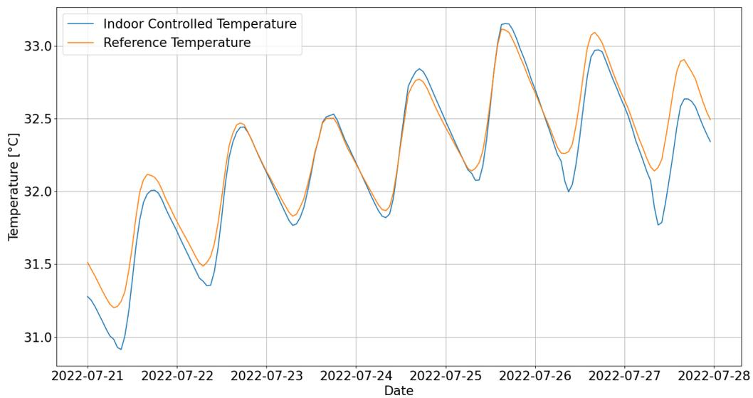
Figure 13.19: Controlled and reference temperature of *act201cc* in the second week
