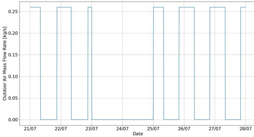
Figure 13.40: Airflow of the mechanical ventilation unit during the simulation
