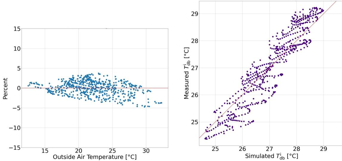
Figure 5.7: Calibration signature on the left and measured vs simulated data on the right for the room *act208da*
