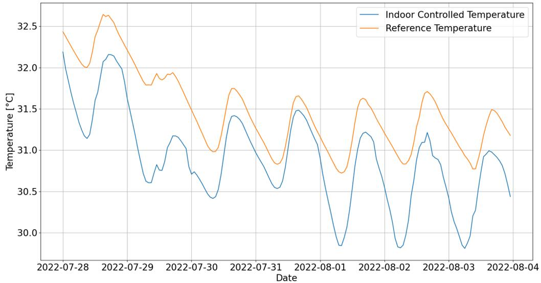
Figure 13.22: Controlled and reference temperature of *act201cc* in the third week
