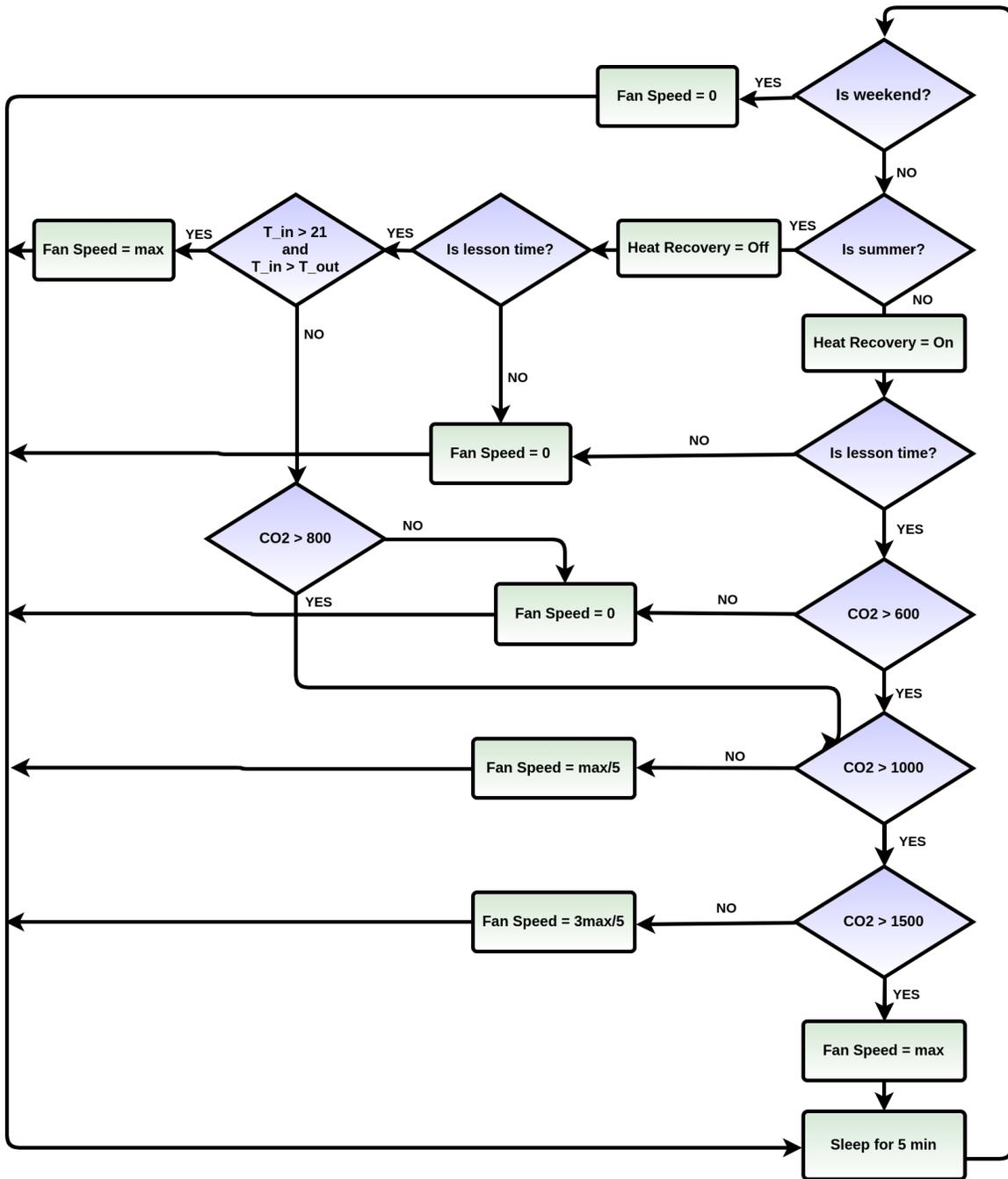
Figure 12.2: Temperature single threshold for ventilative cooling and CO<sub>2</sub>-based control for correct IAQ during lessons time
