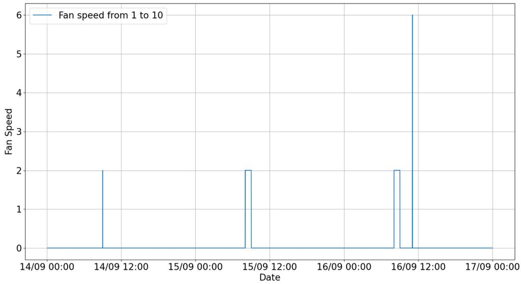
Figure 13.59: Ventilation rate of the mechanical ventilation system in the room *act201cc* with the  $800ppm$  single threshold approach
