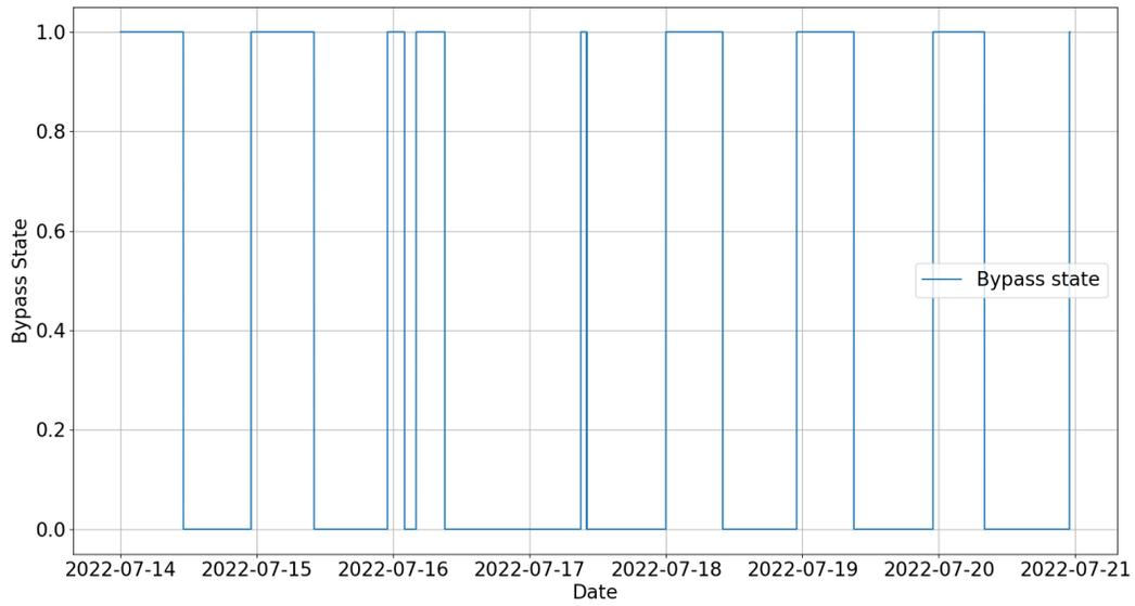
Figure 13.17: Heat recovery bypass of *act201cc* in the first week
