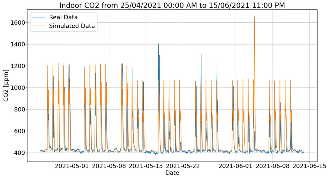
Figure 5.17: Simulated  $CO_2$  behavior of the room *act201bc* in the first part of 2021
