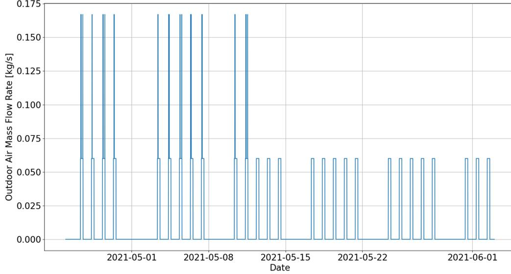
Figure 9.11: Ventilation airflow rate over the selected period
