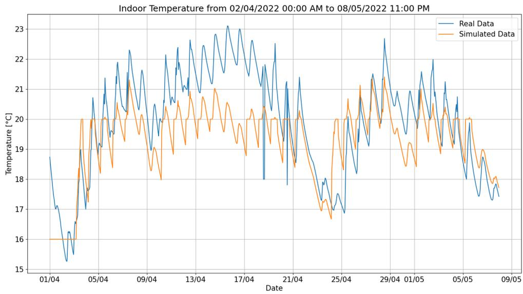
Figure 5.21: Simulated temperature behavior of the room *act201bc* after mechanical ventilation calibration
