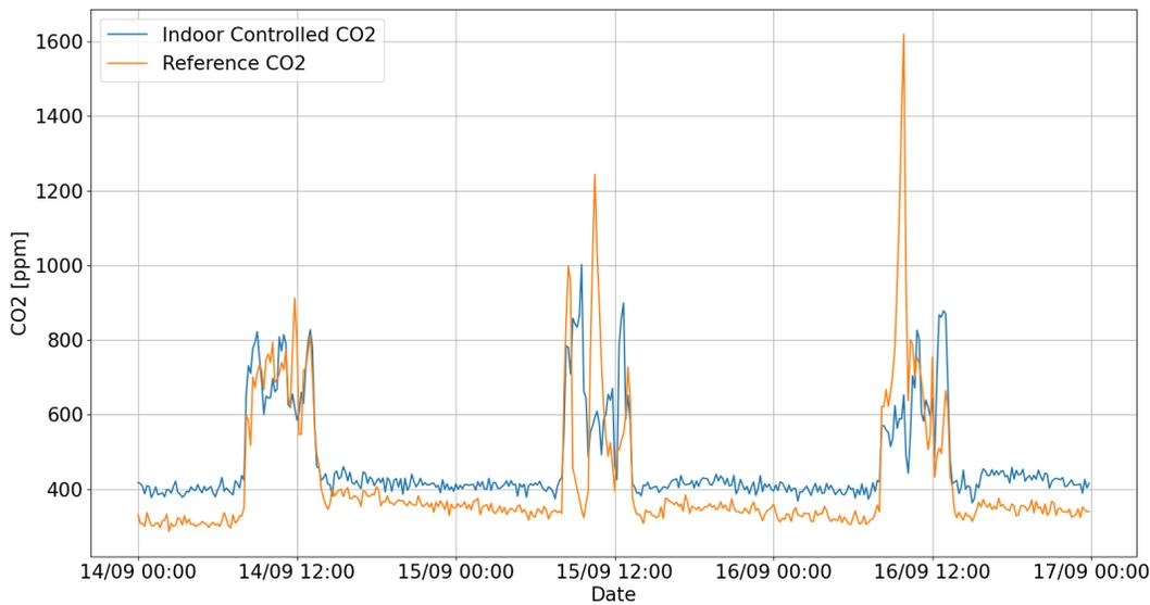
Figure 13.43: Controlled and reference carbon dioxide concentration in the room *act201bc* with the 600ppm single threshold approach
