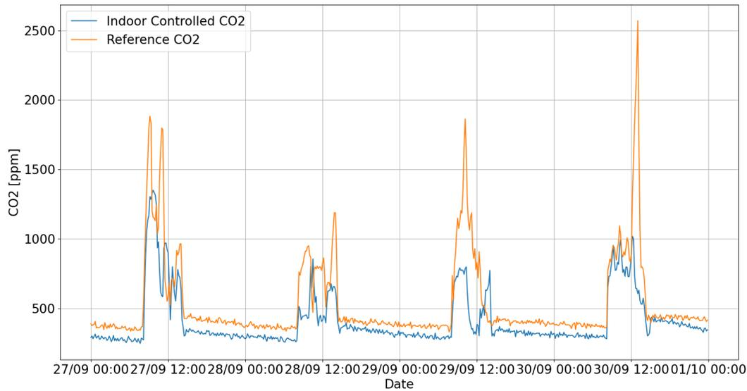
Figure 13.67: Controlled and reference carbon dioxide concentration in the room *act201cc* with the 1000ppm double threshold approach
