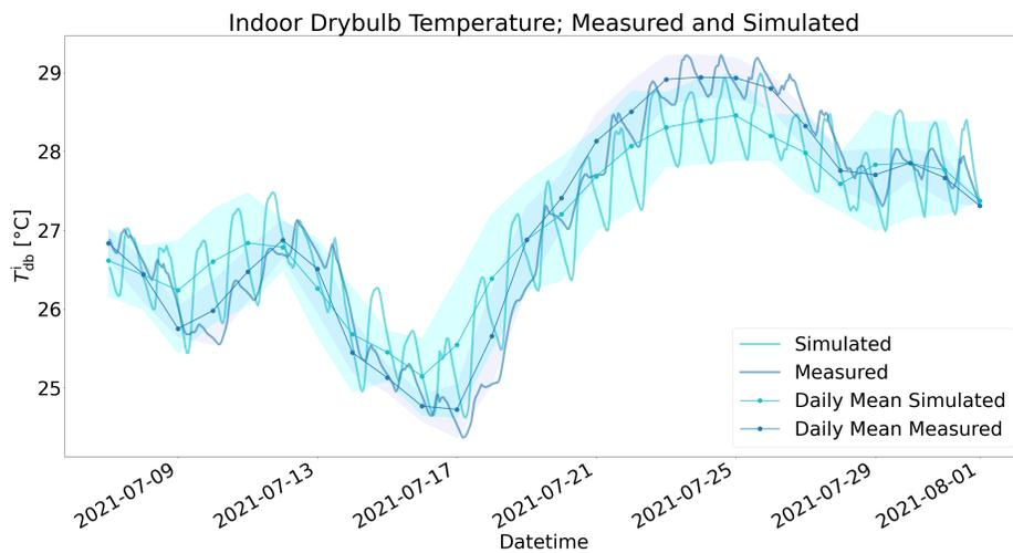
Figure 5.10: Simulated vs measured temperature behavior in the calibration period for the room *act208da*
