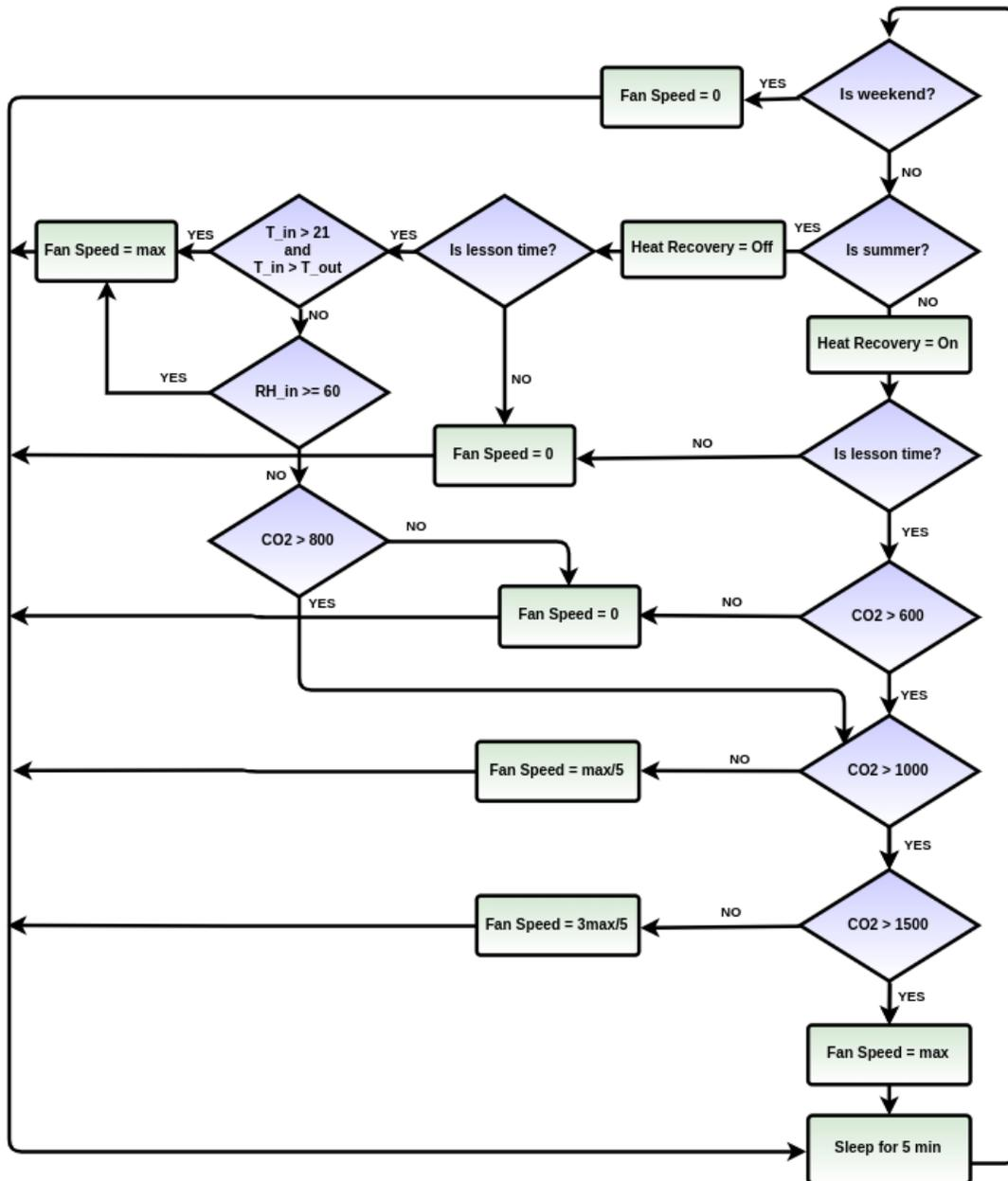
Figure 12.3: Temperature and humidity single thresholds for ventilative cooling and CO<sub>2</sub>-based control for correct IAQ during lessons time
