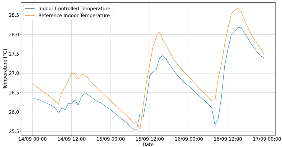
Figure 13.45: Temperature in the room *act201bc* and in the reference one with the  $600ppm$  single threshold approach
