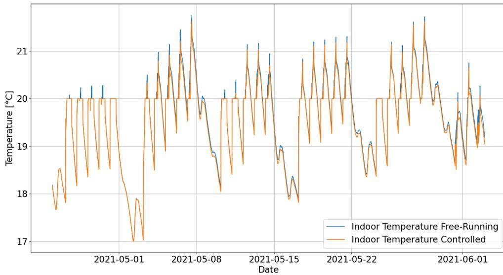
Figure 9.10: Indoor temperature behavior of the free-running building compared with the controlled one over the selected period
