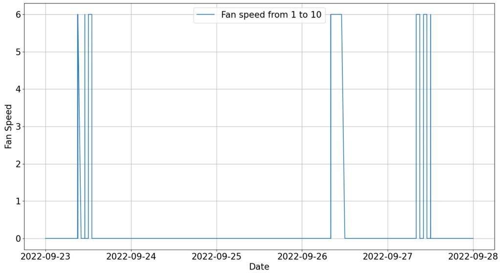
Figure 13.56: Ventilation rate of the mechanical ventilation system in the room *act201cc* with the 1000ppm single threshold approach
