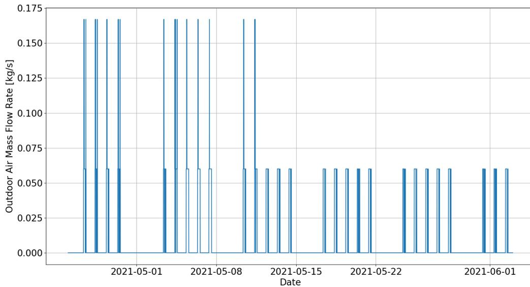
Figure 9.20: Ventilation airflow rate over the selected period
