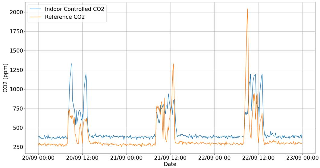
Figure 13.46: Controlled and reference carbon dioxide concentration in the room *act201bc* with the 600ppm double threshold approach
