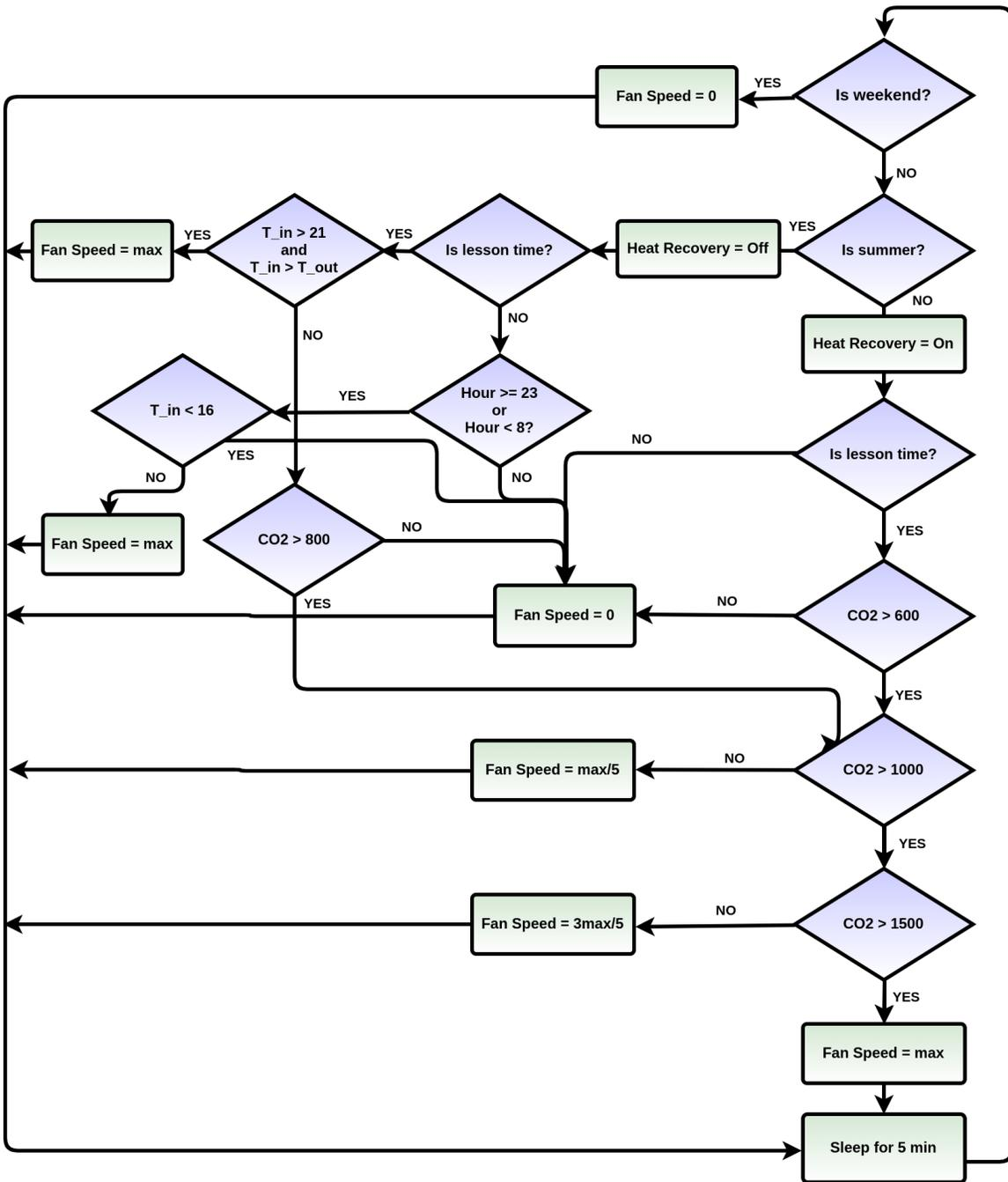
Figure 12.5: Night ventilation from 11:00 PM and temperature single threshold for ventilative cooling and CO<sub>2</sub>-based control for correct IAQ during lessons time
