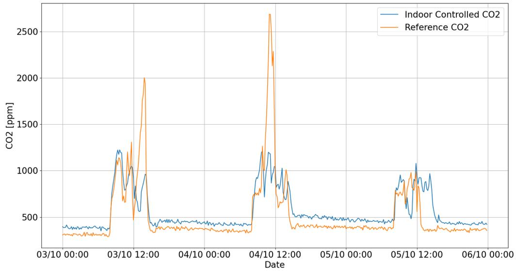
Figure 13.52: Controlled and reference carbon dioxide concentration in the room *act201bc* with the ASHRAE 62 approach
