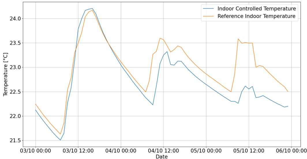
Figure 13.51: Temperature in the room *act201bc* and in the reference one with the 600ppm double threshold approach on the second floor
