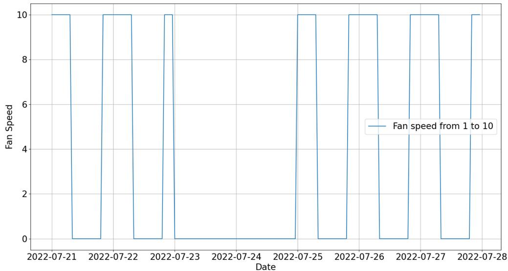
Figure 13.30: Ventilation rate of the mechanical ventilation system in the room *act208da* during the second week
