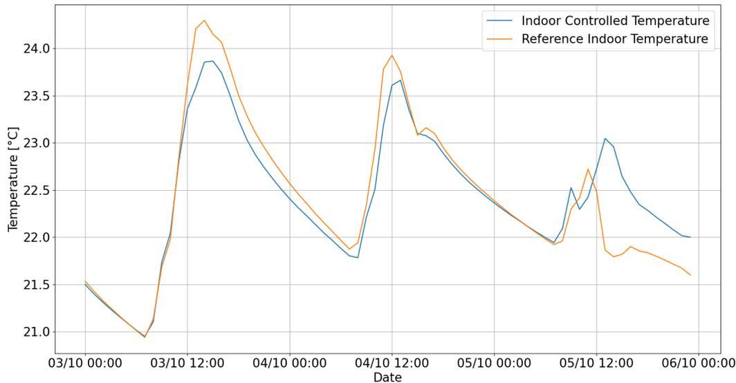
Figure 13.54: Temperature in the room *act201bc* and in the reference one with the ASHRAE 62 approach
