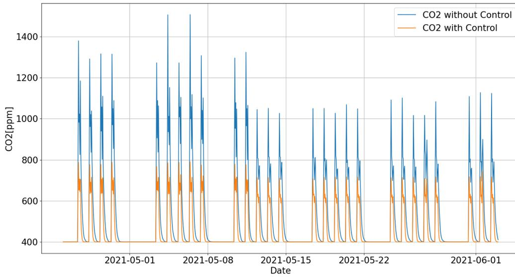
Figure 9.6: Indoor  $CO_2$  behavior of the free-running building compared with the controlled one over the selected period
