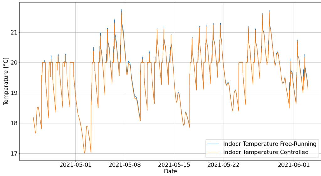
Figure 9.13: Indoor temperature behavior of the free-running building compared with the controlled one over the selected period
