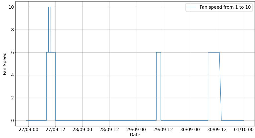
Figure 13.68: Ventilation rate of the mechanical ventilation system in the room *act201cc* with the 1000ppm double threshold approach
