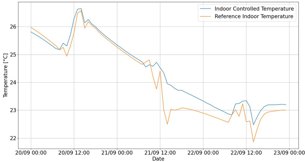
Figure 13.48: Temperature in the room *act201bc* and in the reference one with the 600ppm double threshold approach
