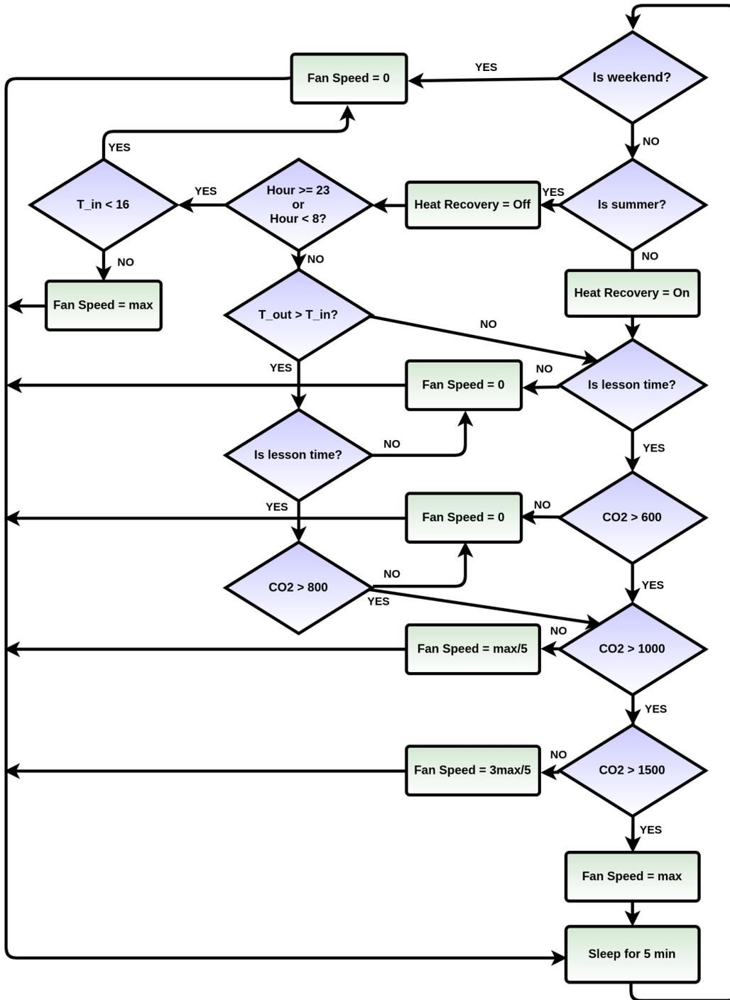
Figure 12.4: Night ventilation from 11:00 PM for ventilative cooling and CO<sub>2</sub>-based control for correct IAQ during lessons time
