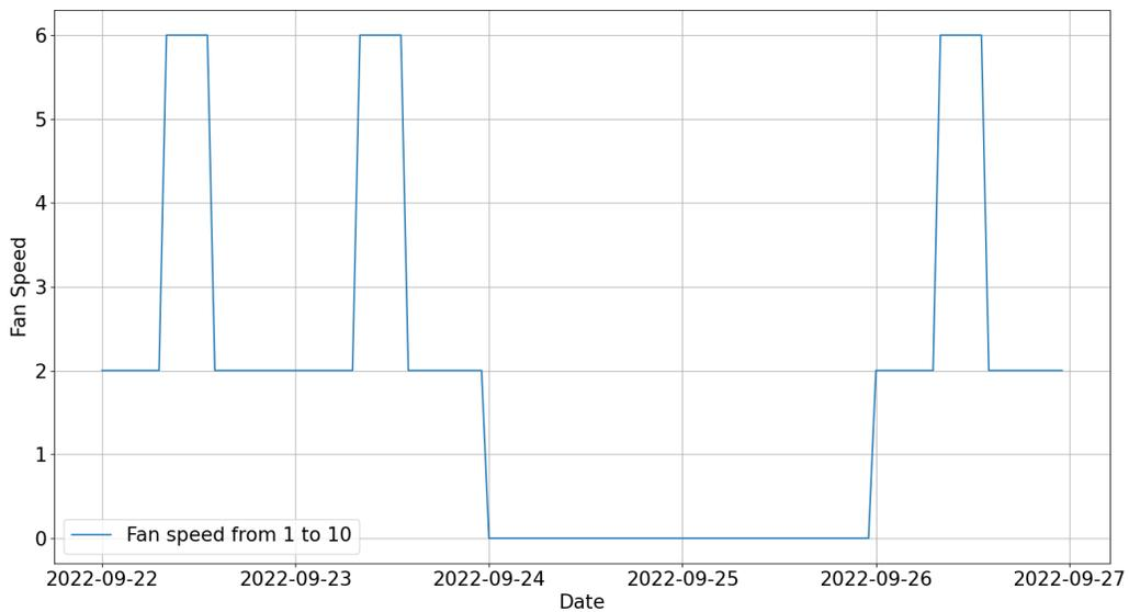
Figure 13.65: Ventilation rate of the mechanical ventilation system in the room *act201cc* with the ASHRAE 62.1 approach
