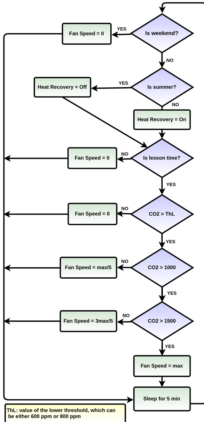
Figure 8.2: Ventilation algorithm based on a single  $CO_2$  threshold
