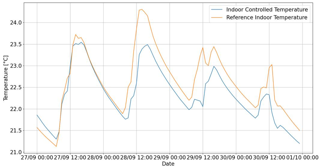
Figure 13.69: Temperature in the room *act201bc* and in the reference one with the 1000ppm double threshold approach
