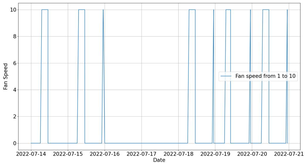
Figure 13.9: Ventilation rate of the mechanical ventilation system in the room *act201bc* during the first week
