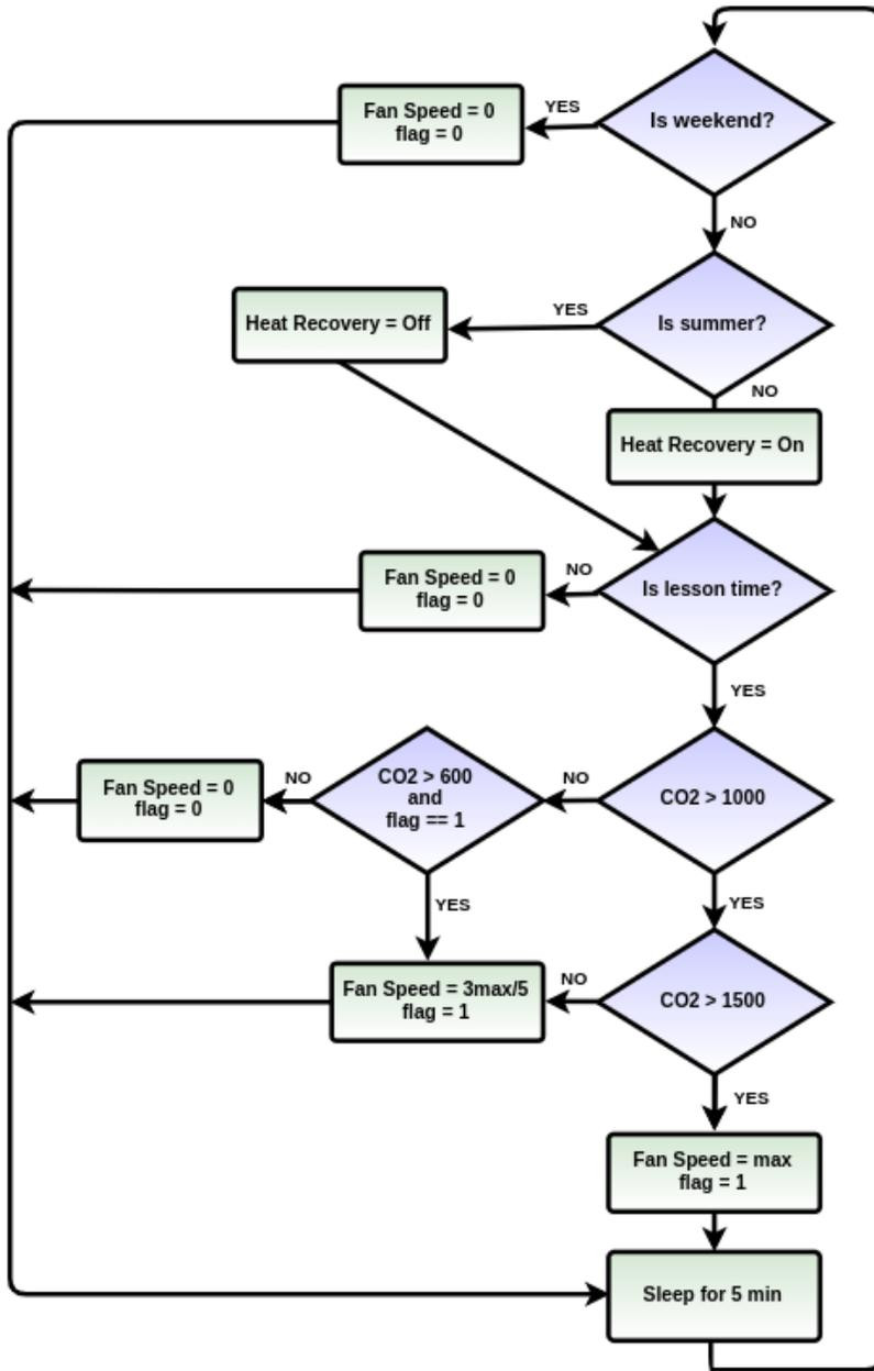
Figure 12.9:  $CO_2$  double threshold of  $600ppm$  and  $1000ppm$  approach
