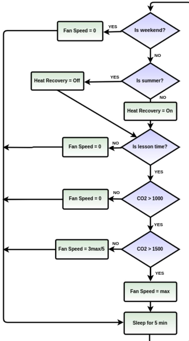
Figure 12.8:  $CO_2$  single threshold of  $1000ppm$  approach
