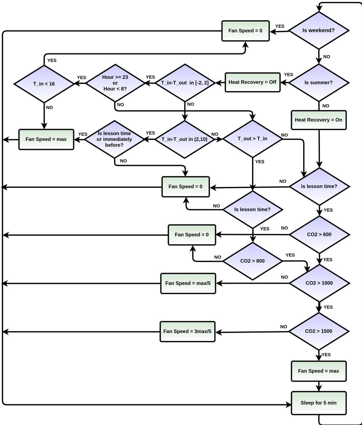
Figure 12.1: Internal and external temperature difference control for ventilative cooling and CO<sub>2</sub>-based control for correct IAQ during lessons time
