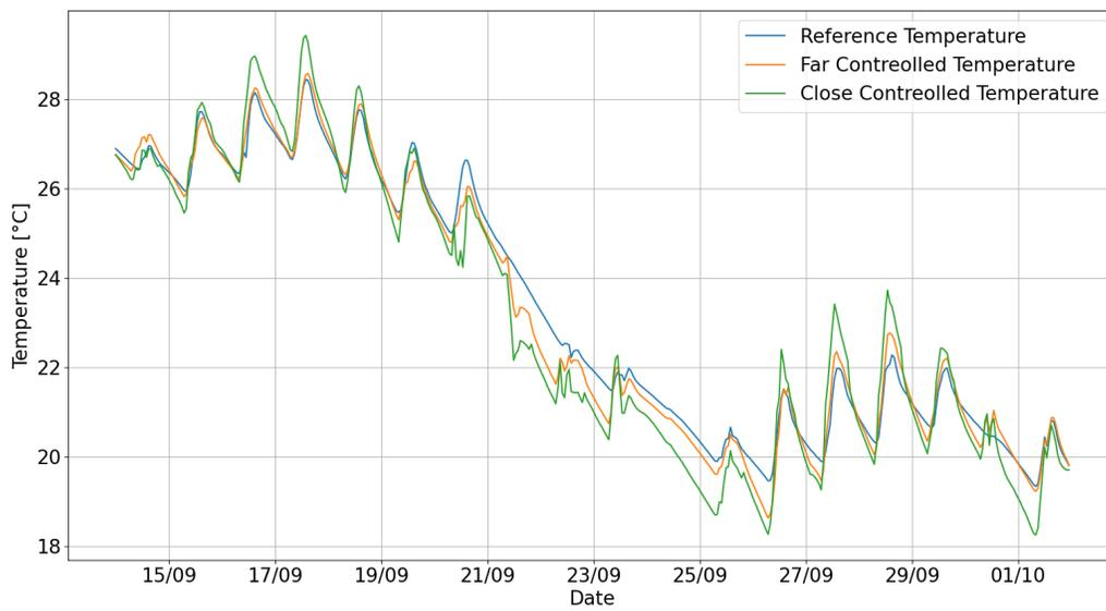
Figure 13.41: Sensor data of reference room and controlled one from far and near the mechanical ventilation unit
