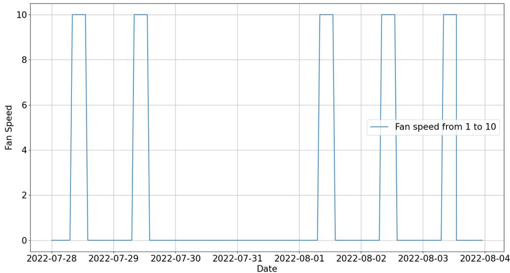
Figure 13.15: Ventilation rate of the mechanical ventilation system in the room *act201bc* during the third week
