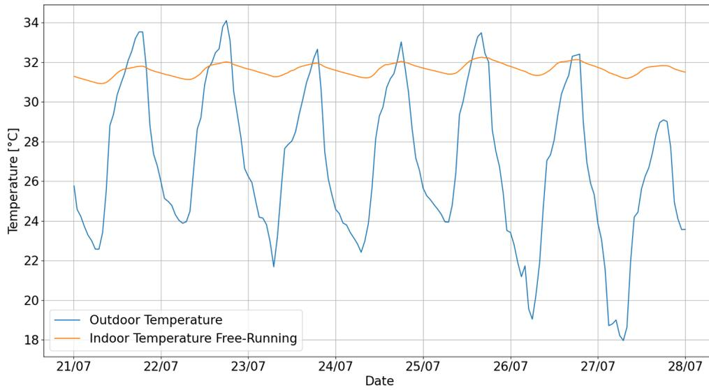
Figure 13.38: Outdoor and free-running indoor temperatures behaviors
