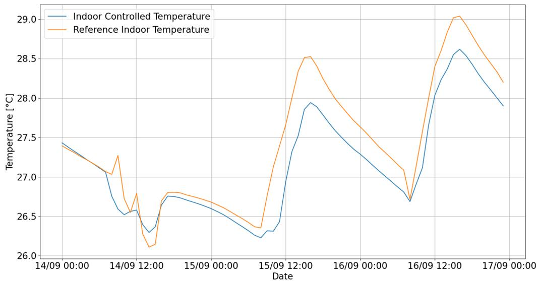
Figure 13.60: Temperature in the room *act201bc* and in the reference one with the  $800ppm$  single threshold approach
