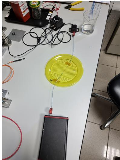
Figure 3.2: Set-up overview, wavelength interrogation.
