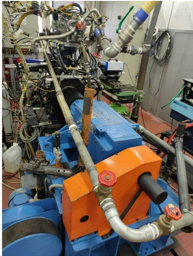
Figure 2.7 Test rig setup (top), Electric machine coupled with the engine (49.7 kW power, 230 Nm maximum torque)(bottom) from [6]
