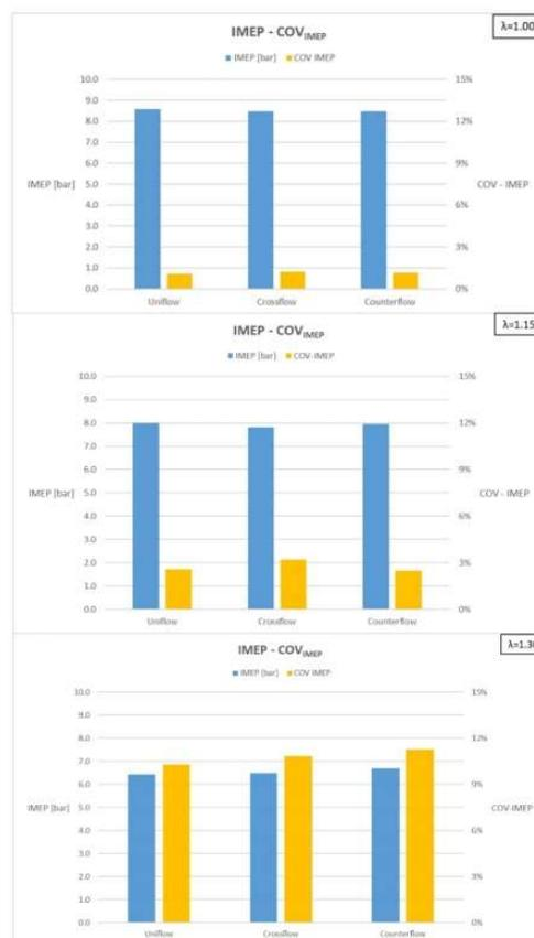
Figure 1.7 IMEP and  $COV_{IMEP}$  for different air-fuel ratio from [6].
